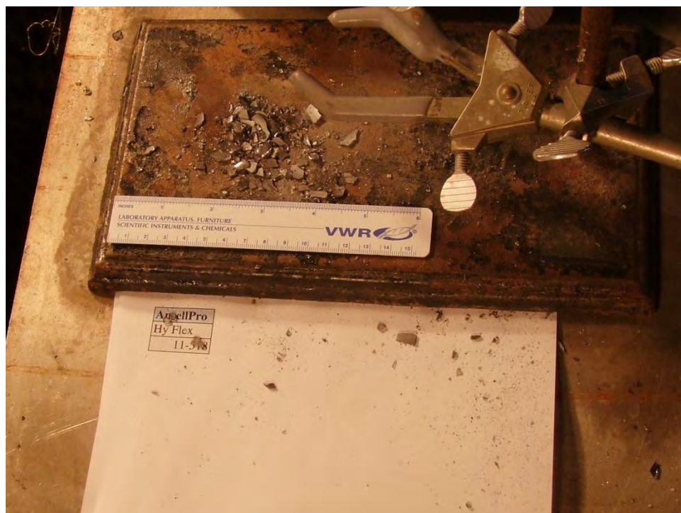
Figure A-6 Representative of glass particulate size from detonation of 20 mL vial
