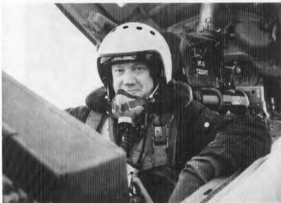
Fig. 16—Author after Strapping In. Holes in Helmet Help Ensure Helmet Retention During High-Speed Ejection
