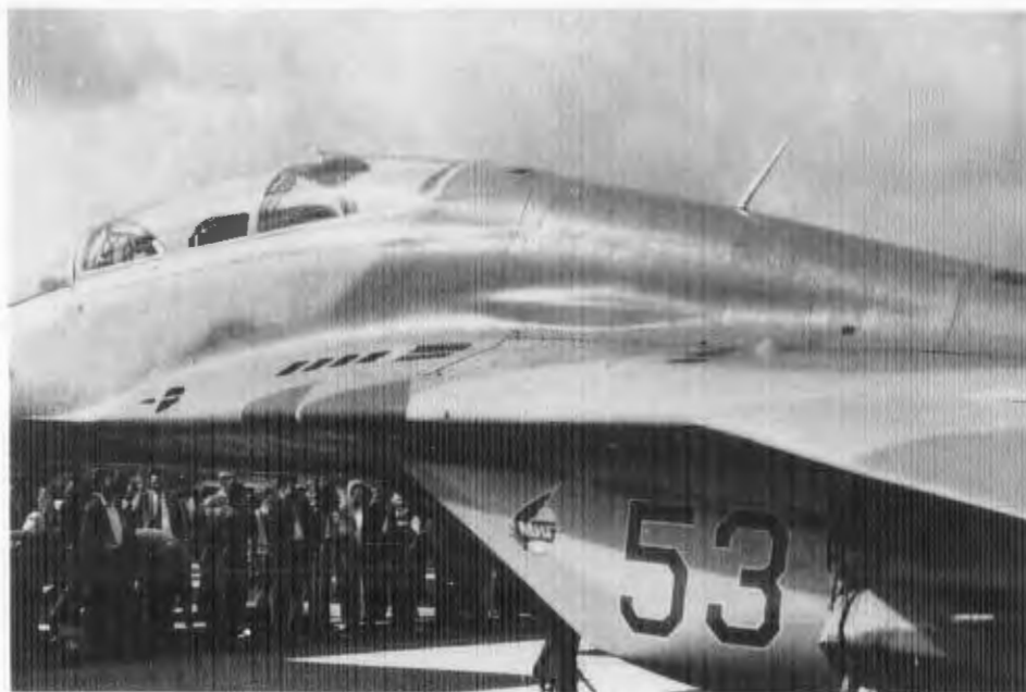
Fig. 32—MiG-29UB at Farnborough Showing Fuselage Bulge and Rough Finish of Aerodynamic Surfaces
