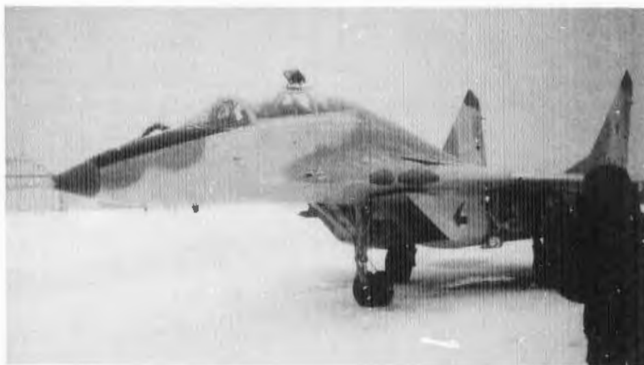
Fig. 1—MiG-29UB Before Taxi with Aft-Cockpit Periscope Extended. Note Right-hand Inlet Door Closed, Indicating Right Engine Running. Note Also Melted Snow Beneath Fuselage Caused by Engine Bleed-Air Exhaust
