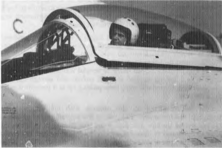
Fig. 26—Anatoly Kvochur at Farnborough with MiG-29 Canopy in Cracked Position, Showing High Canopy Rails and Restricted Field of View
