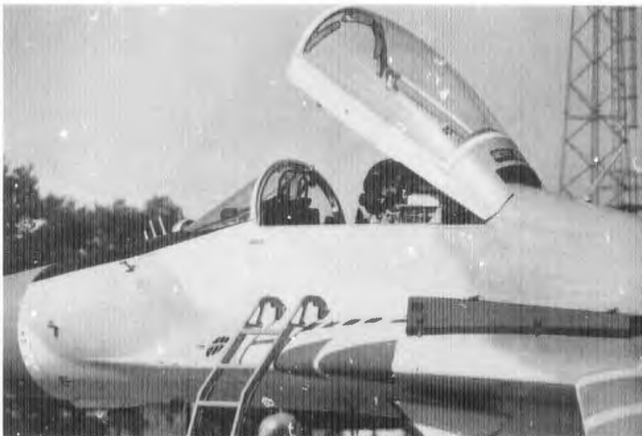
Fig. 25—MiG-29 Cockpit and Canopy Arrangement
