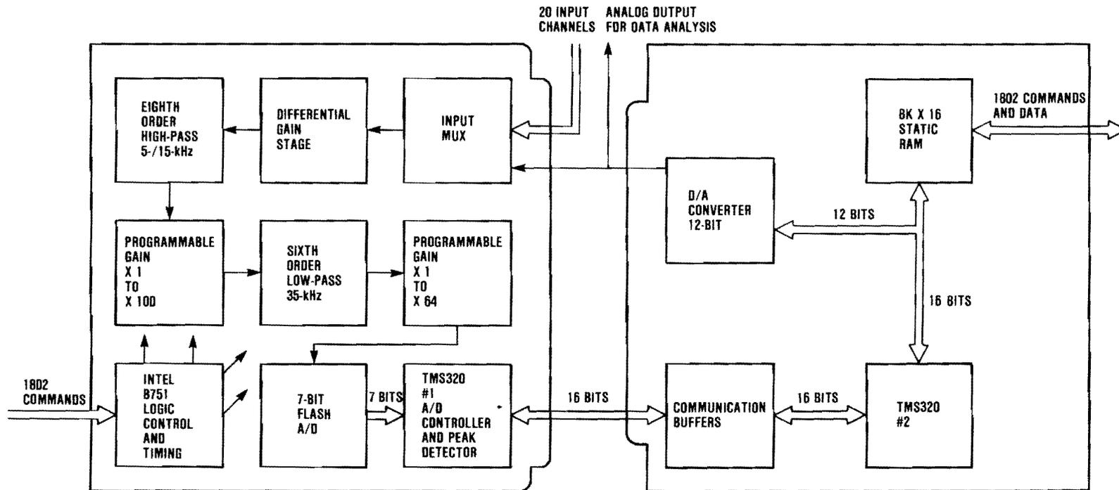
Figure D-2. SPADE Analyzer Signal Processing Block Diagram
