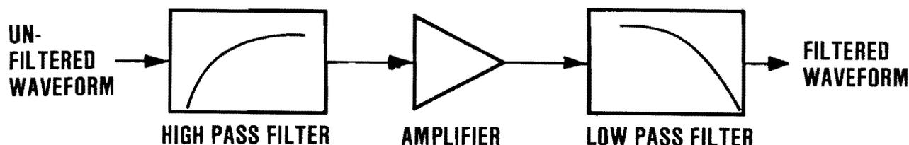
Figure 49. Filter System Block Diagram
