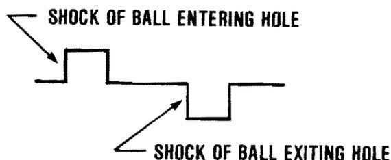
As can be seen, the model deviates from the original model in that two shock pulses, not one, are generated. The first shock pulse originates from the ball entering the fault while the second shock pulse originates from the ball exiting the fault. The detection scheme is based upon an understanding of the physical phenomena of these events, and a signal processing design capable of discriminating the resultant signal characteristics.
