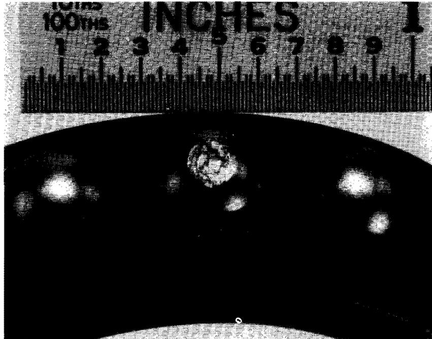
Figure C-21. 90-Degree Gearbox -424 Bearing Ball Fault C/D,
