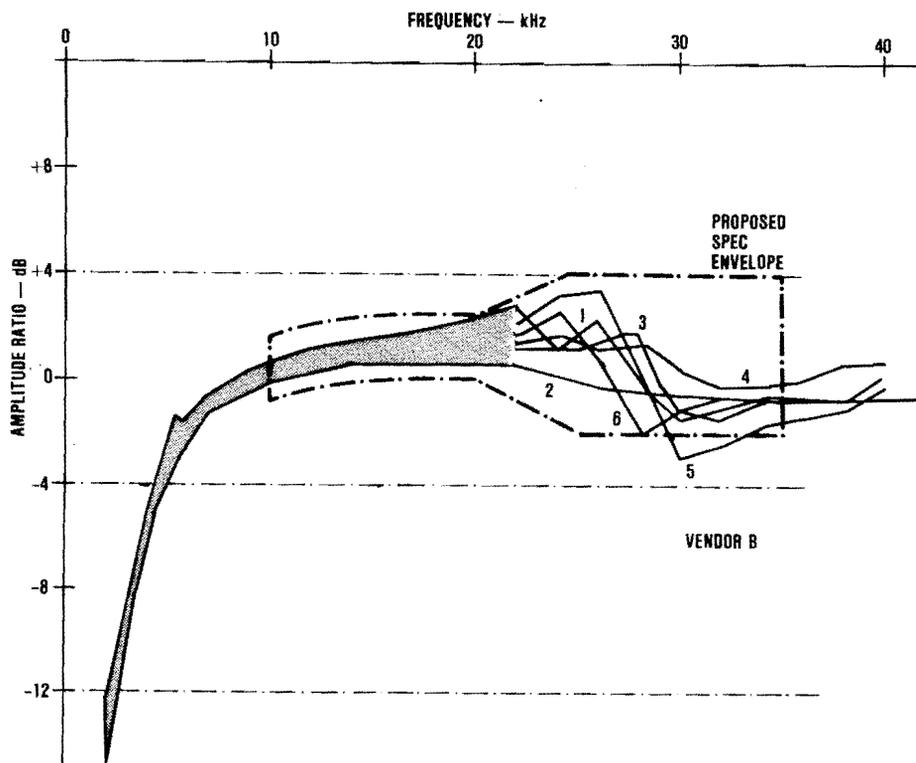
Figure 53. Frequency Response of Six Vendor B Sensors
