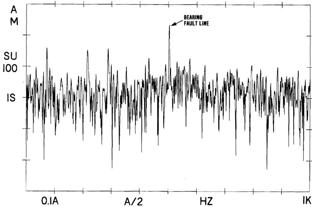
Figure 115. Bearing Fault Signature Resulting From Single FFT
