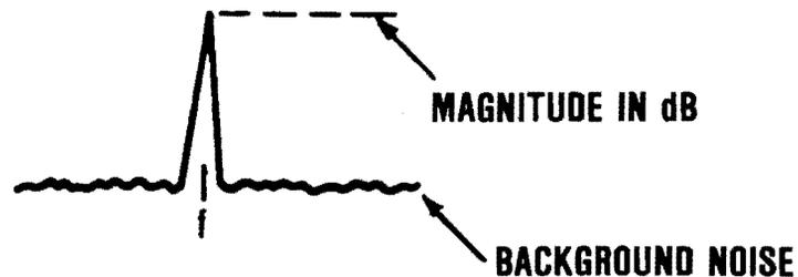
As a fault progresses in severity, the structure of lines in the FFT will change both in width and in amplitude. Figure 117 shows the change in the spectrum from a fault which progressed from the C/D level to the extremely gross category. The identification and classification process is designed to accommodate this possible change in line structure.
