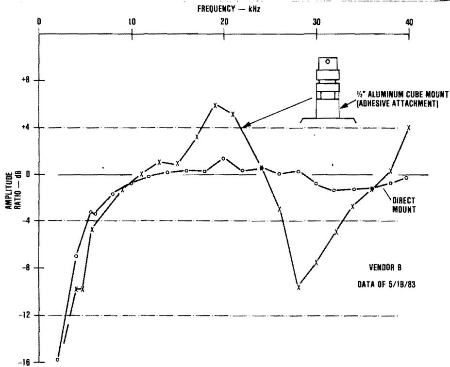
Figure 56. SPADE Sensor Mount Effect
