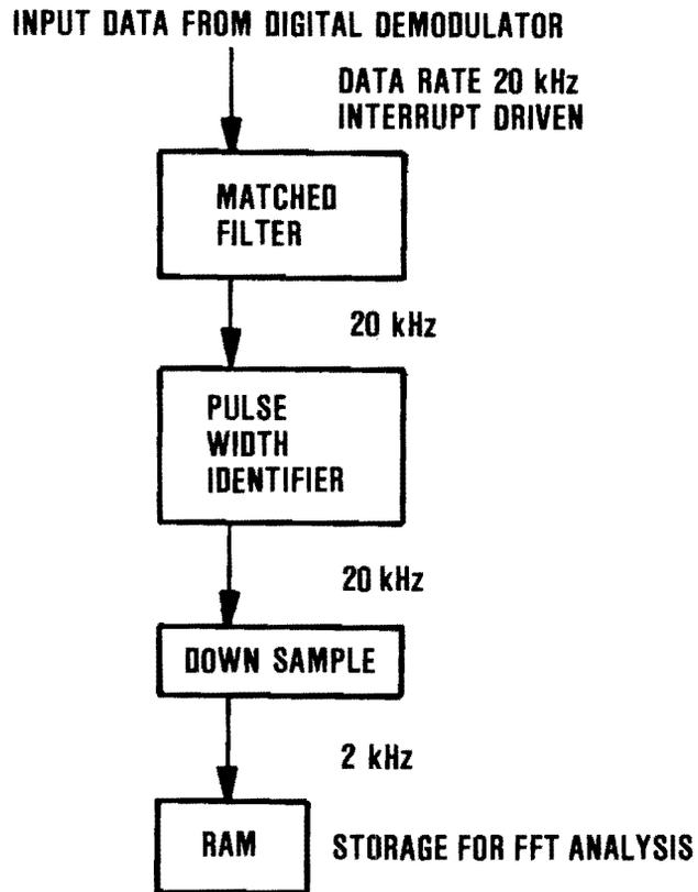
The pulse processing module is interrupt driven and accepts data at a 20 kHz rate from the digital demodulator. The input data stream from the digital demodulator is shown in Figure 110. The data is first passed through a matched filter to extract signals with bearing signature features. The output of the matched filter, shown in Figure 111, demonstrates that the matched filter is quite effective in extracting possible bearing signatures from other signal elements.
