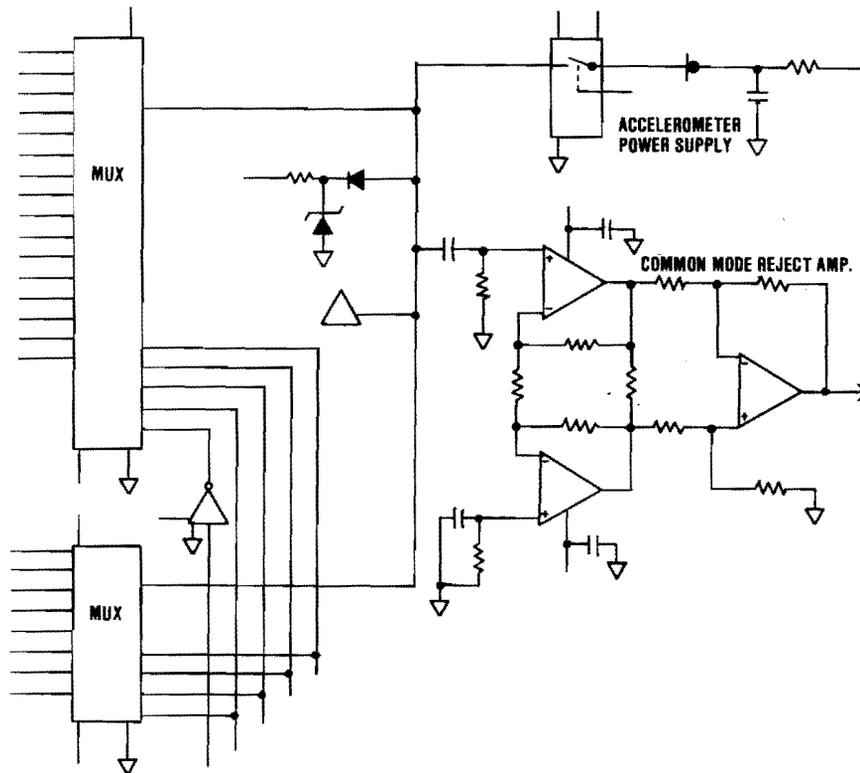
Figure 101. SPADE Analyzer Electrical Front End
