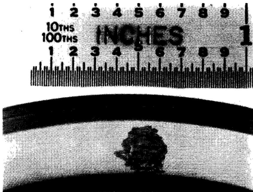
Figure C-22. 90-Degree Gearbox -407 Bearing Outer Race C/D,
