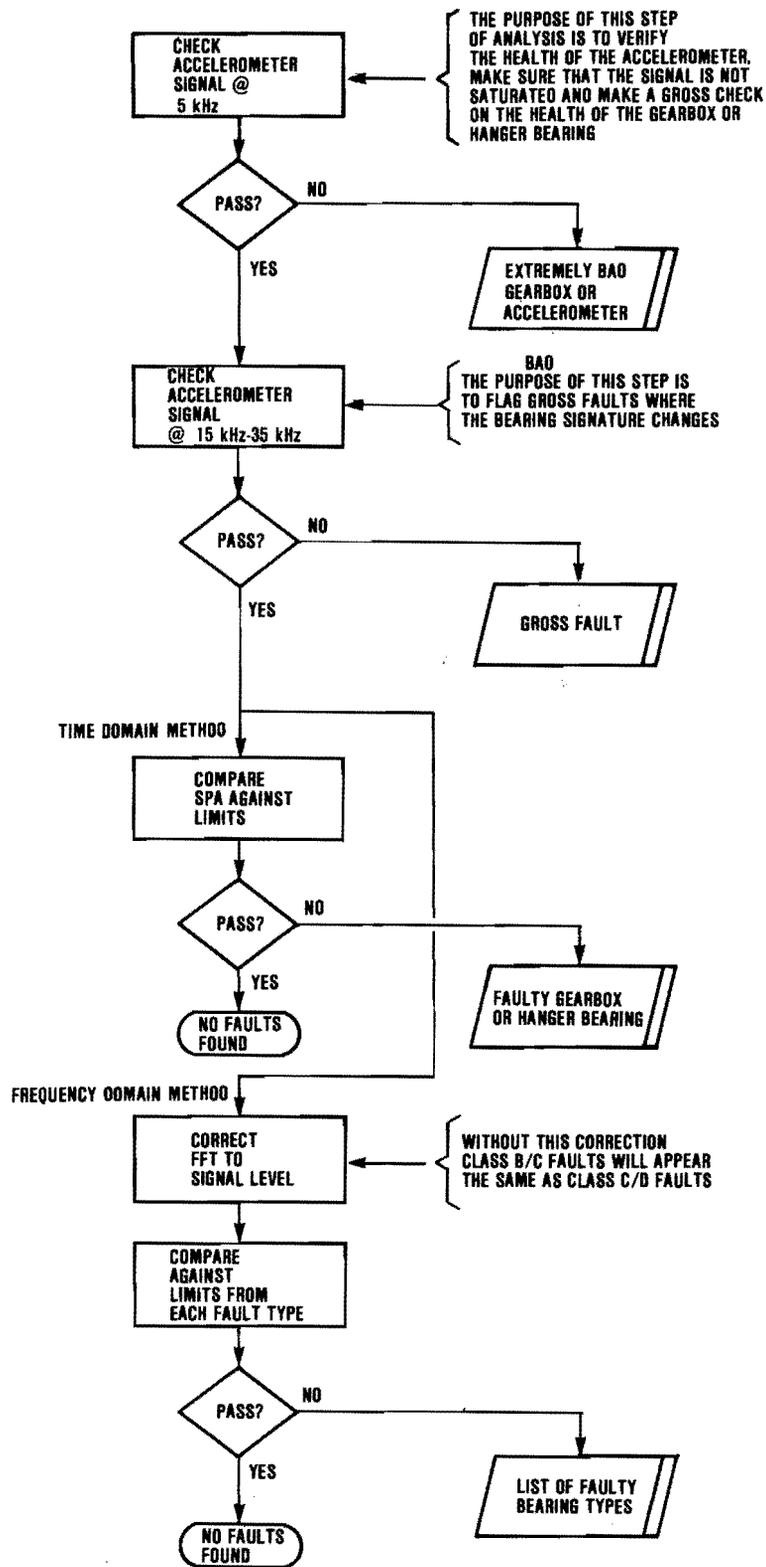
Figure 98. Processing Required to Determine Bearing Assembly Faults
