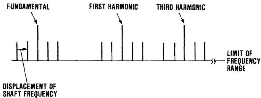
From the list of spectral peaks identified in the previous module, an attempt is made to match the spectral lines with the pattern presented above. The following rules are employed in analyzing spectral peaks:
