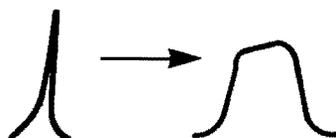
Although the amplitude of the signal decreases, the power in the peak increases due to the increased area of the peak. Therefore, another quantity must be defined in order to account for this effect. This quantity is the area under the peak and is defined by the shaded area shown in the illustration below.
