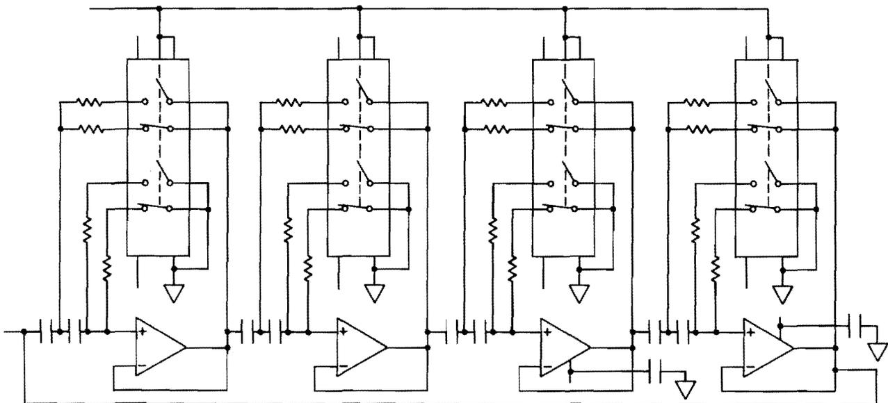
Figure 45. 5/15 kHz Butterworth High-Pass Filter Design
