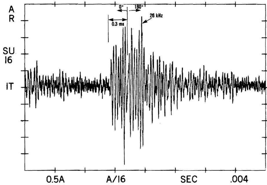
Figure 9. Details of Outer Race Fault Signal
