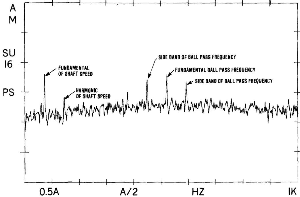
Figure 88. Inner Race Fault/Digitally Processed
