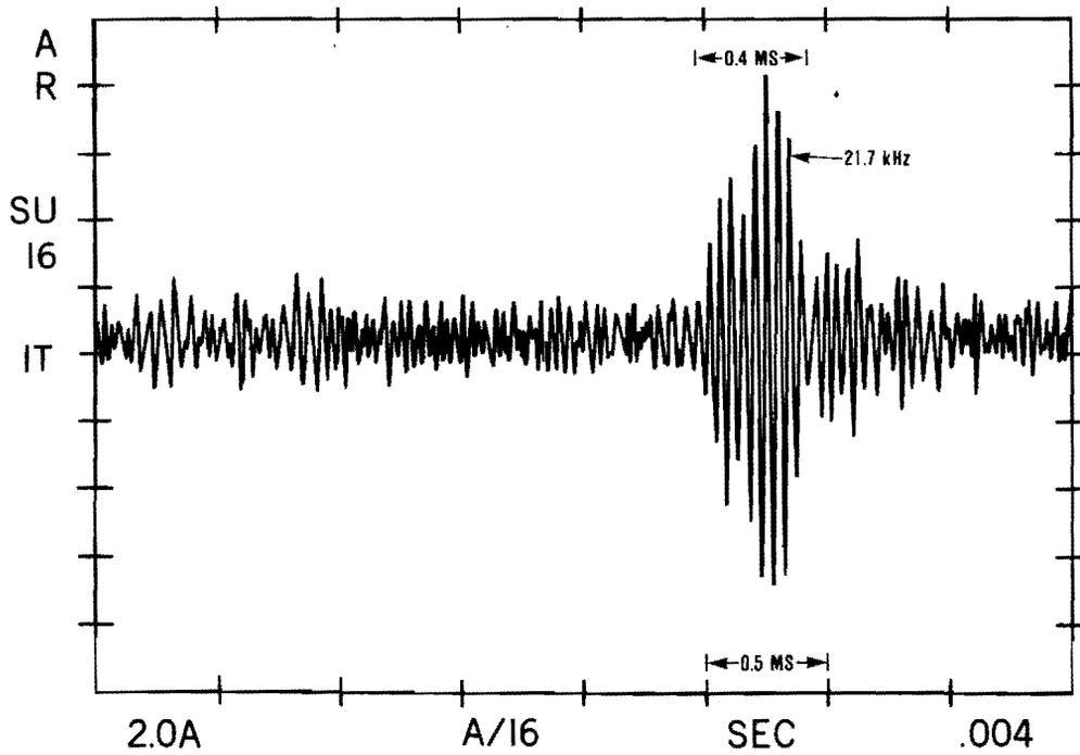
Figure 10. Details of Inner Race Fault Signal
