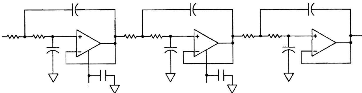
Figure 48. 35 kHz Butterworth Low-Pass Filter Design
