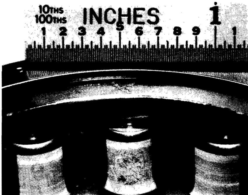
Figure C-15. 42-Degree Gearbox -310 Bearing Roller Fault C/D,
