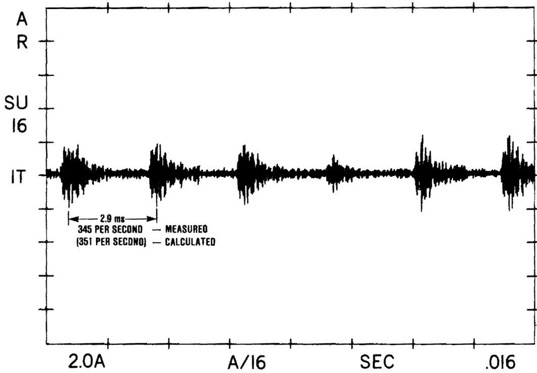
Figure 3. Band-Pass Filtering Reveals Bearing Fault Signal
