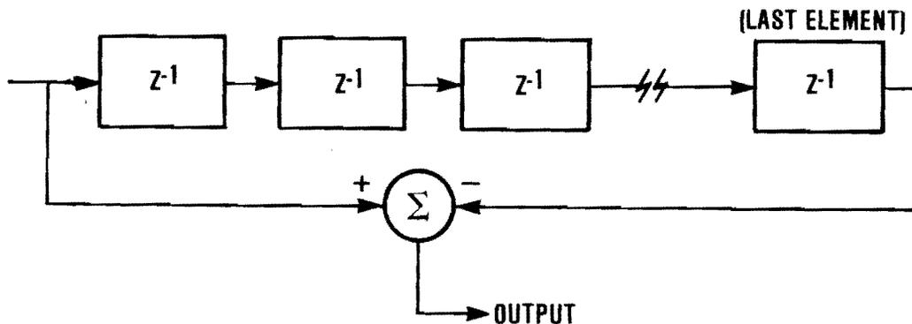
In this implementation of the matched filter, the initial state is important and hence the filter's delay elements must be initialized to zero before execution.
