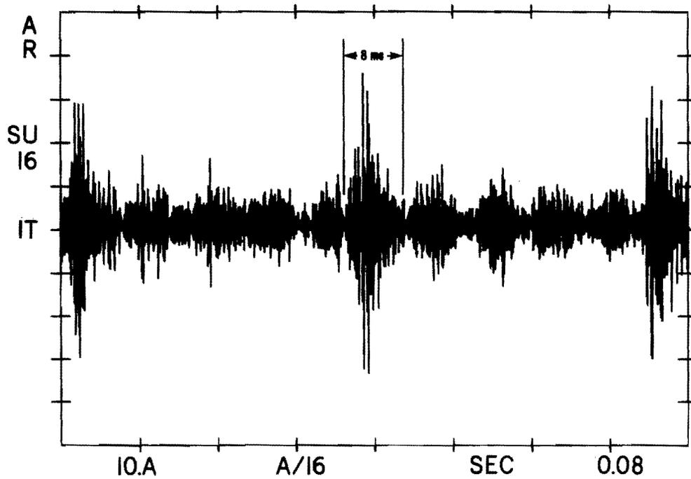
Figure 15. Machinery Imbalance Clutter Waveform (5 kHz High-Pass Filtered)
