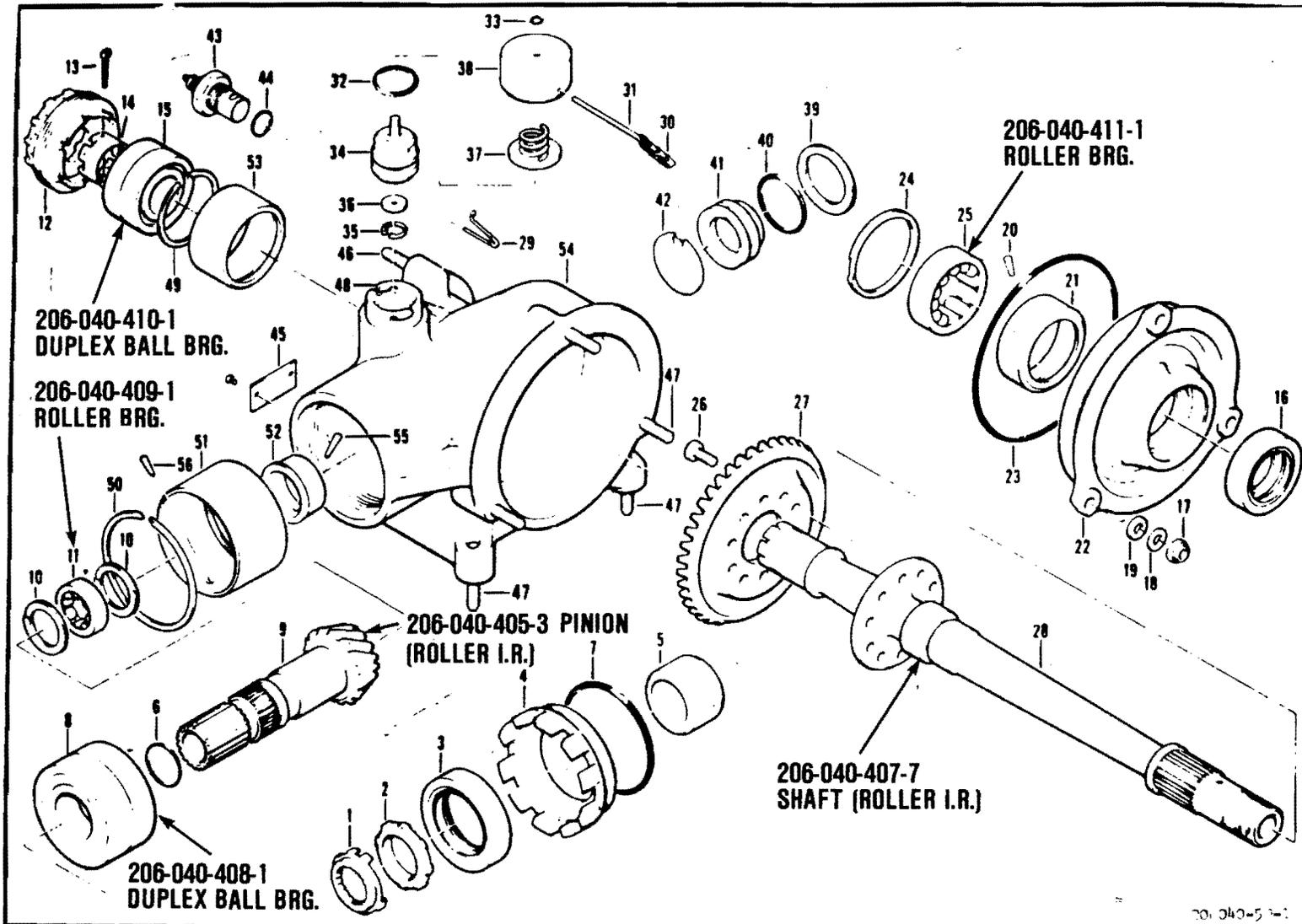
Figure C-45. Tail Rotor Gearbox, OH-58 A/C
