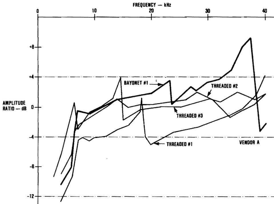
Figure 51. Frequency Response of Four Vendor A Sensors
