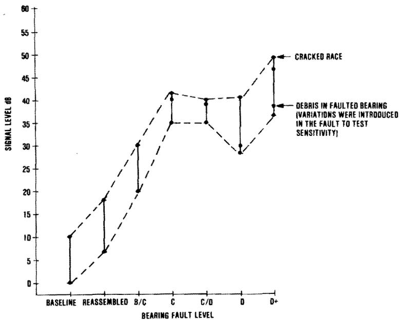
Figure 44. Typical SPADE Processing Signal Level as a Function of Bearing Fault Level
