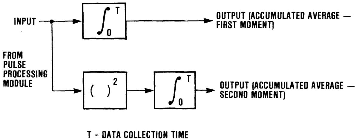
The processing consists of two paths. The first path simply accumulates the sum of the output of the pulse processing module, and the second path squares the output of the pulse processing module and accumulates the sum. It was anticipated that a statistical relation between these summations could be obtained for fault detection. However, as shown in Section 8, the time domain method performed very poorly.
