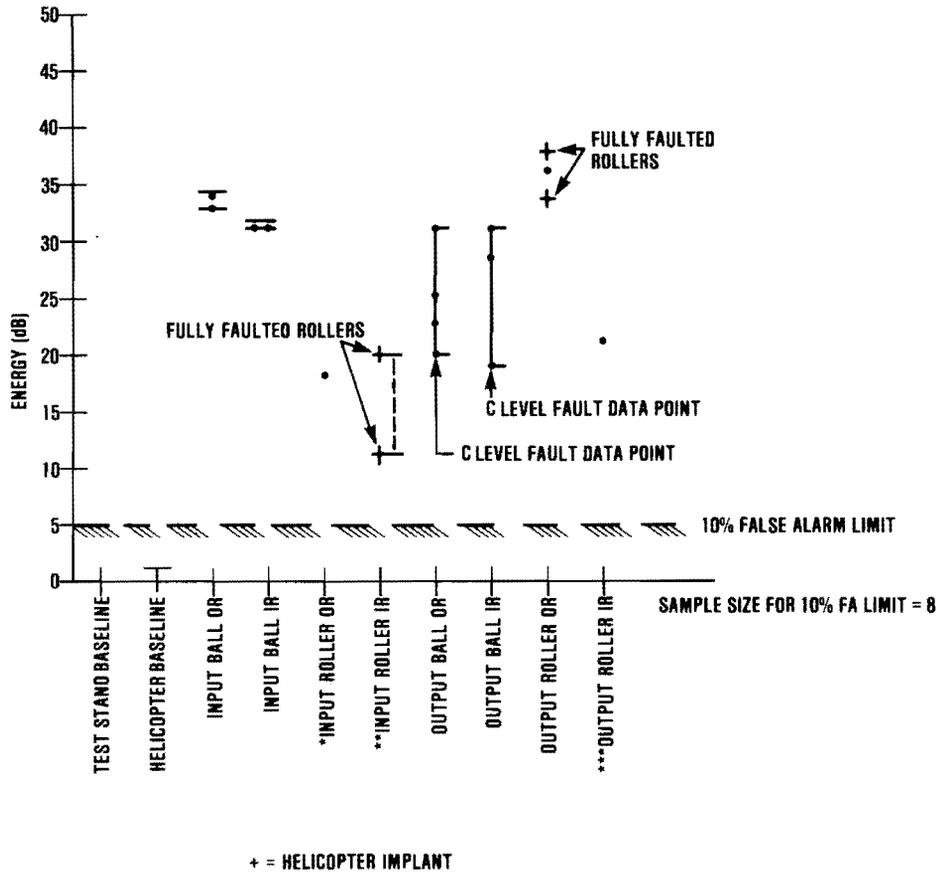
Figure 123. Frequency Domain Performance, 90-Degree Gearbox Data for UH-1 and AH-1 Aircraft
