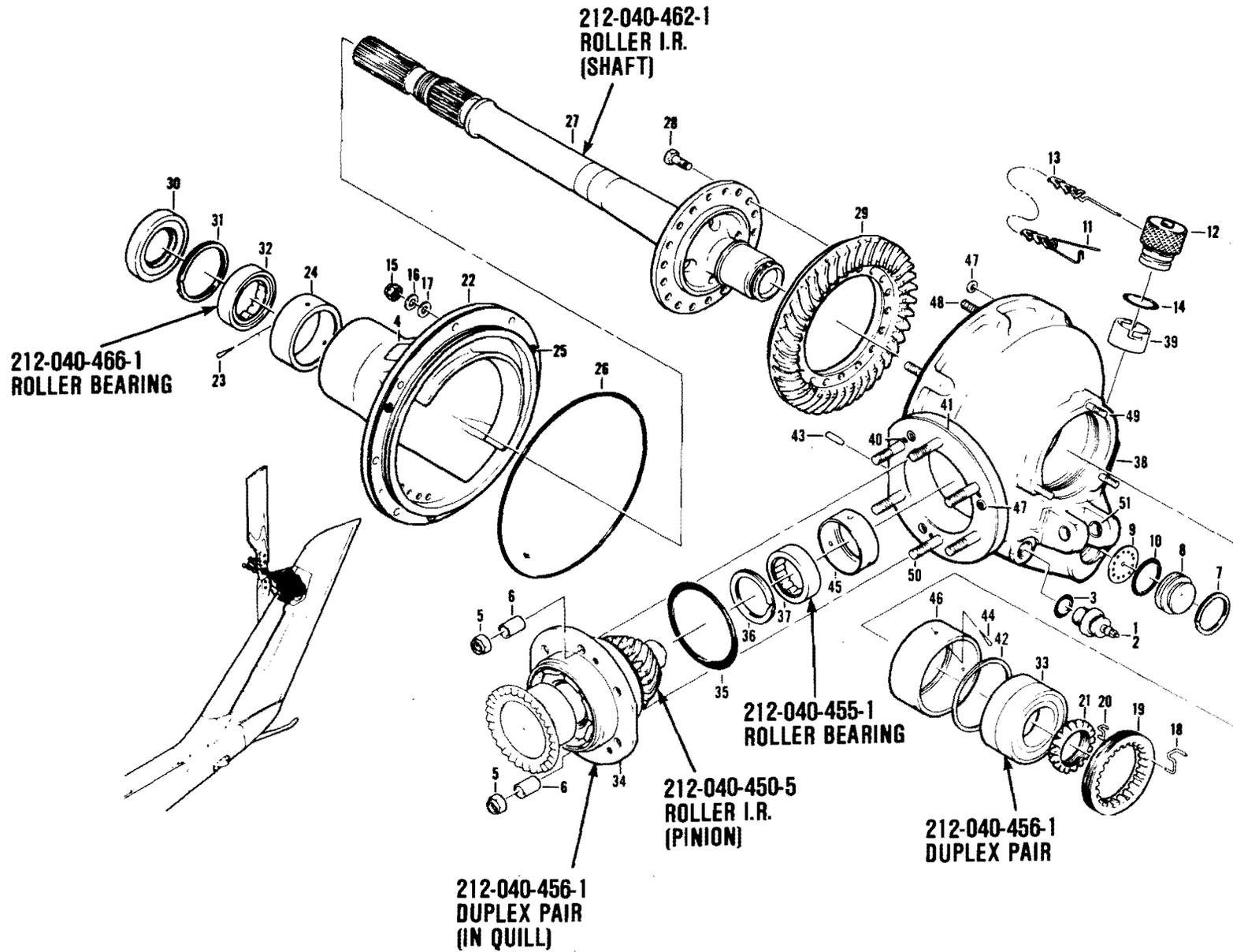
Figure C-9. Gearbox Assembly, 90-Degree Tail Rotor Drive, AH-1S
