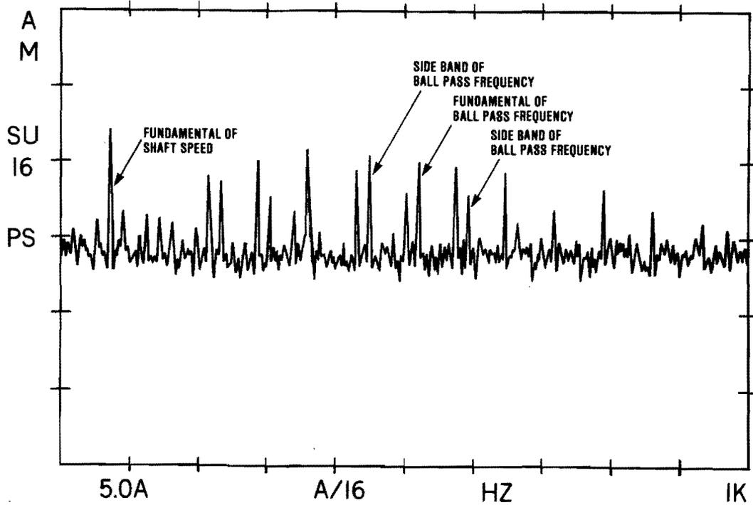
Figure 112. Unprocessed Spectrum
