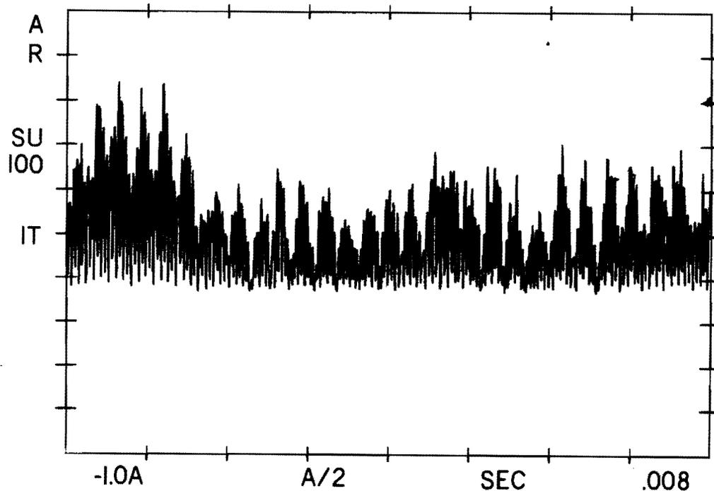
Figure 80. Demodulated Band-Passed Signal of a Ring Gear Fault
