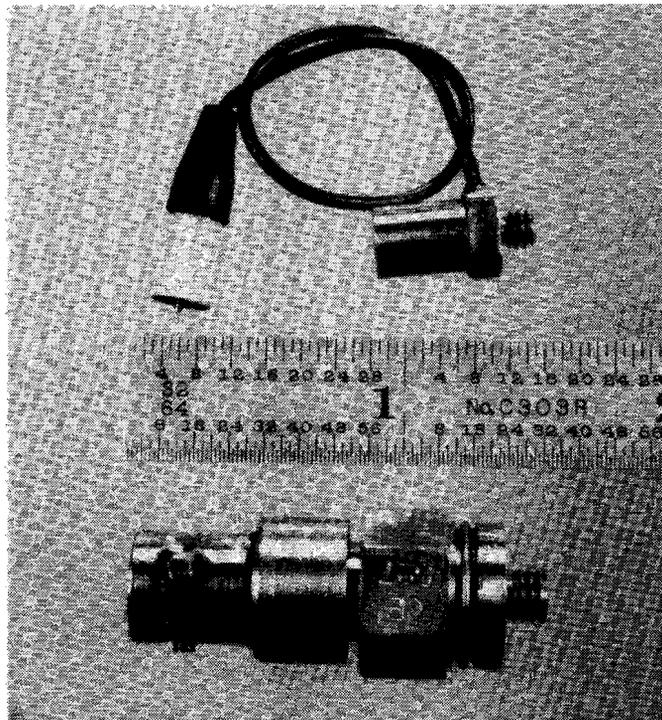
Figure 52. Vendor B's SPADE Sensor and Miniature Accelerometer
