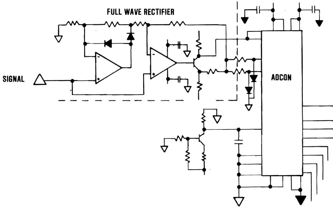
Figure 105. Full Wave Rectifier and A/D Converter
