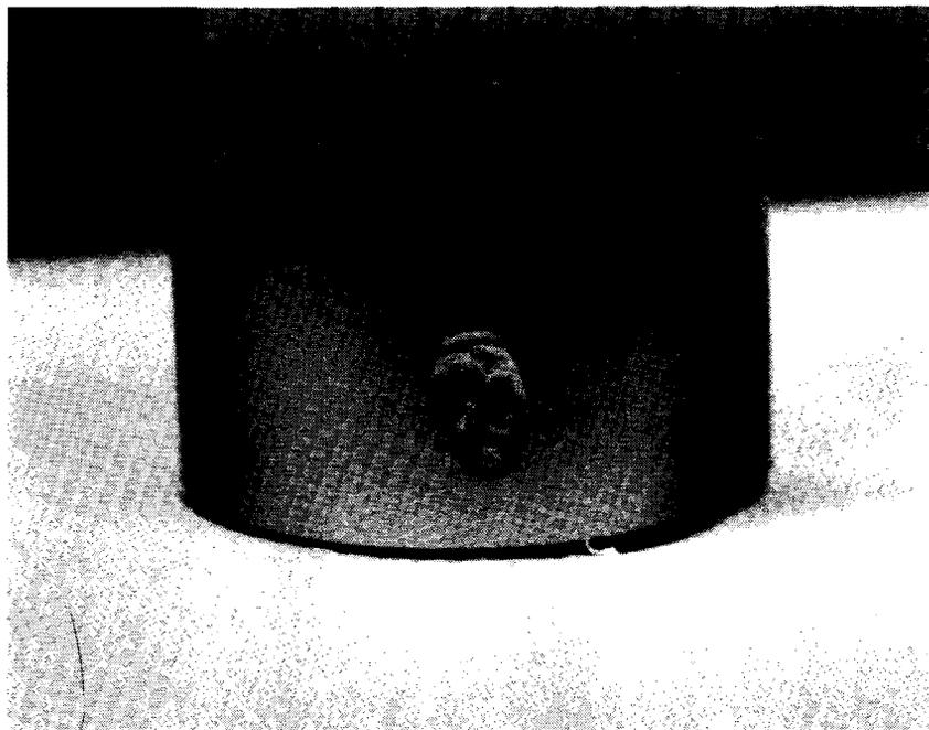
Figure C-32. 90-Degree Gearbox -462 Shaft (Inner Roller BRG Race
