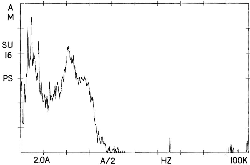
Figure 100. Power Spectrum of Raw Accelerometer Signal
