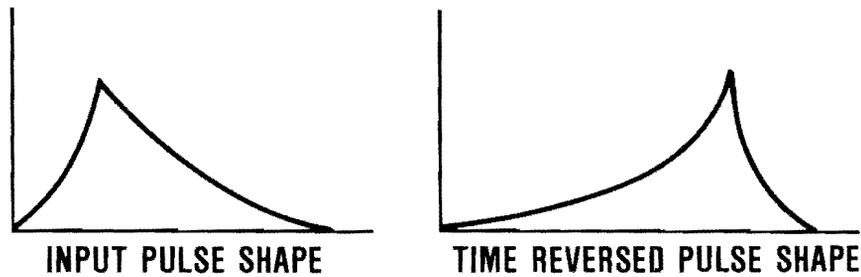
Figure 73. Impulse Response of a Matched Filter
