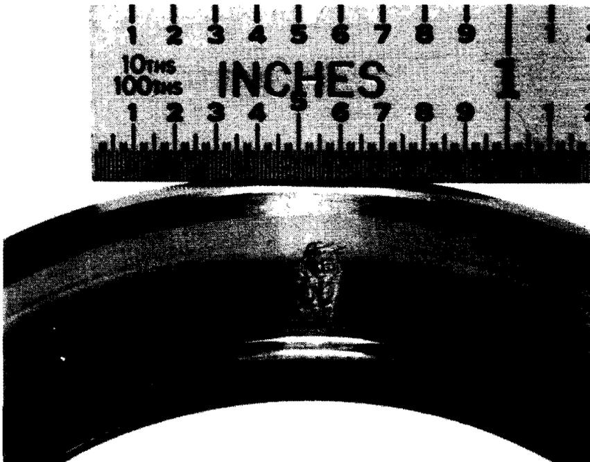
Figure C-16. 90-Degree Gearbox -406 Bearing Outer Race C/D,
