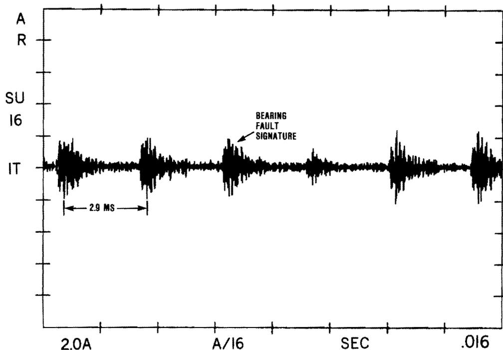
Figure 13. Band-Pass Filtered Signal
