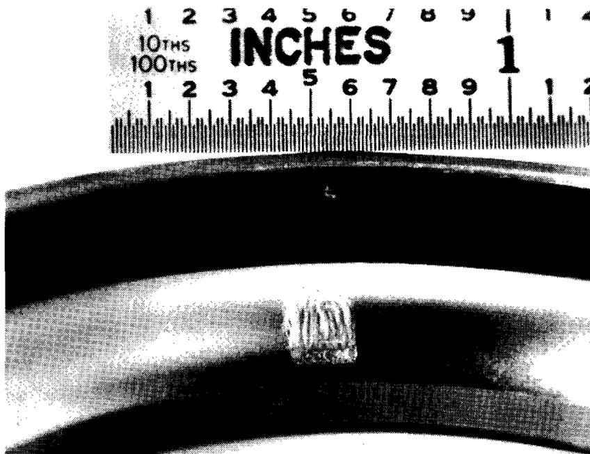
Figure C-34. 42-Degree Gearbox -143 Bearing Outer Race C/D,
