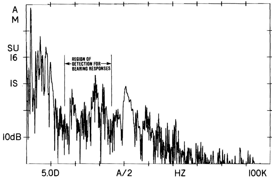
Figure 11. Frequency Response of a Resonance Accelerometer
