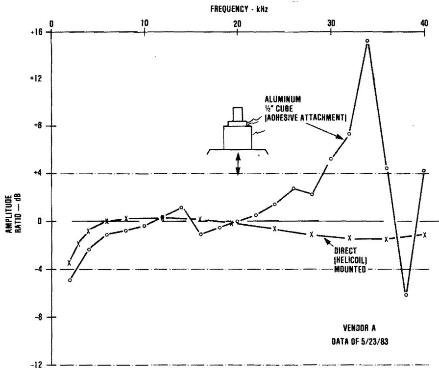
Figure 55. Effect of Simple Cube Mount on Accelerometer Response
