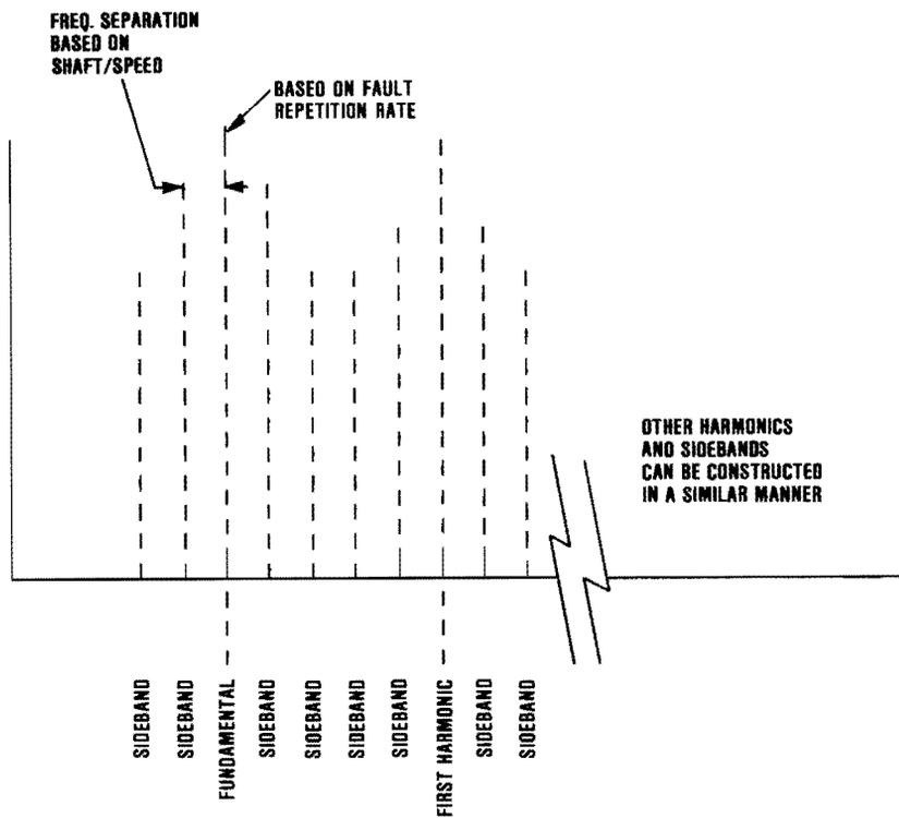
Figure 128. Typical Frequency Template for Bearing Faults
