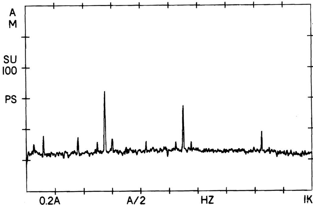
Figure 38. Frequency Domain Spectra of a Bearing Fault
