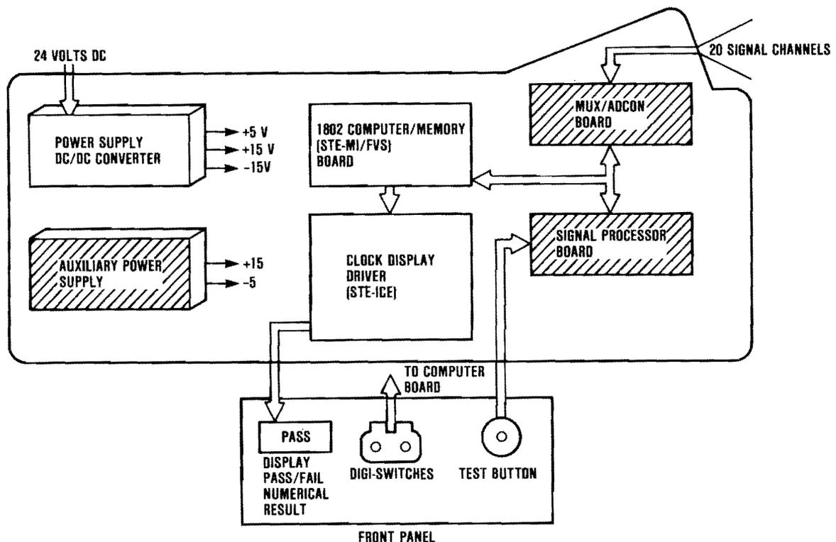
Figure D-1. SPADE Analyzer Electrical Block Diagram
