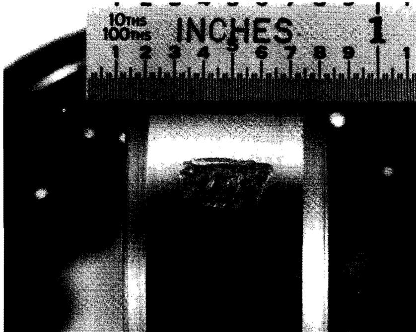
Figure C-13. 42-Degree Gearbox -310 Bearing Inner Race C/D,
