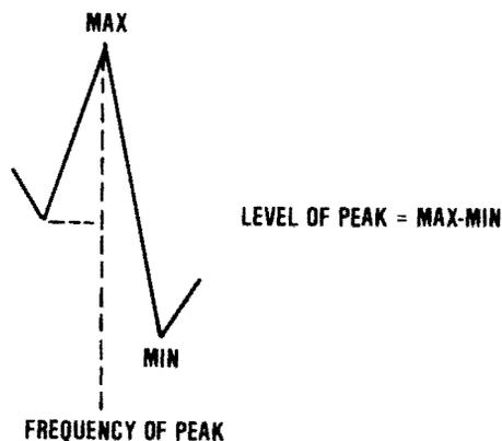
At this stage of the processing, no decision is made on whether a spectral peak is a bearing fault signal or not.
