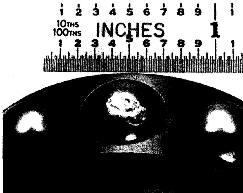
Figure C-14. 90-Degree Gearbox -143 Bearing Ball Fault C/D,
