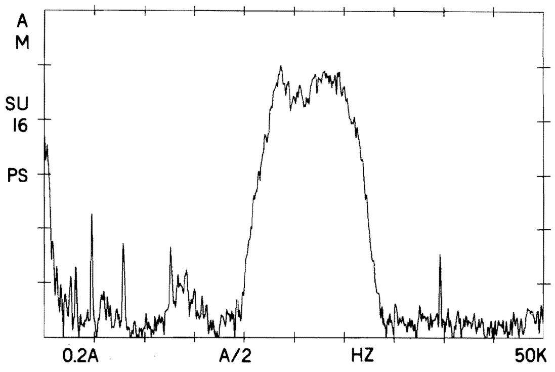
Figure 35. Power Spectrum After Application of Band-Pass Filter
