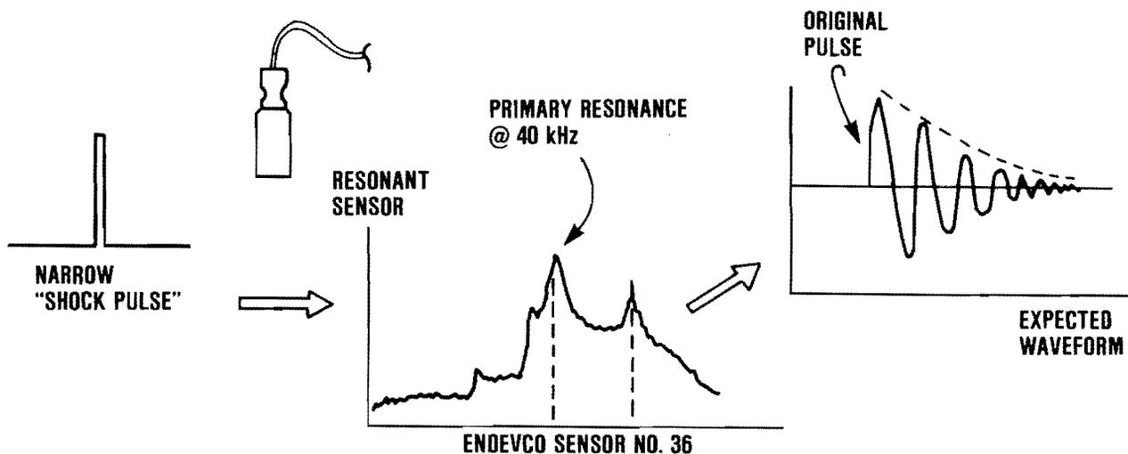
Figure 20. Shock Pulse Waveform
