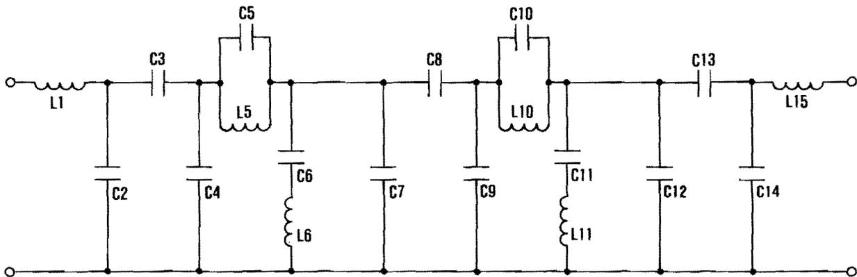
Figure F-1. 27 kHz Elliptical (Cauer) Bandpass Filter
