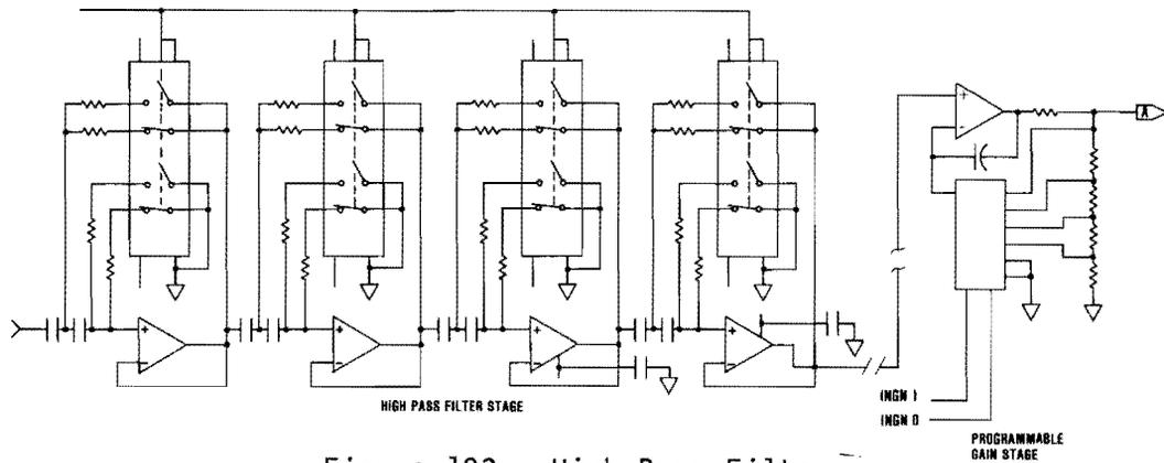
Figure 103. High-Pass Filter
