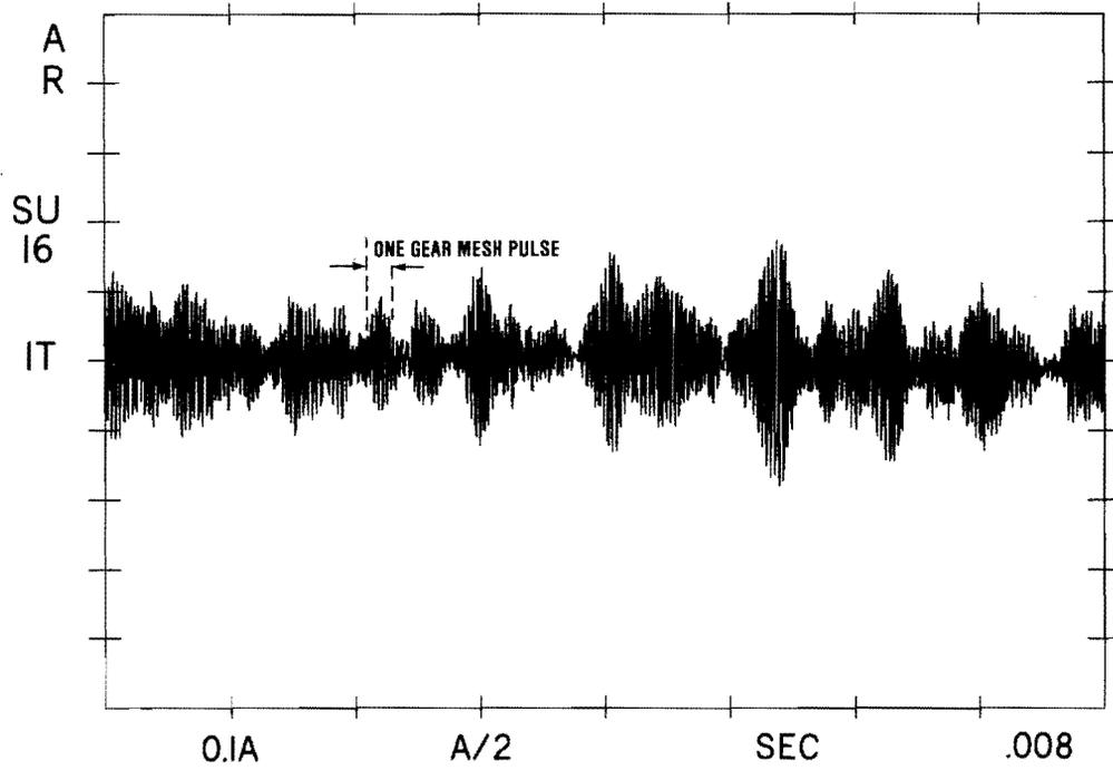
Figure 17. Gear-Mesh Waveform
