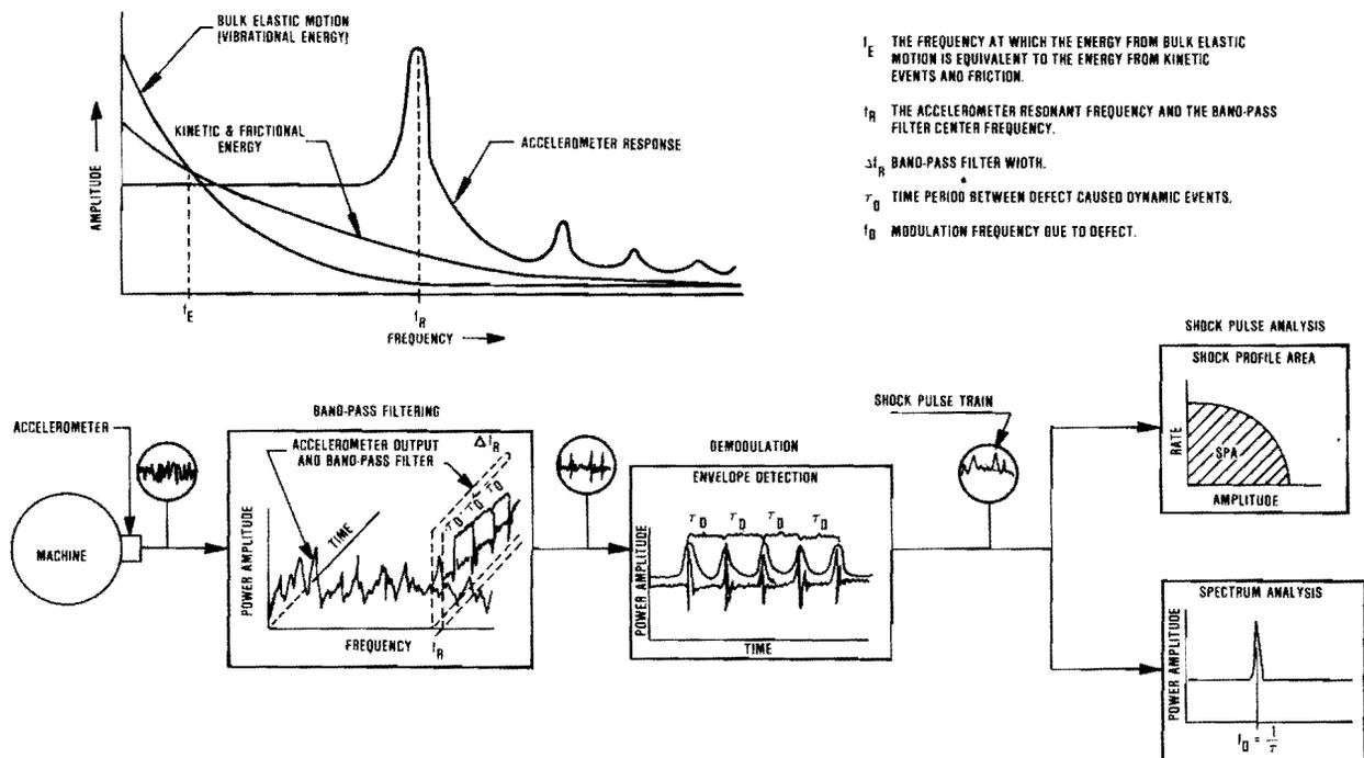
Figure 22. Advance Development Model SPADE System Block Diagram
