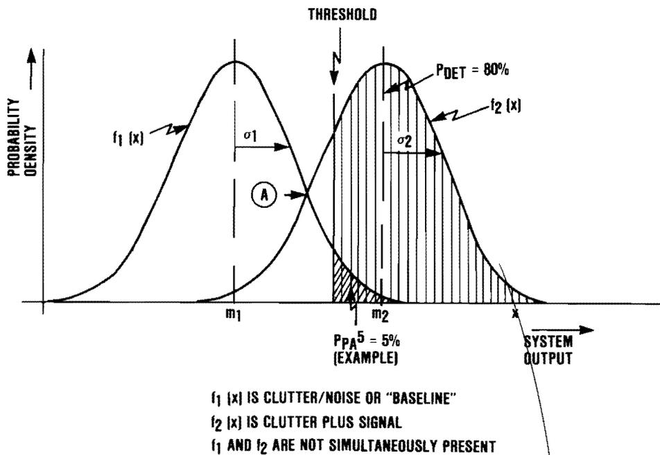
Figure H-1. Relationship of False Alarms and Signal Detection
