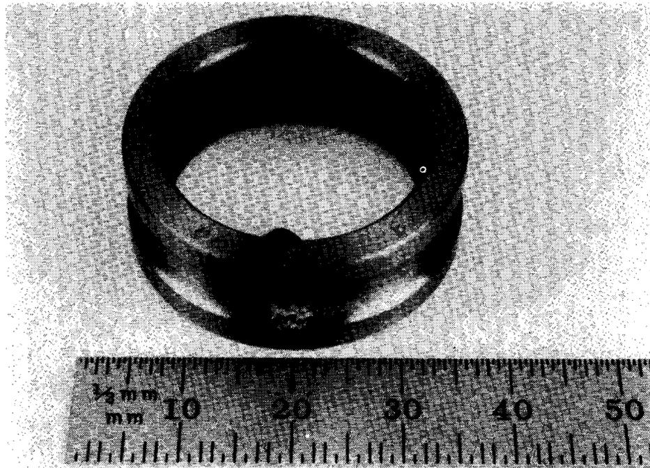
Figure C-52. 90-Degree Gearbox -410 Bearing Inner Race C/D Fault, Runs 9A + 9B
