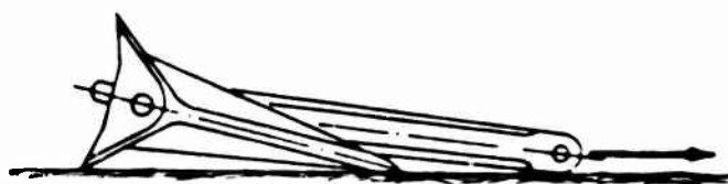
Anchor dragging on hard seafloor with fluke tips unable to bite in.
