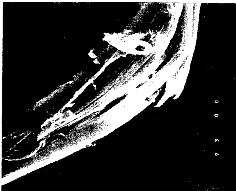
a) Fiber 09273 as spun from a biphasic solution; fractured in liquid nitrogen (x1000).
