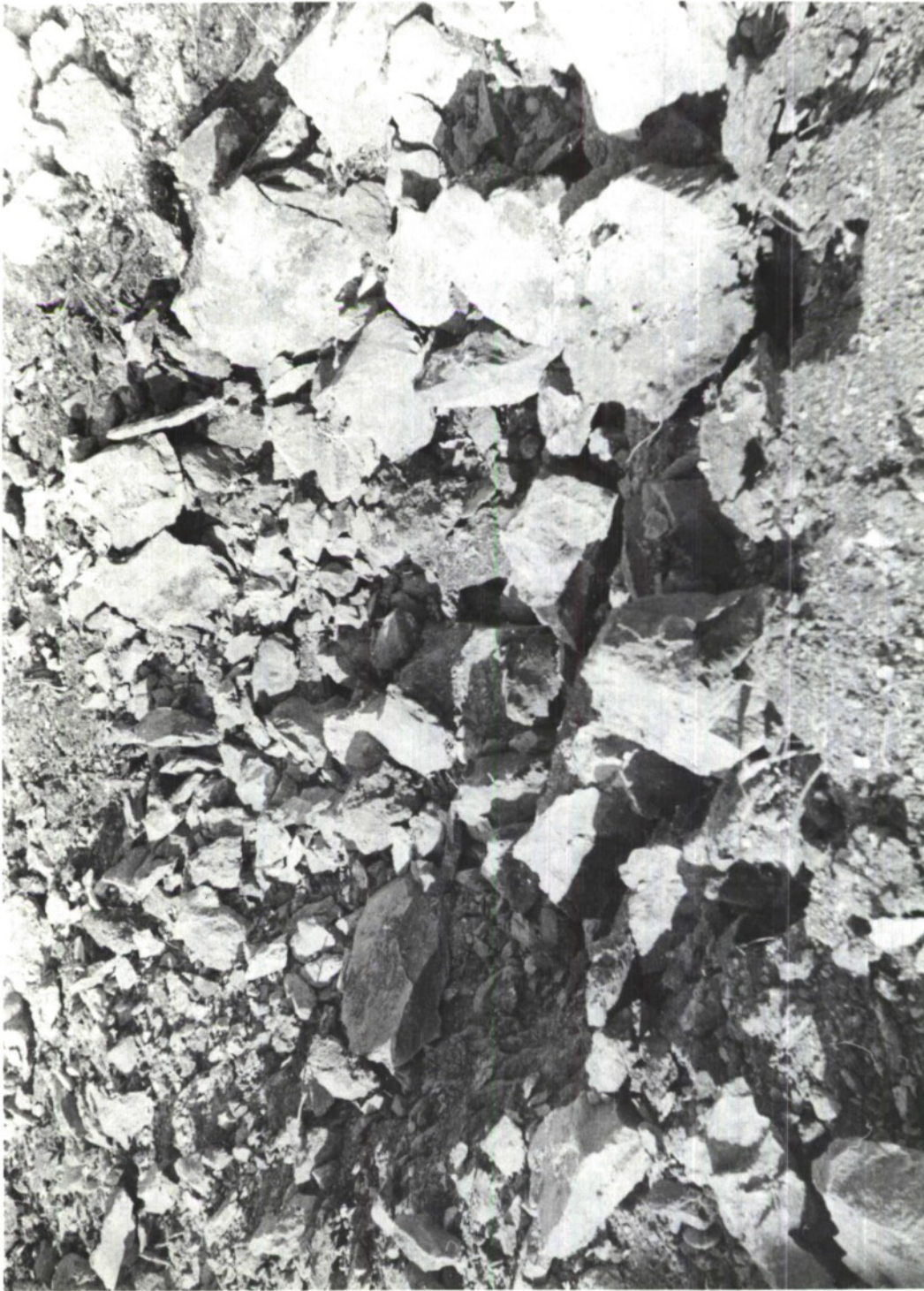
Fig 26 Shot #11: Result of 3 lb of liquid explosive in a 3½'-deep hole produced by an M28A2 HEAT rocket head
