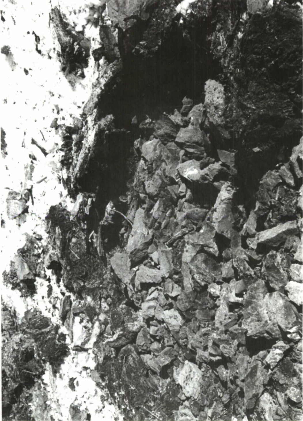
Fig 29 Shot #10: Result of 3 lb of liquid explosive in a 4" dia by 3' deep-bored shot hole
