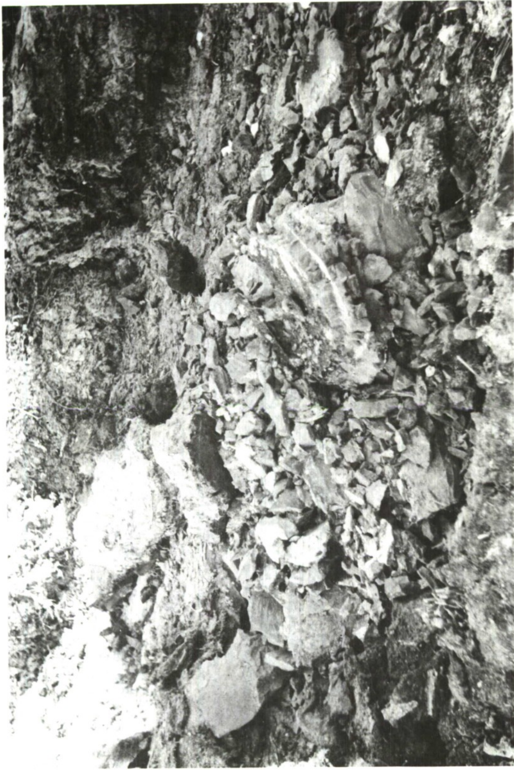
Fig 11 Shot #1: Result of 3 lb of M1 dynamite in a 4" dia x 3' deep-bored shot hole
