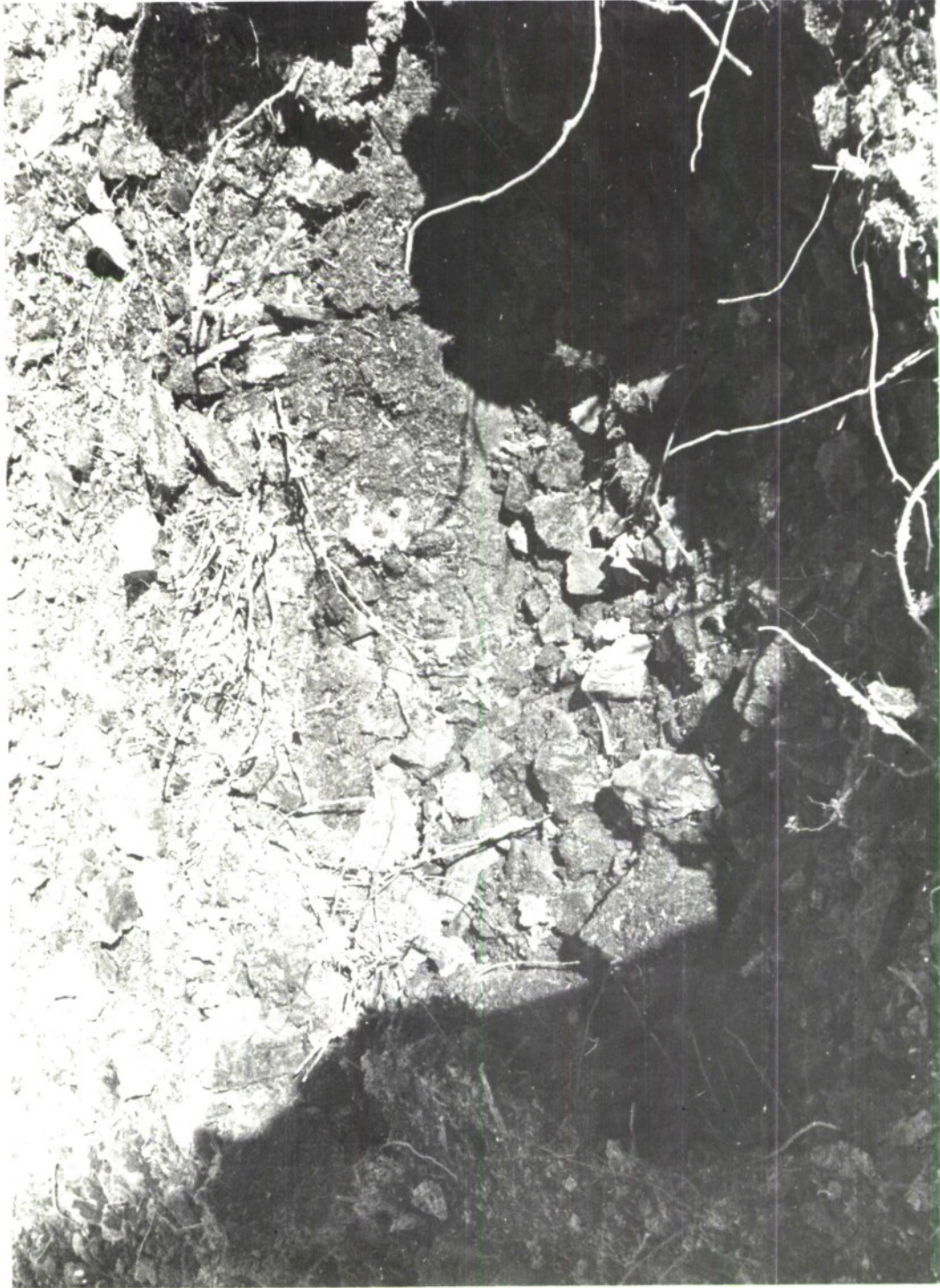
Fig 22 Shot #8: Result of 3 lb of liquid explosive in a 2½" dia by 3' deep-bored shot hole
