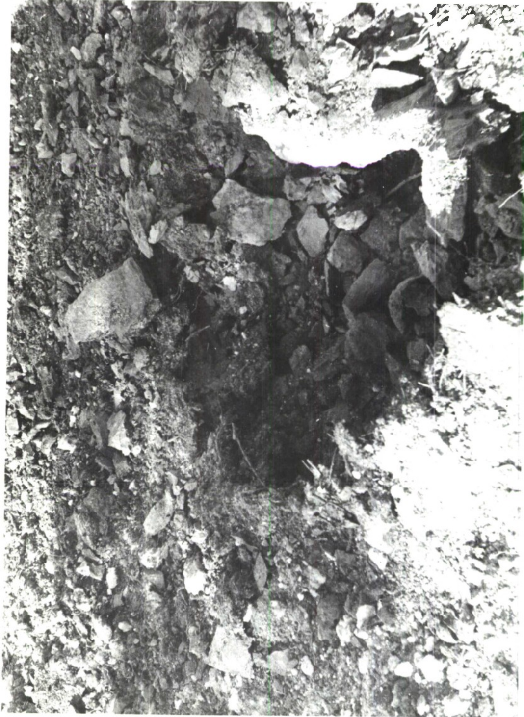
Fig 28 Shot #13: Result of 2 lb of liquid explosive in a 1½'-deep hole produced by an M28A2 HEAT rocket head
