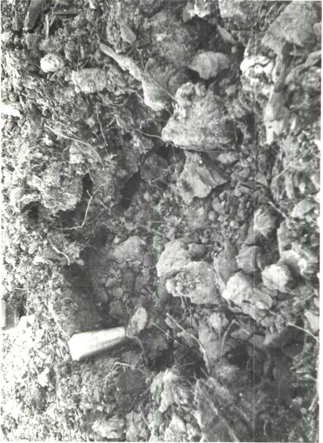
Fig 14 Shot #4: Result of 3 lb of hand-tamped M1 dynamite in a 2½" dia x 3' deep-bored shot hole
