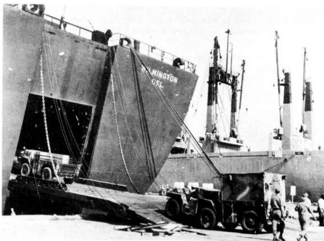
Figure 8-46. RORO Operations GTS Callaghan .
