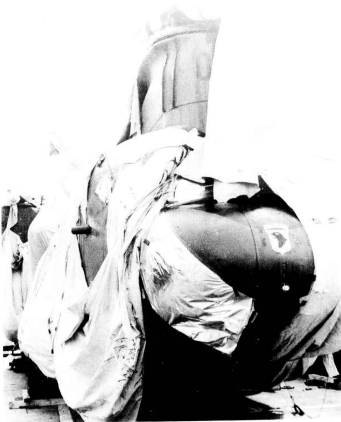
Figure 8-74. Damaged CH-47 Redi-Covers.
