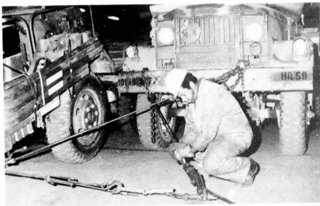
Figure 8-41. Tiedown Restraints Were Carefully Checked.
