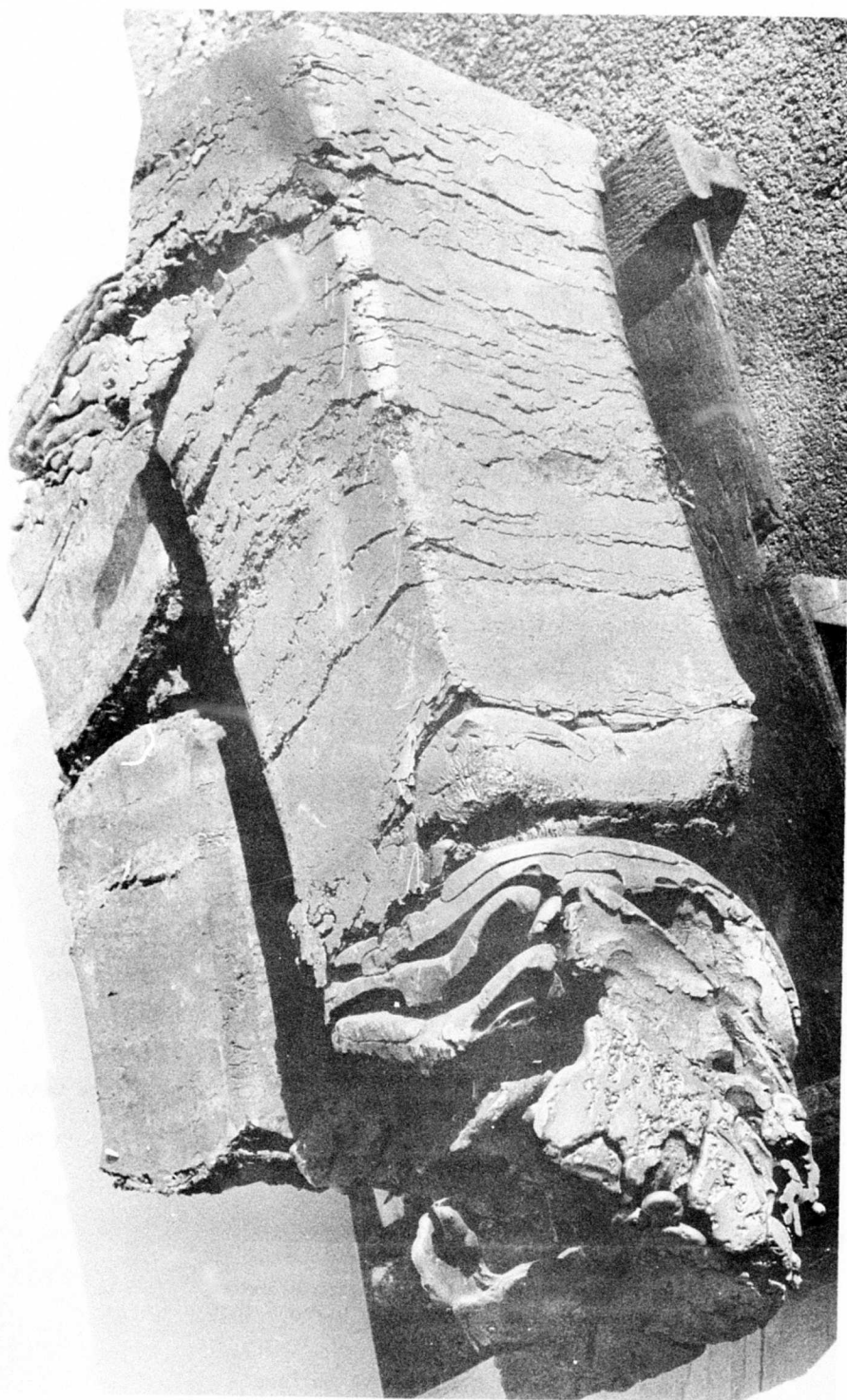
Figure 23 Press Forged Plasmarc Drip Melted Ingots of Inconel 718. (Severe Cracks Seen are at Melt Interruption Locations in the Starting Ingot.)
