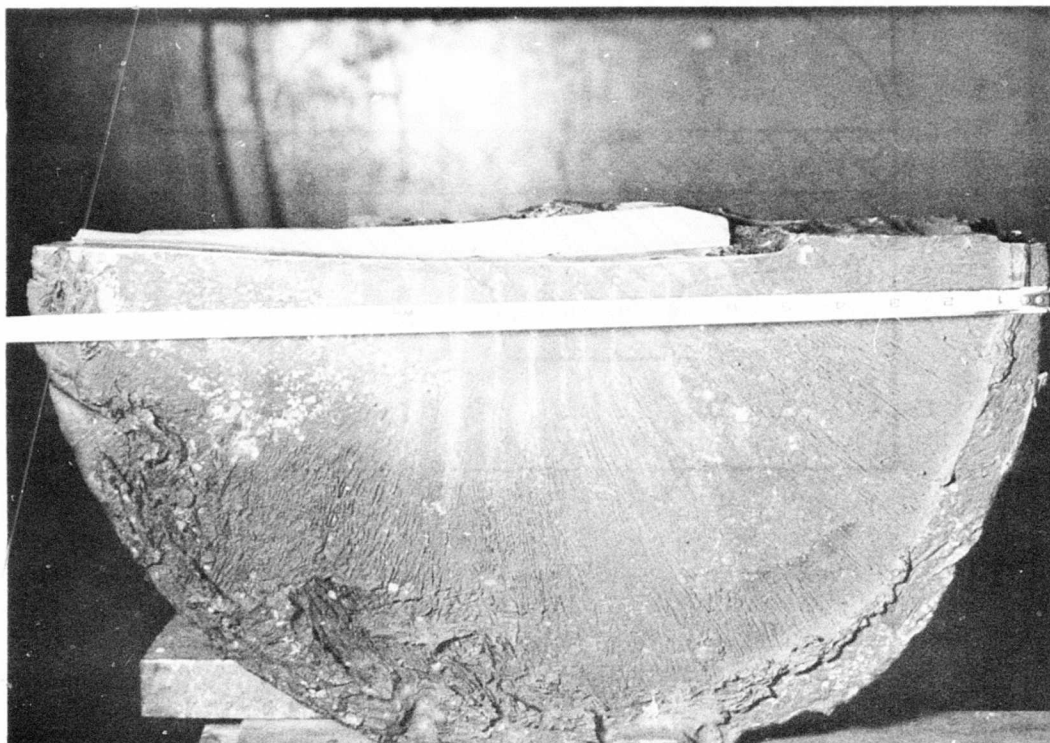
Figure 12 Plasmarc Melted Inconel 718 Ingot (600 lbs.). (Ingot Top Surface Shows No Shrinkage Cavity.)
