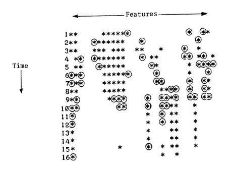
Figure 5. Reference array for word ERASE resulting from merging training data for talkers MH and EC. Encircled points are not common to both talkers.
