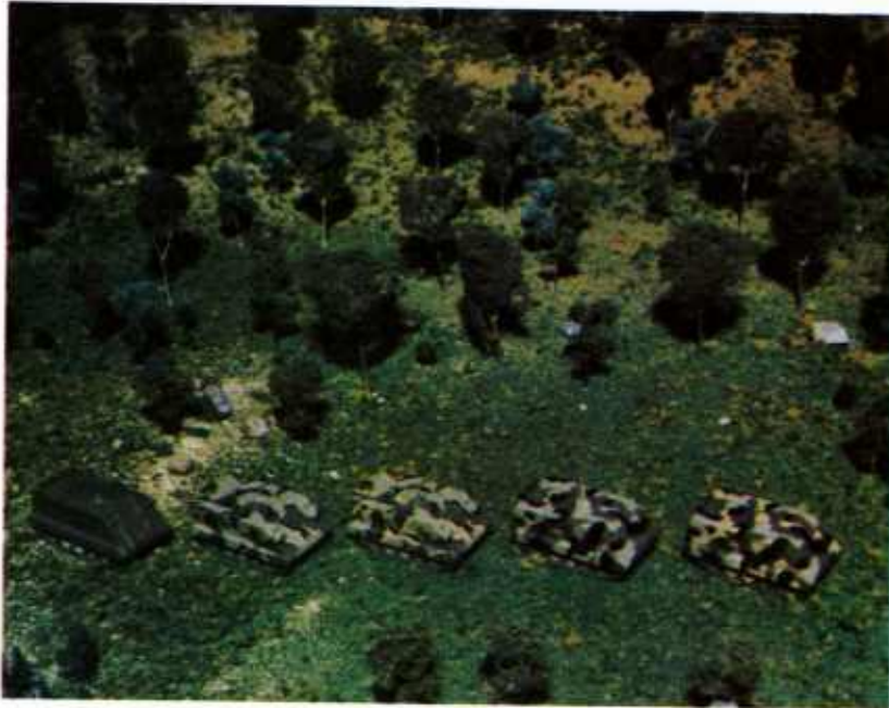
Figure 2. Photographs of the Terrain Model at Two Ranges. The APC's in the Lower Photograph are, from Left to Right, FG, M3, M4, S3, and S4.
