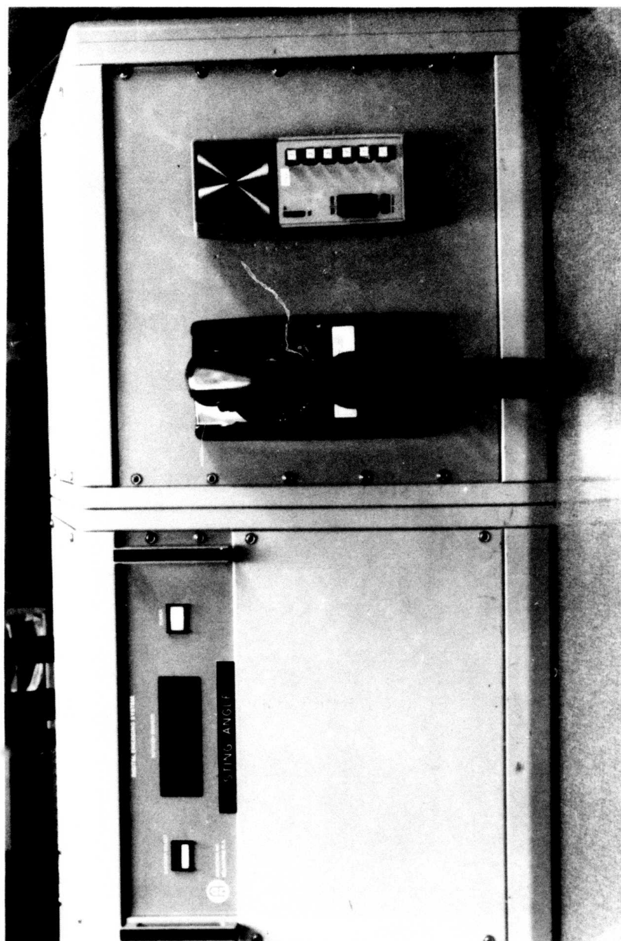
Figure 9. Sting Angle Indicator and Communication Panel
