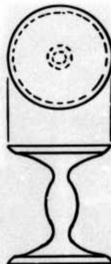
Figure 76. Recommended chaplet design for emergency use.
