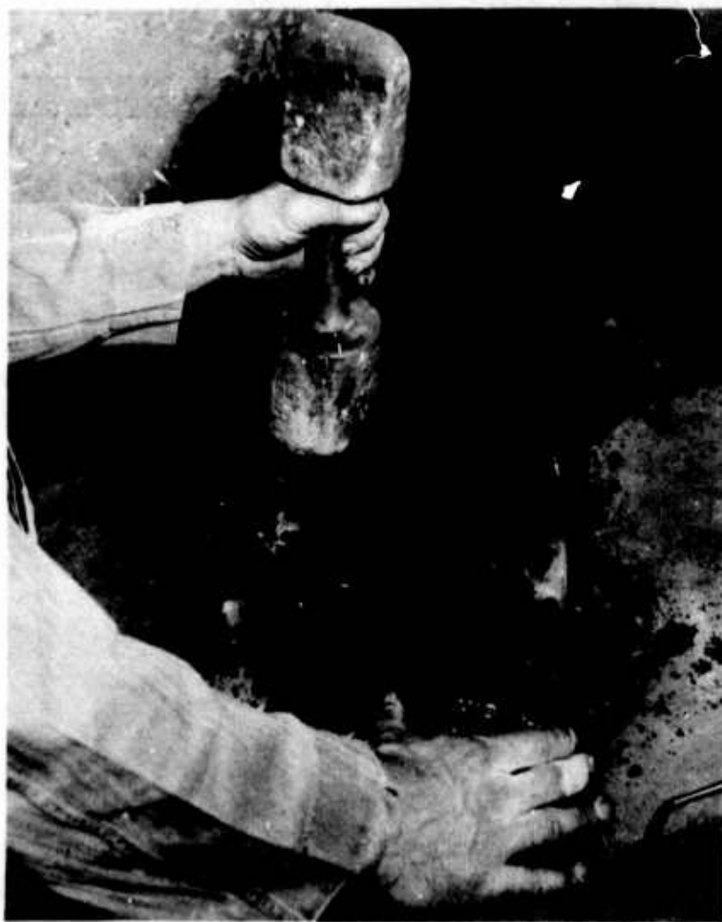
Figure 103. Ramming up the core.
