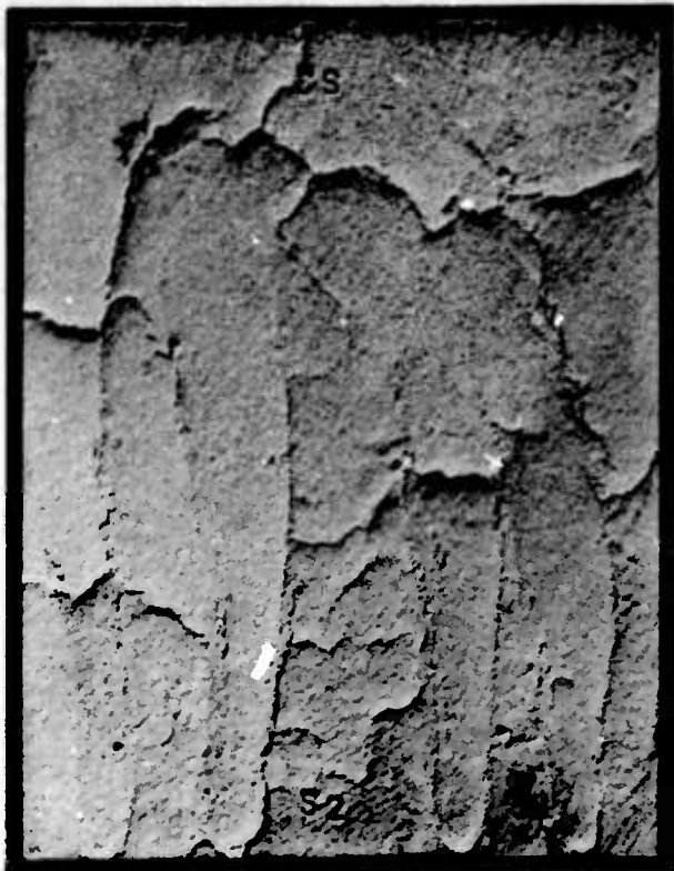
Figure 212. Rattails. (Sand lacked good expansion properties)
