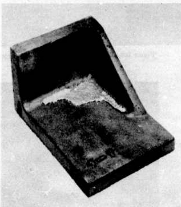
Figure 207. Expansion scab. (Caused by too many fines in the sand)
