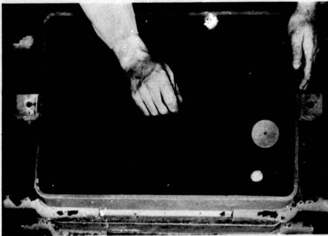
Figure 85. Venting the cope.
