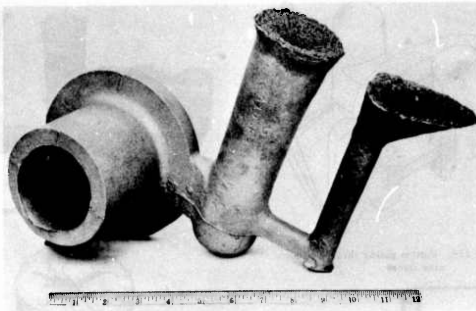
Figure 125. Parting gate through the riser.
