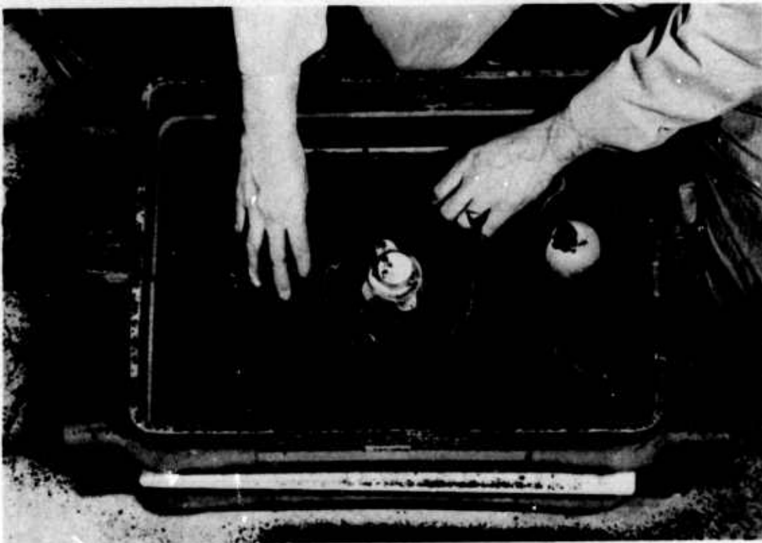
Figure 79. Hand packing riddled sand around the pattern.
