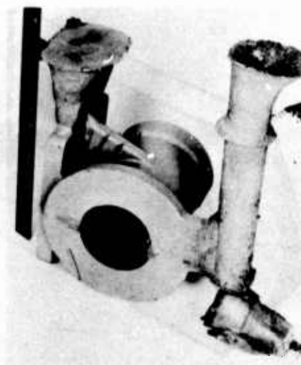
Figure 138. Cold metal riser. (Not Recommended)
