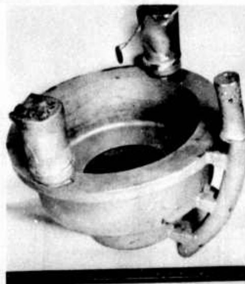
Figure 136. Proper riser size and shape.
