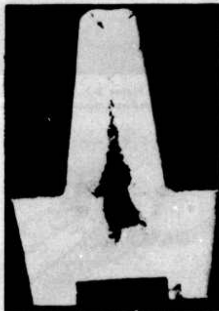
Figure 199. Gross shrink. (Caused by inadequate feeding)
