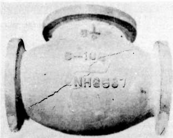
Figure 215. Cracked casting. (Caused by a hard core)
