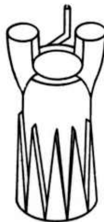
Figure 237. Tapered chills on a G metal bushing.
