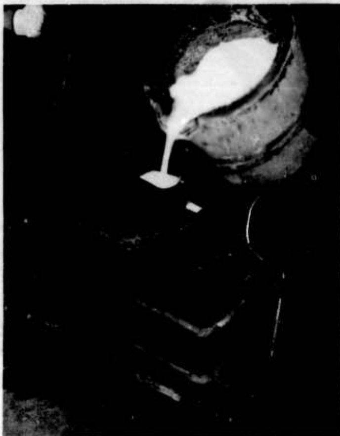
Figure 91. Pouring the mold.
