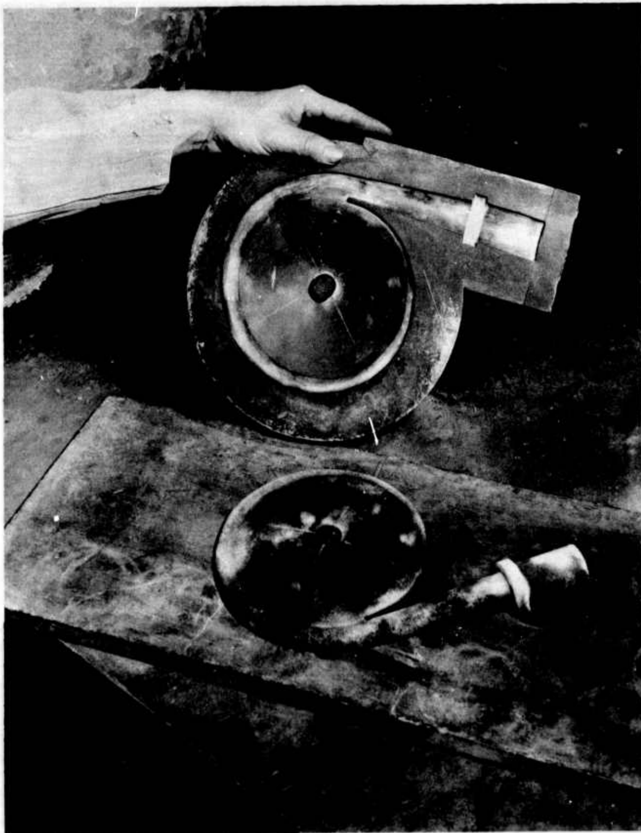
Figure 107. Drag core turned out.
