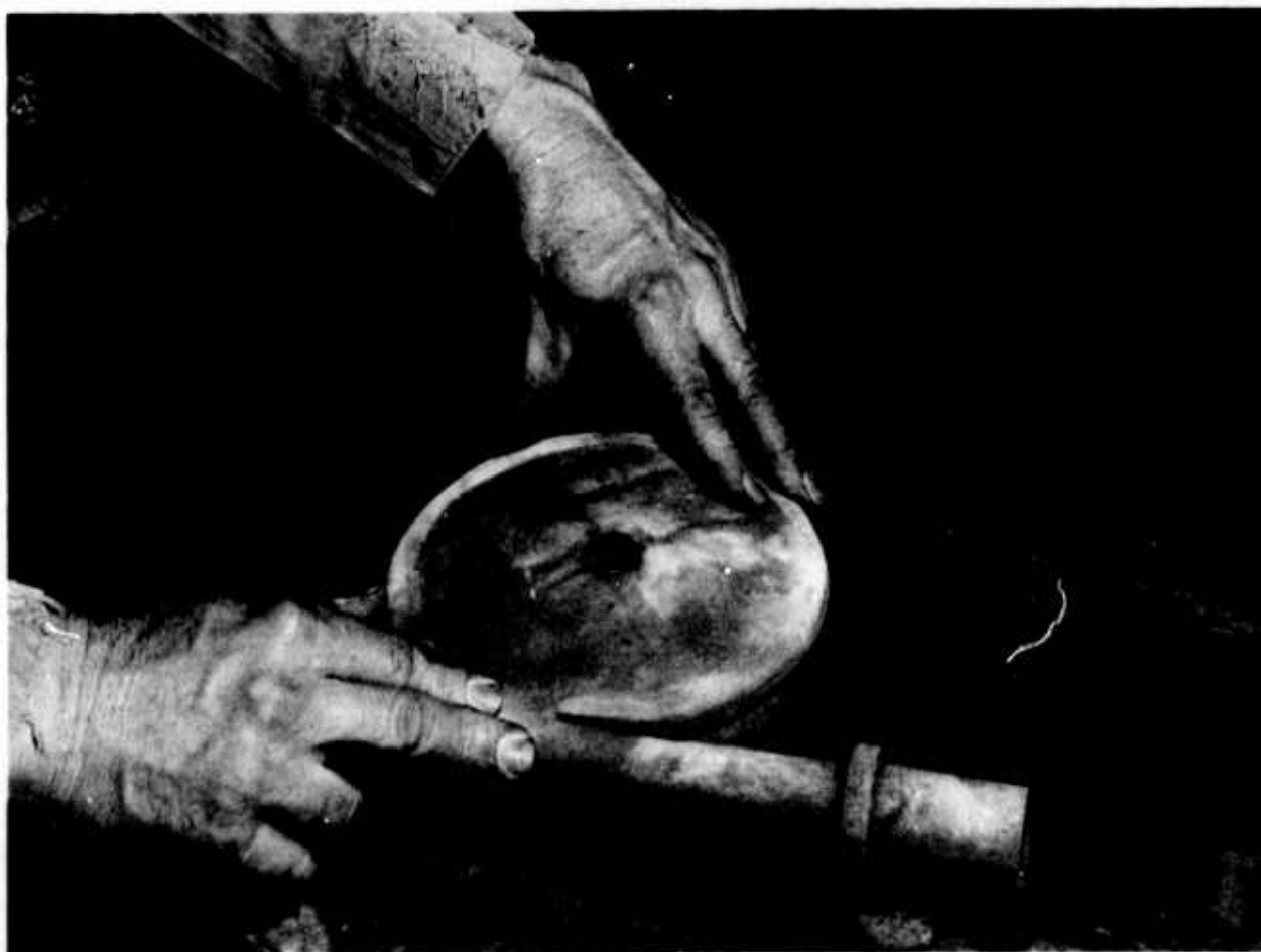
Figure 110. Assembling the two core halves.
