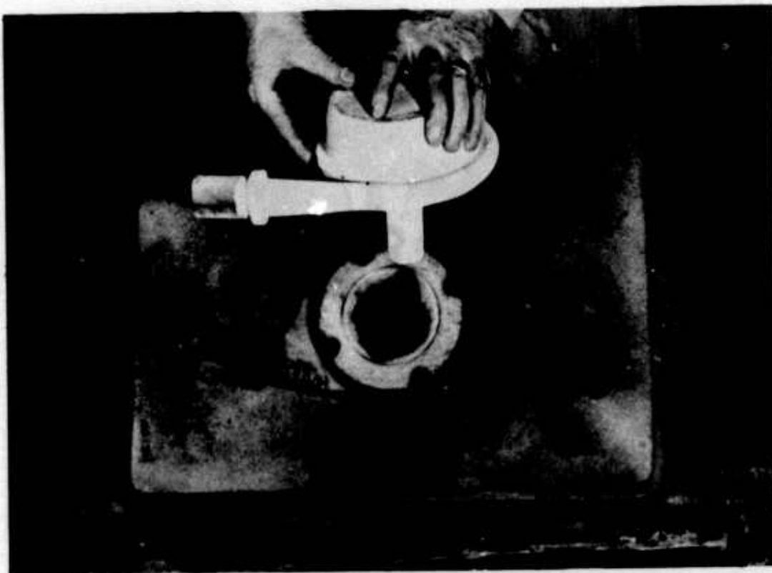
Figure 88. Setting the core.
