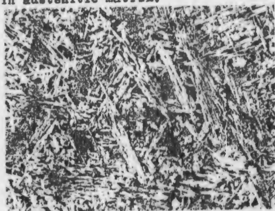
X100 Nital Picral 1.4" thick plate as cast. Center of steel base. Widmanstätten structure, sorbite and ferrite.
