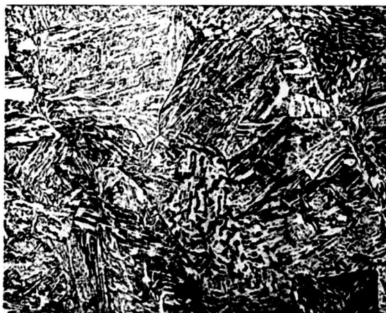
X200 Nital Picral Middle of cross-section. Coarse structure with considerable ferrite.
