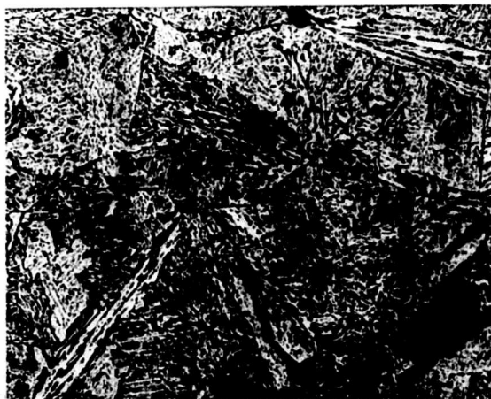
X200 Nital Picral Outer third of cross-section. Coarse structure with less ferrite.
