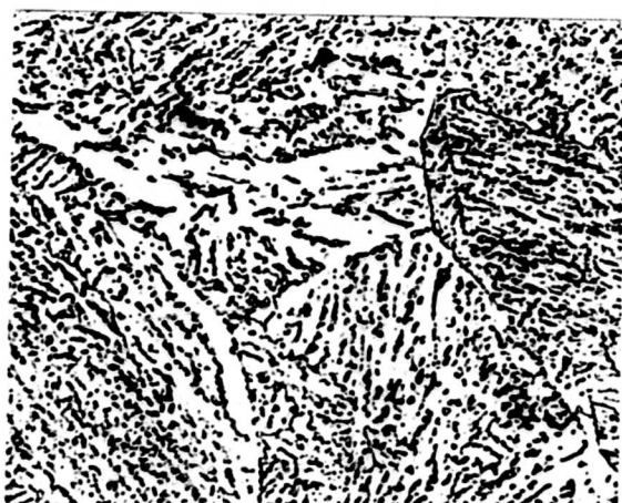
X1000 Nital Picral Outer third of cross-section. Sorbite, ferrite, and grain boundary carbides.
