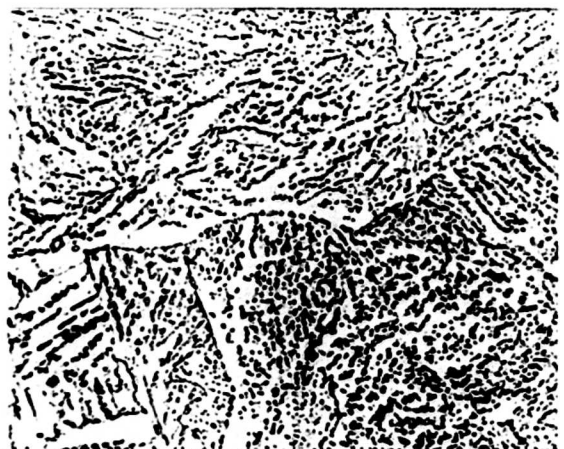
X1000 Nital Picral Outer third of cross-section. Sorbite, ferrite, and grain boundary carbides. Less ferrite than in midsection.
