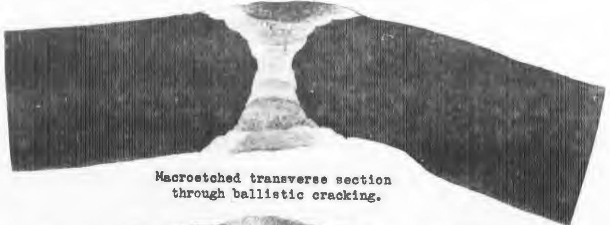
Macroetched transverse section through ballistic cracking.
