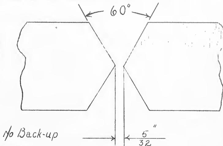
PLATE PREPARATION: FLAME POLYMER
