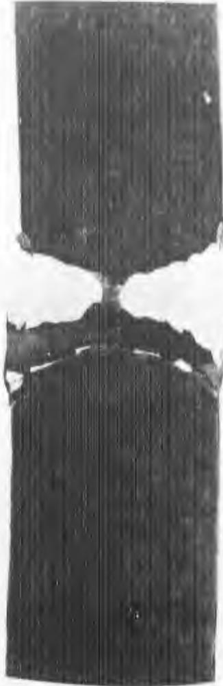
Macroetched transverse section through ballistic fracture.
