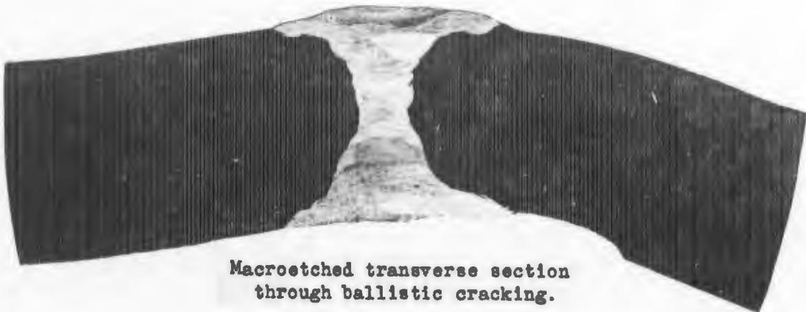
Macroetched transverse section through ballistic cracking.
