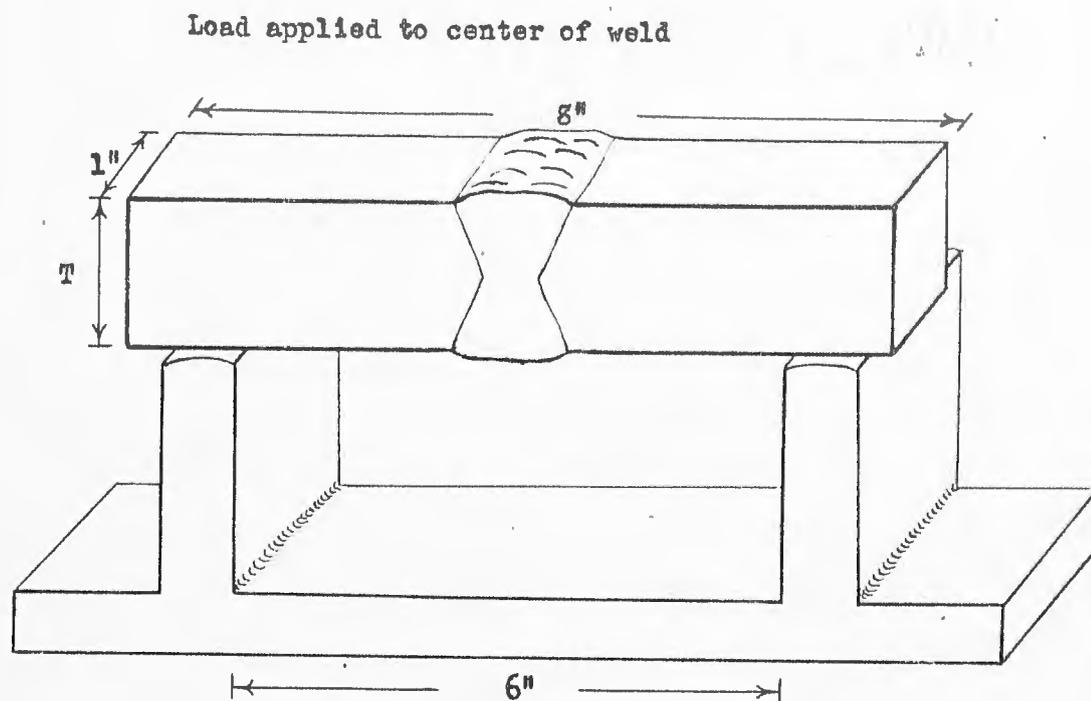
Supported on six-inch span; bars of 1 inch and 1 1/2 inch thickness broken in a steam press; bars of lesser thickness broken with one blow of drop weight
