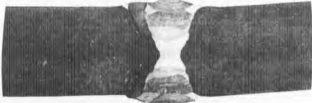
Macroetched transverse section through ballistic fracture.
