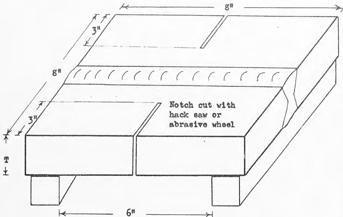
Supported on six-inch span; broken with one blow of drop weight or steam hammer
