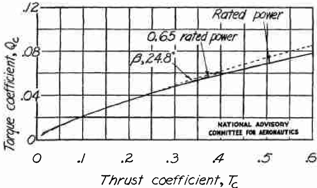
Figure 5.- Comparison of variation of  $T_c$  with  $Q_c$  for constant-power operation and for the propeller with blade angle fixed at  $24.8^\circ$  at 0.75 radius.
