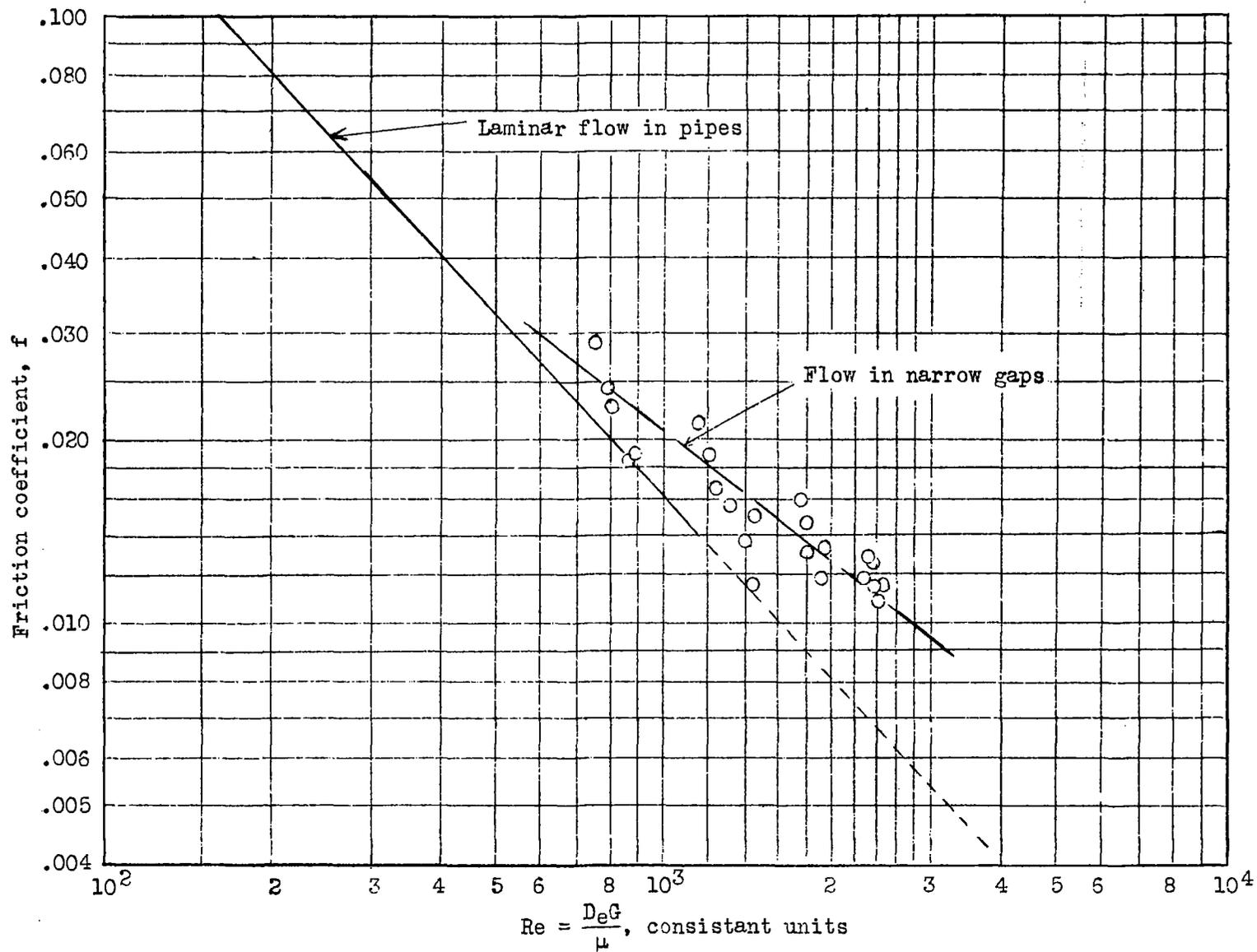
Figure 24.- The relation between the friction factor and Reynolds number for flow of air in pipes, ( $D_e$  = diameter, ft); and in narrow gaps between parallel surfaces, ( $D_e$  = gap width, ft) Taken from figure 8, reference 5.
