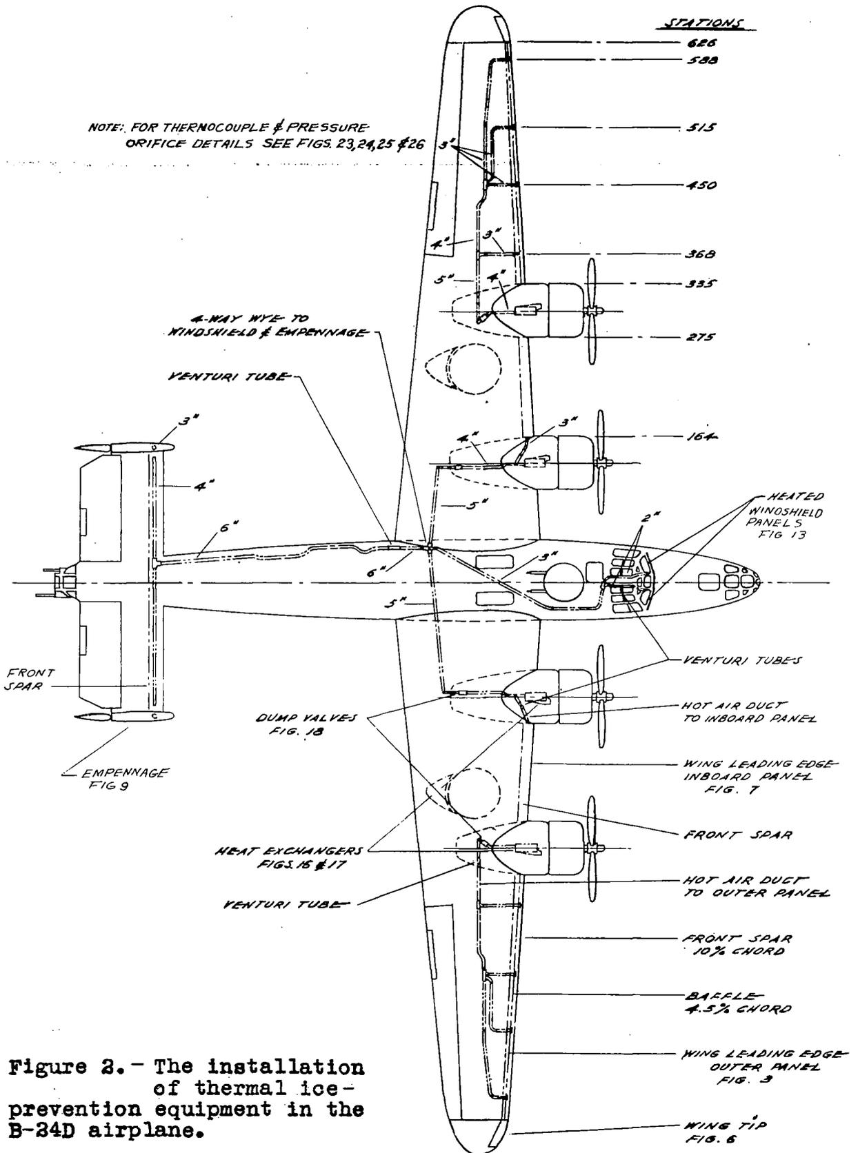
Figure 2.- The installation of thermal ice-prevention equipment in the B-24D airplane.
