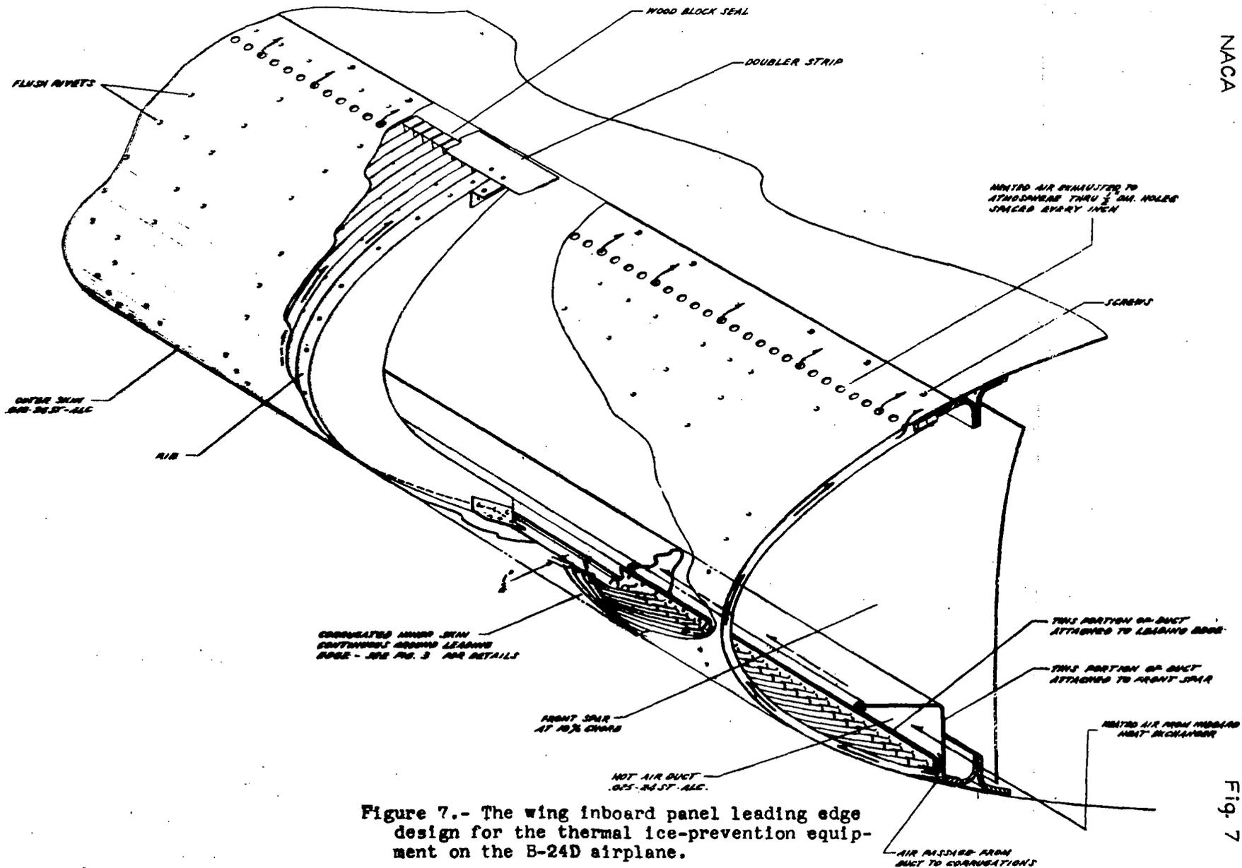
Figure 7.- The wing inboard panel leading edge design for the thermal ice-prevention equipment on the B-24D airplane.
