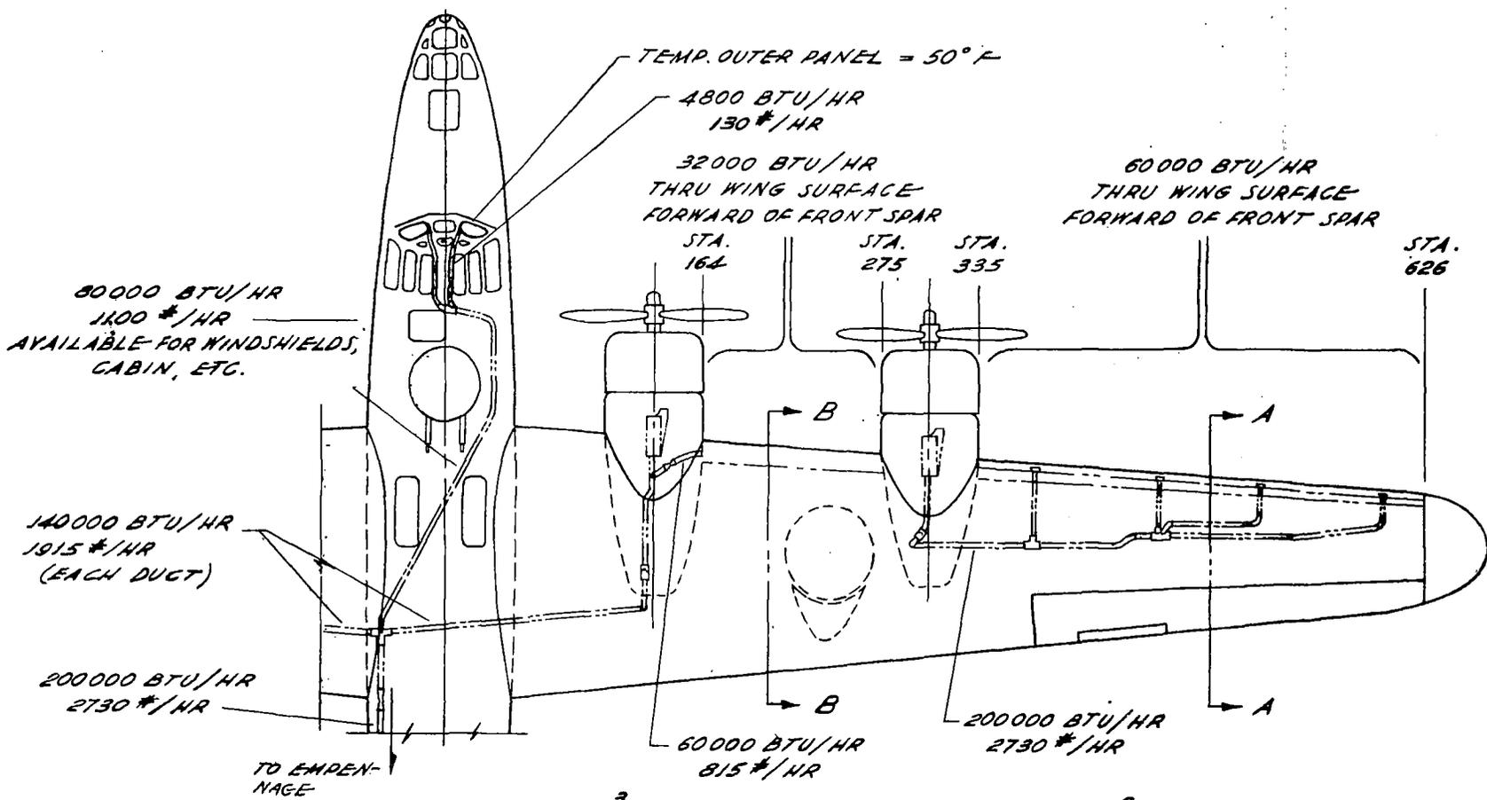
Figure 20.- The results of the analysis of the thermal ice-prevention equipment, showing the distribution of the heated air in the wings and windshield in the B-24D airplane.
