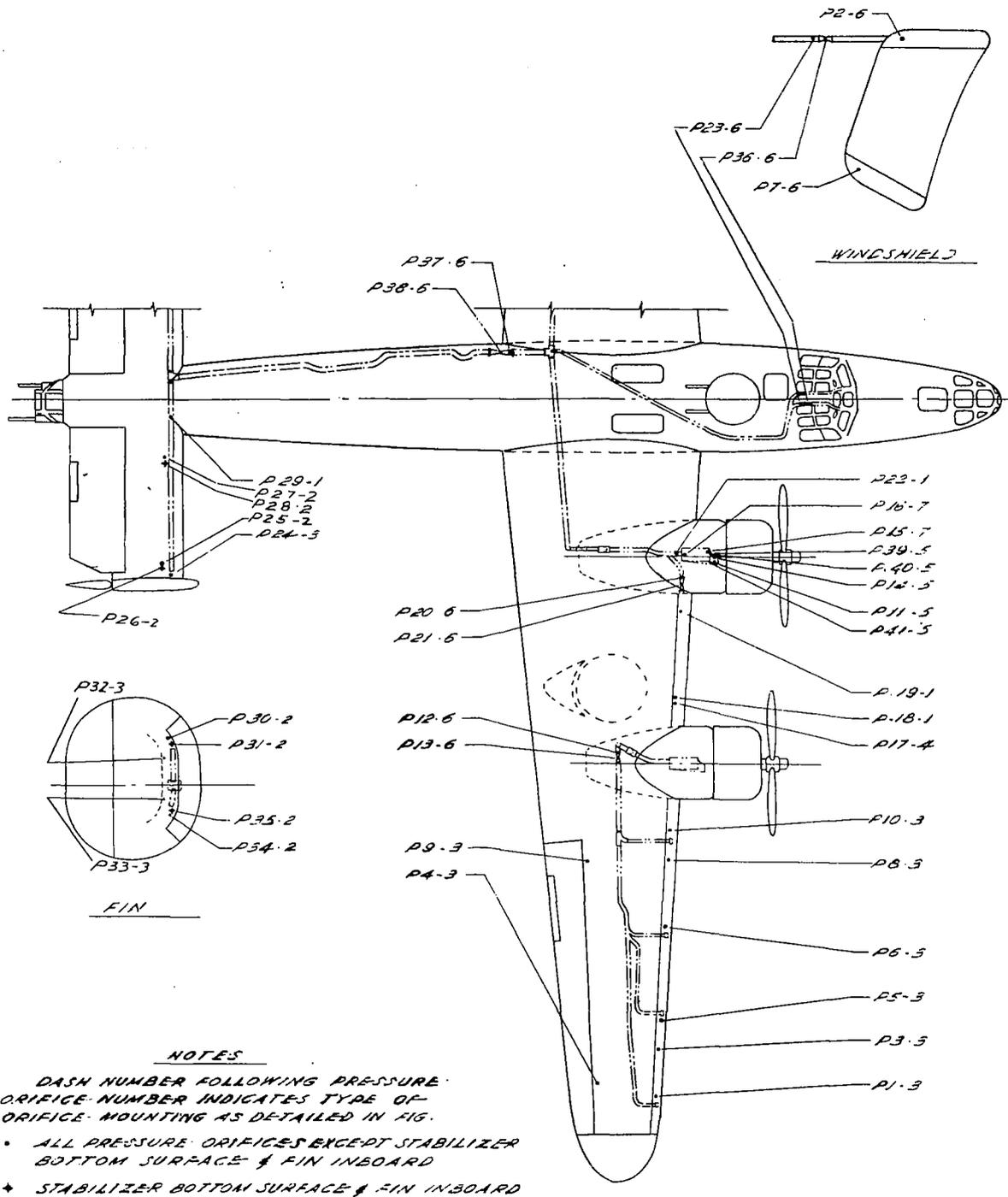
Figure 27.- The pressure orifices which were installed on the B-24D airplane and which were employed in studying the thermal qualities of the ice-prevention equipment.
