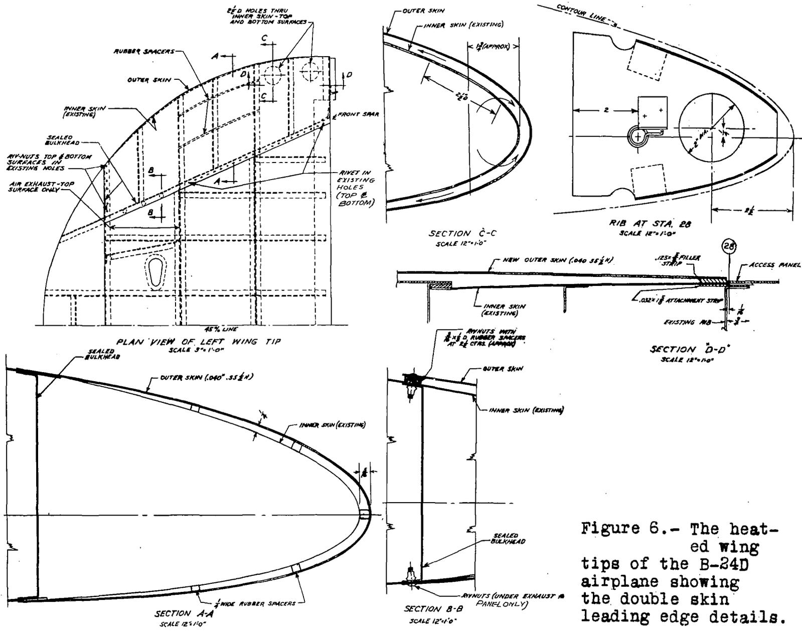
Figure 6.- The heat-treated wing tips of the B-34D airplane showing the double skin leading edge details.
