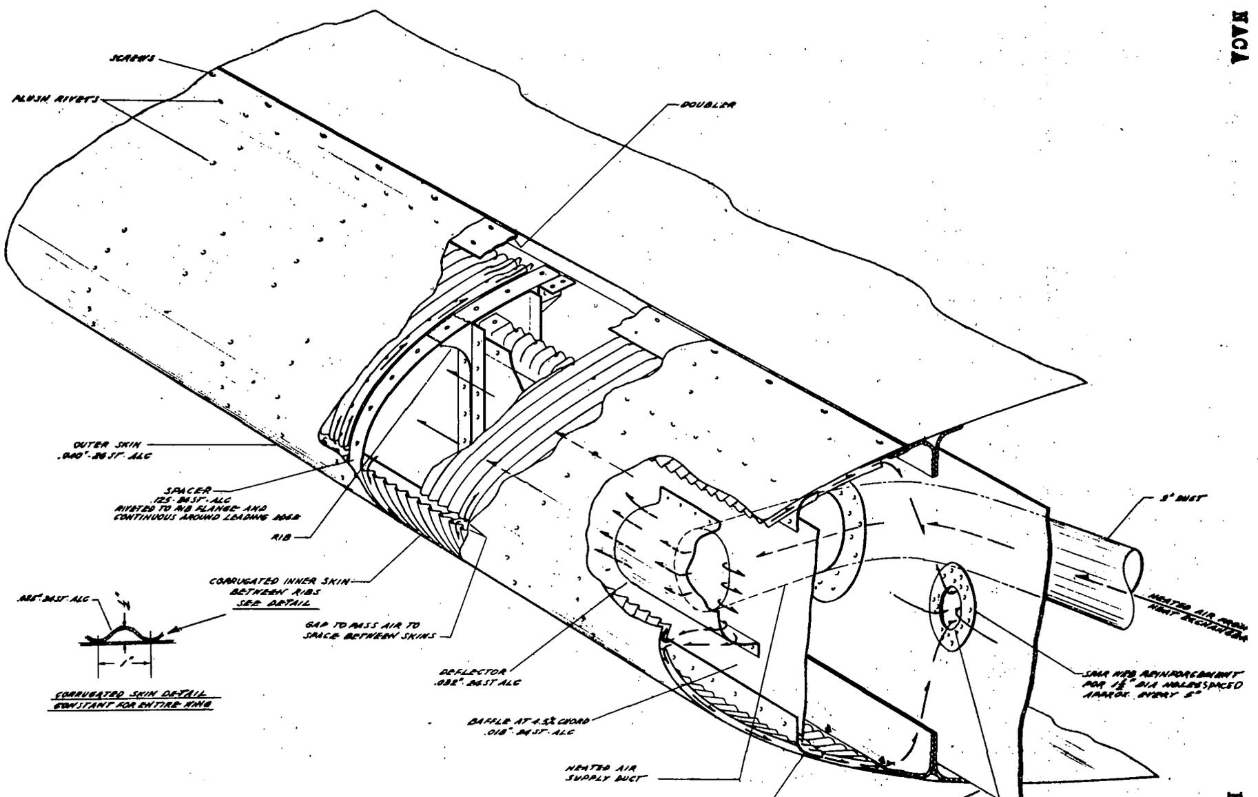
Figure 3.- The wing outer panel leading-edge design for the thermal ice-prevention equipment on the B-24D airplane.
