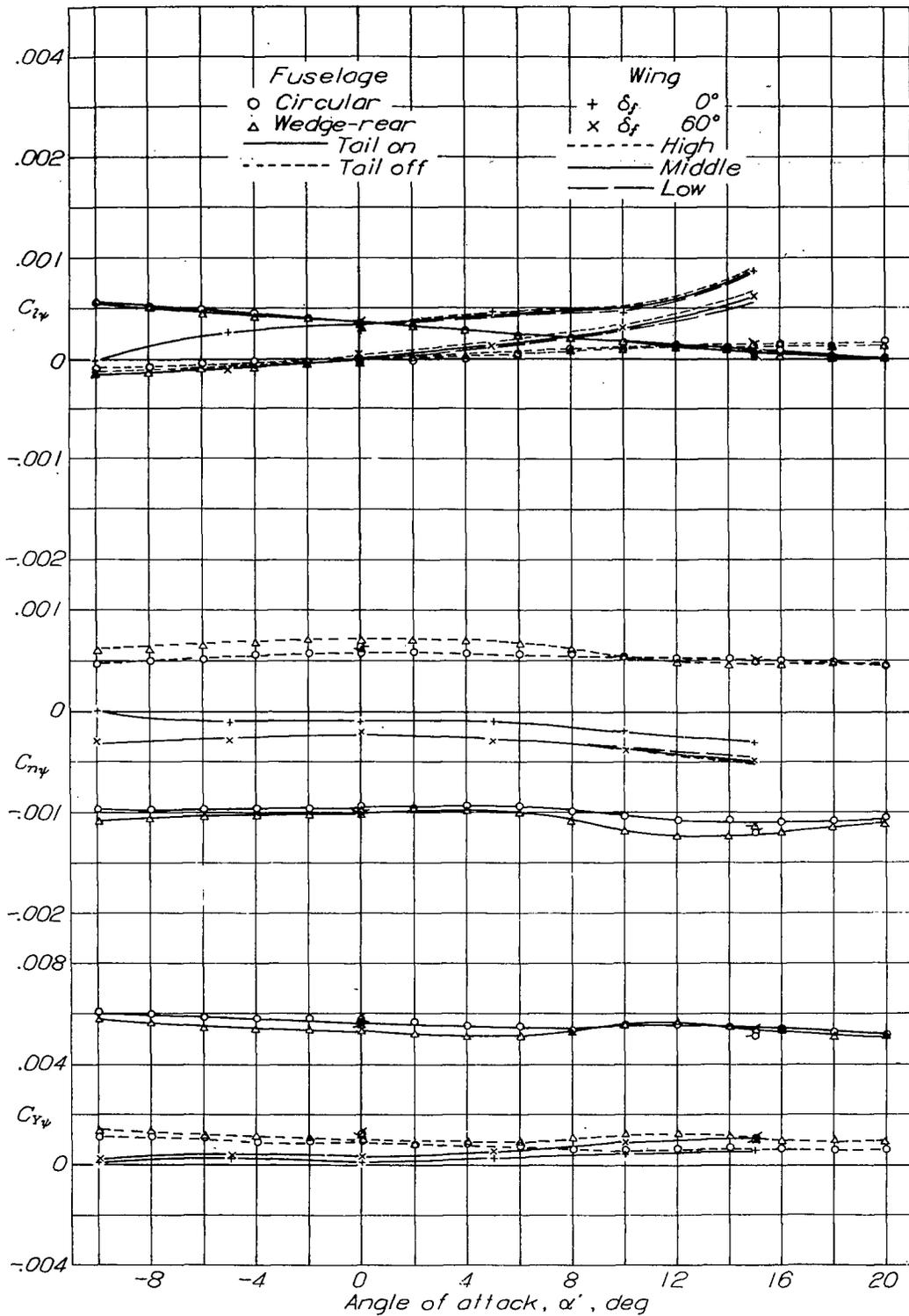
Figure 3.- Variation of  $C_{l\psi}$ ,  $C_{n\psi}$ , and  $C_{y\psi}$  with angle of attack. NACA 23012 wing alone, fuselage alone, and fuselage with tail. (Data for wing and circular fuselage converted from references 7 and 1, respectively.)
