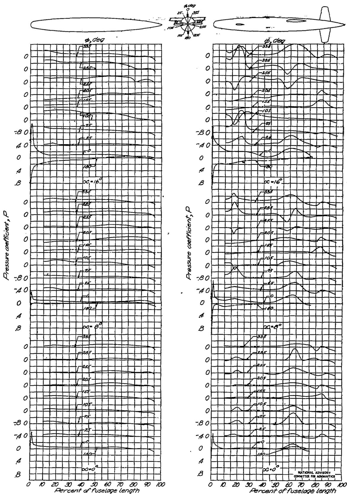
Figure 4.- Fuselage pressure distribution for several positions of the generator.  $\mu = 5^\circ$ .
