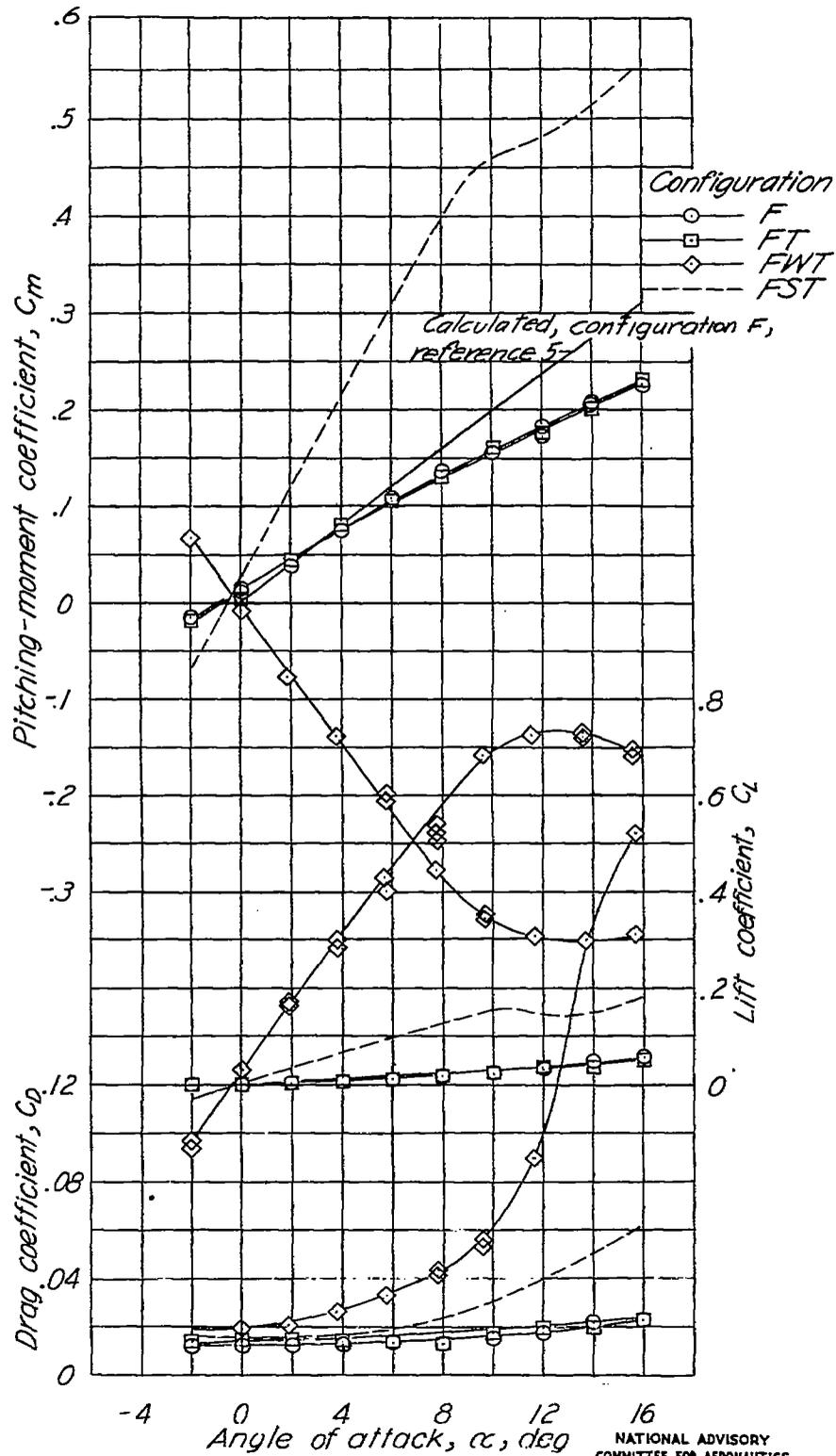
Figure 9. - Variation of lift, drag, and pitching-moment coefficients with angle of attack for several configurations.  $\mu=0^\circ$ .
