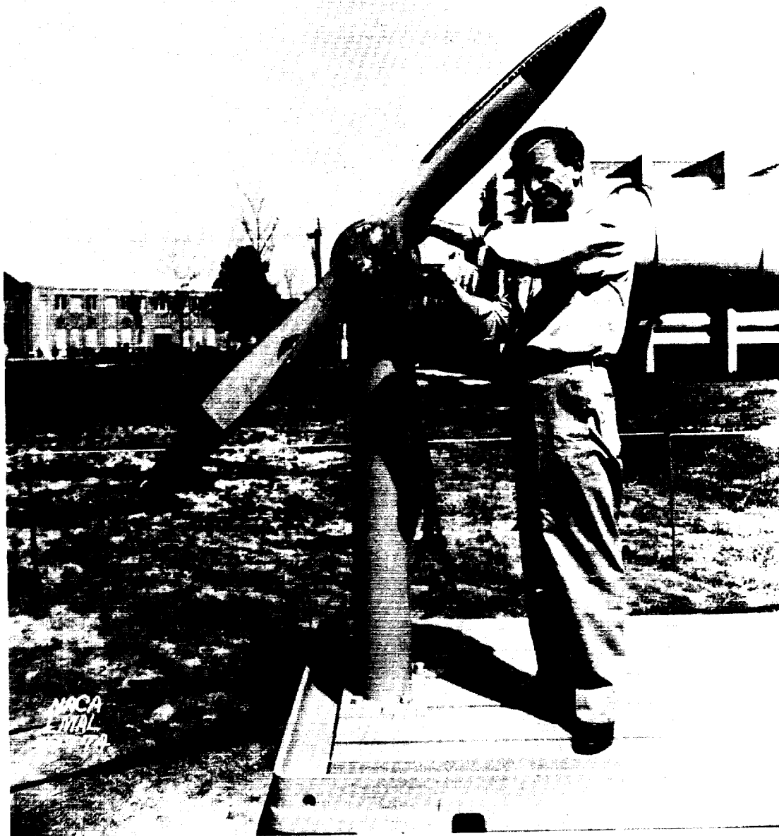
(b) Two-blade propeller mounted on test stand.
