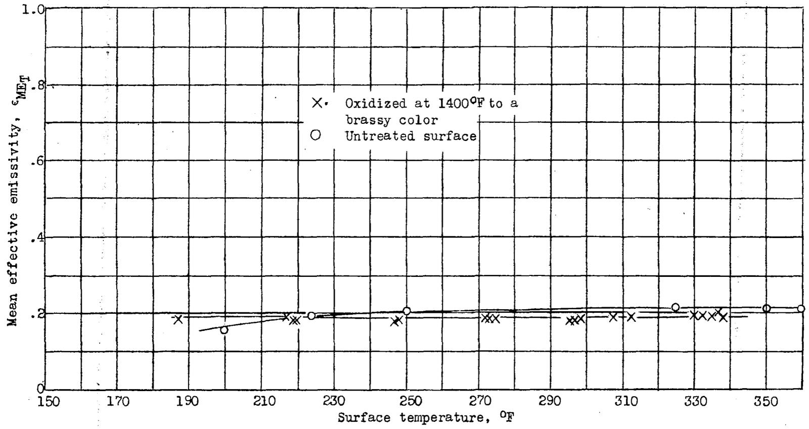
Figure 2.- Emissivity of Inconel as a function of temperature.
