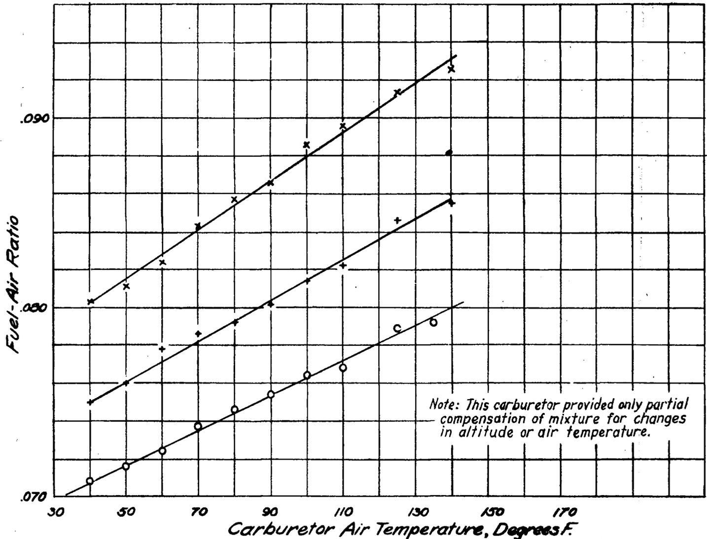
Figure 4 Effect of Carburetor Air Temperature on Fuel/Air Ratio
