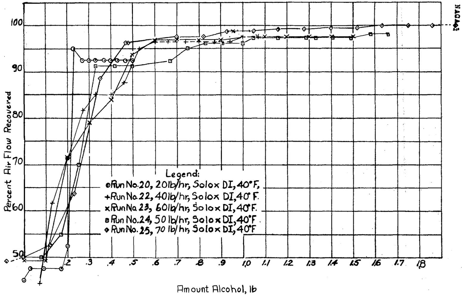
Figure 30. — Air Flow Recovery versus Alcohol Amount, Holley Ring, De-icing Fluid, Solox DI, Water Discontinued When Alcohol Flow Started; Initial Air Flow 4000 lb/hr; Initial Fuel Air Ratio .070
