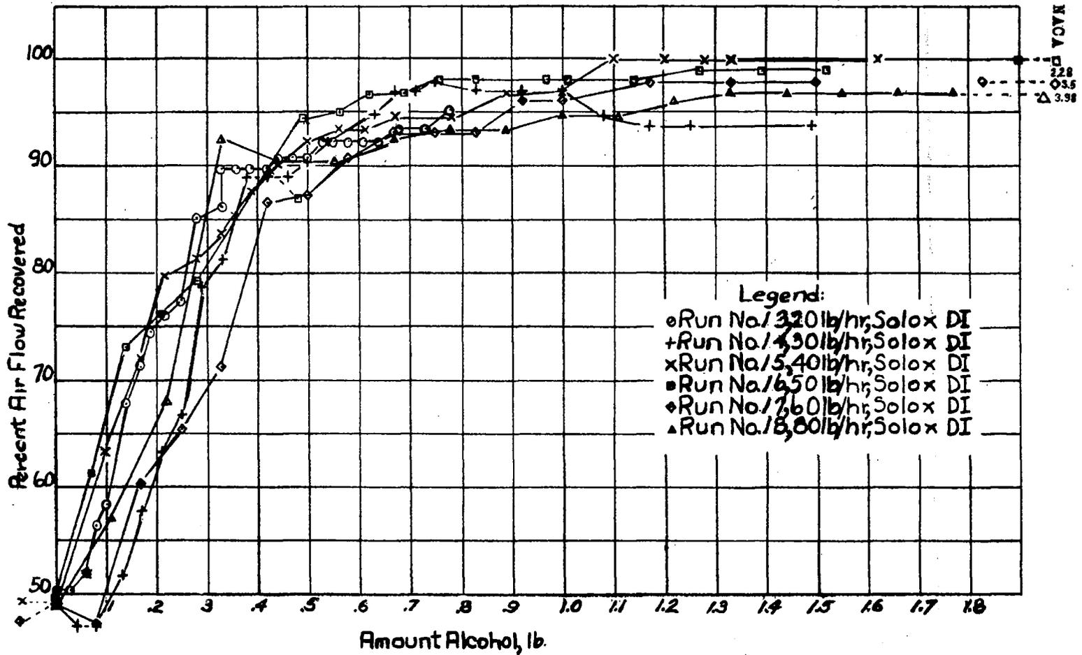
Figure 29.— Air Flow Recovery versus Alcohol Amount; Holley Ring; De-icing Fluid, Solox DI; Water Injected Throughout Tests, Initial Air Flow 4000 lb/hr, Initial Fuel Air Ratio 0.70
