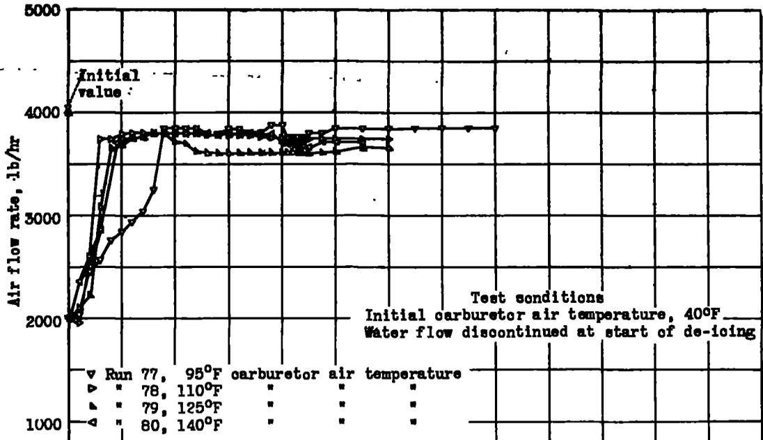
Figure 35b.- De-icing by means of heated air - Series M.
