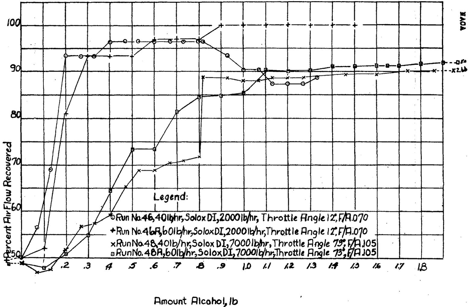
Figure 32. — Air Flow Recovery versus Alcohol Amount, Holley Ring; De-icing Fluid, Solox DI; Water Injected Throughout Tests,
