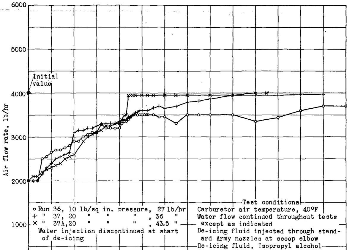
Figure 19.- De-icing by means of fluid at cruising throttle - Series E.
