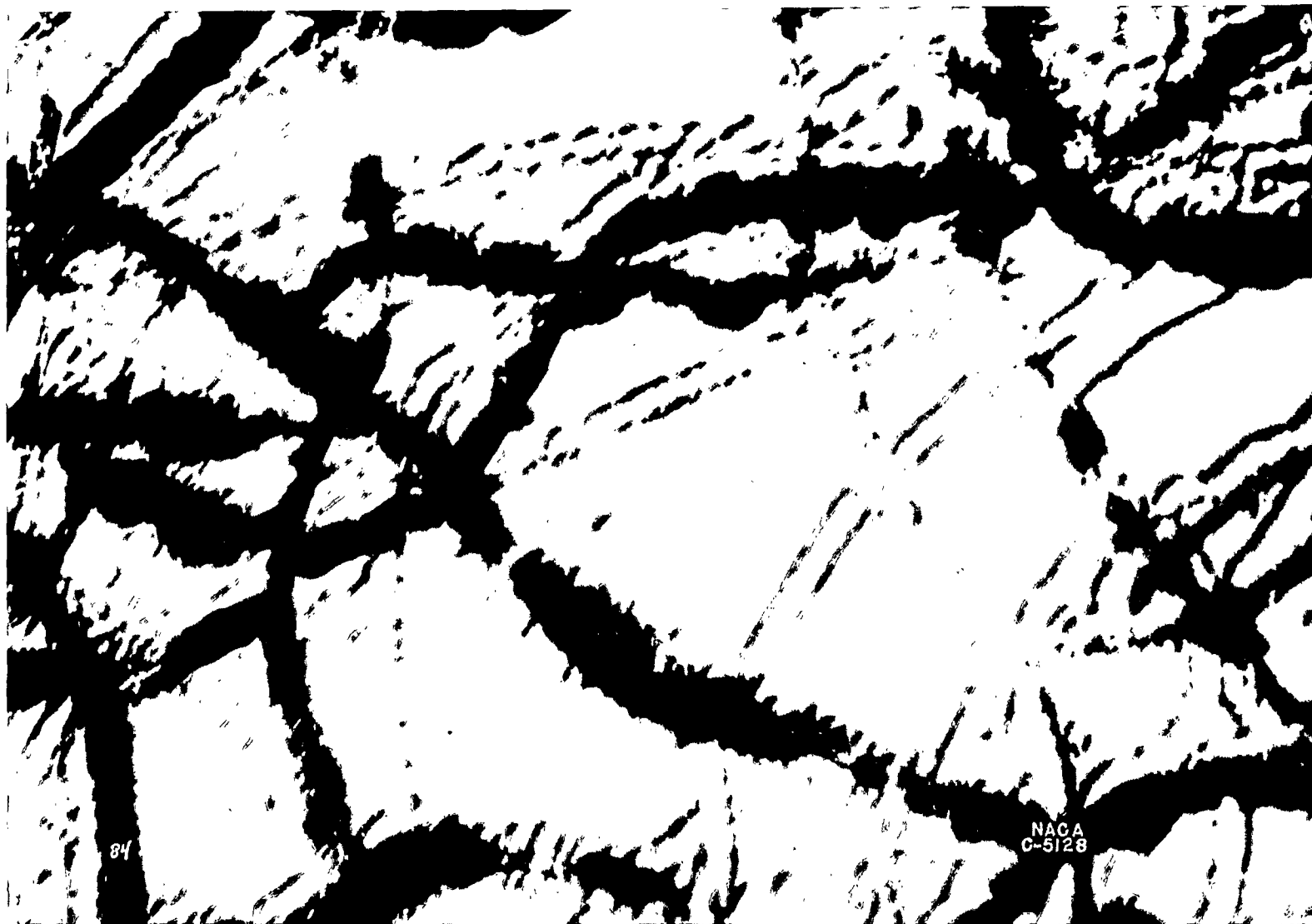
Figure 6. - Photomicrograph of choke-bore porous chrome-plated cylinder barrel representative of barrel surfaces at the middle of ring travel on the major-thrust face. Condition before silver plating and before test 8. Estimated porosity, 40 percent. X108.
