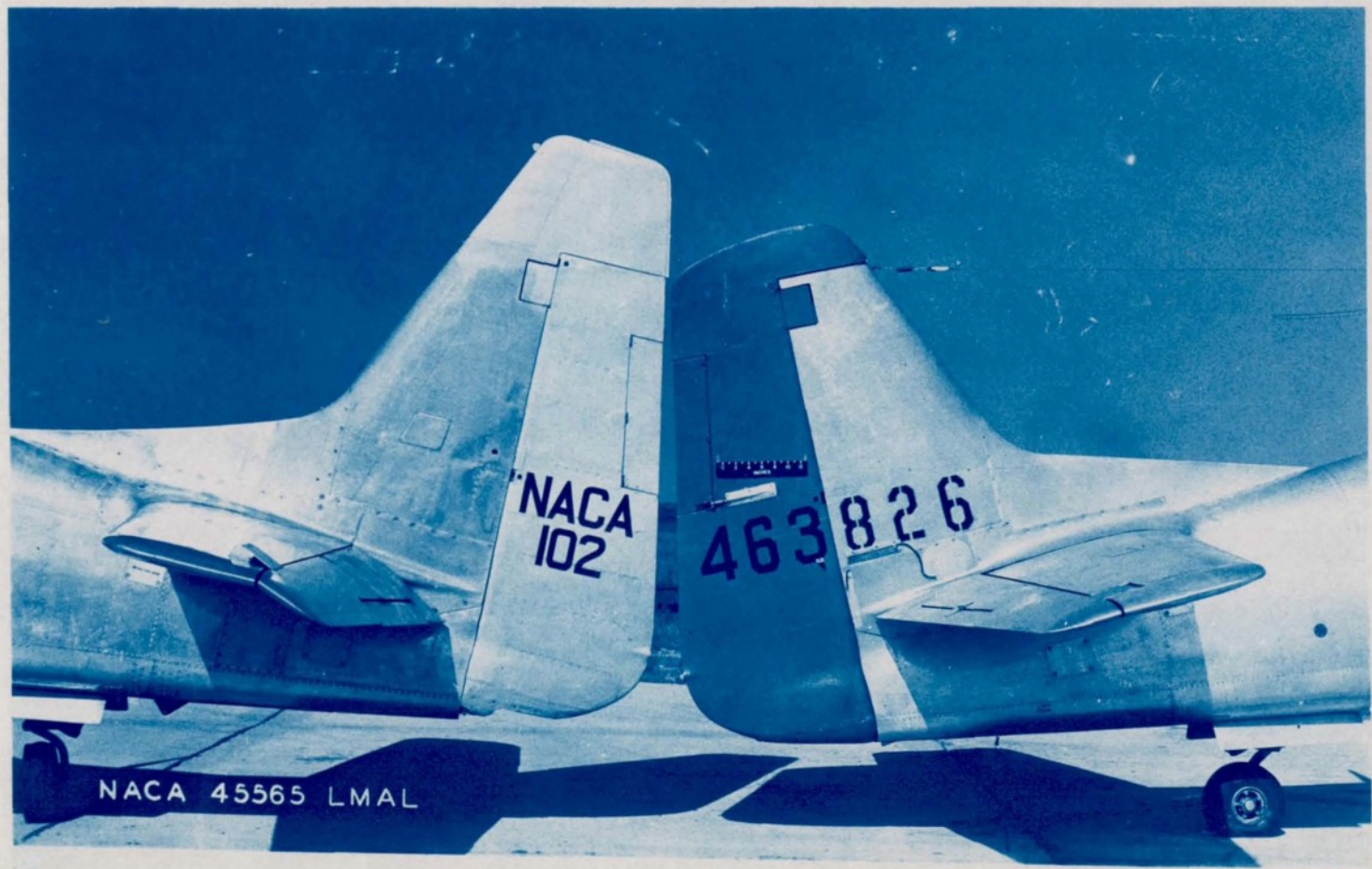
Figure 3.- Comparison of a P-51D-5-NA airplane with an extended tail and P-51D-20-NA (AAF No. 44-63826) with a horn balanced rudder.
