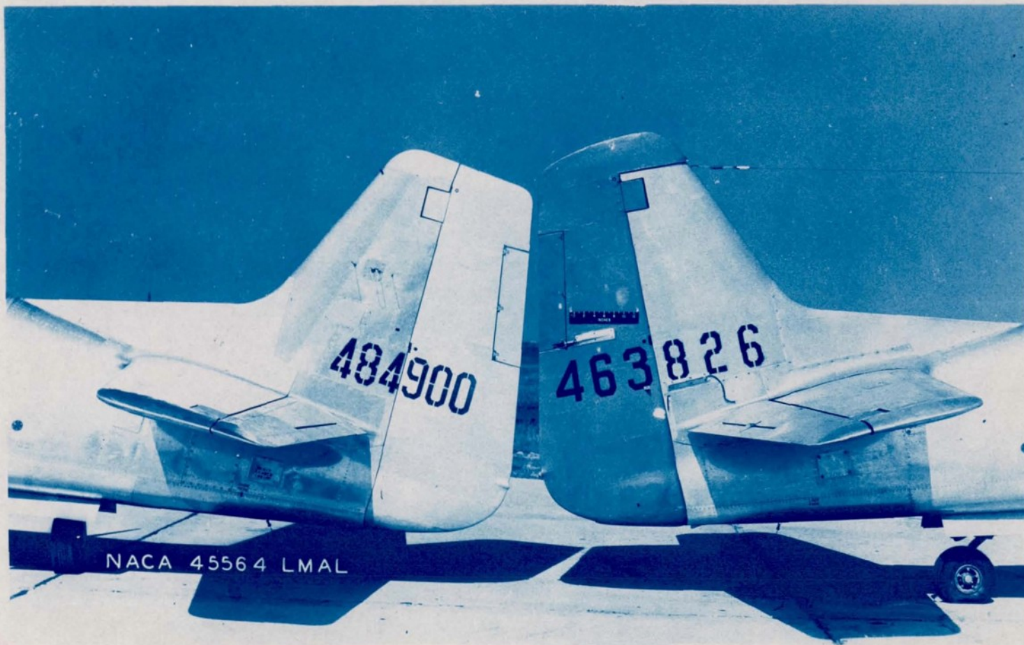
Figure 4.- Comparison of a P-51D-25-NT airplane with an original production configuration and the P-51D-20-NA (AAF No. 44-63826) with a horn balanced rudder.
