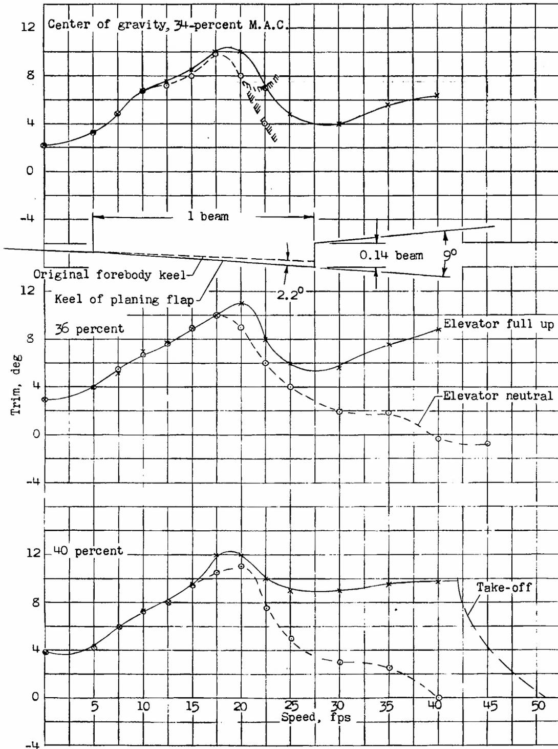
Figure 11.- Model 134PF-3. Variation of trim with speed. Step depth = 0.14 beam, stabilizer  $5^\circ$  up.  $C_{D0} = 0.87$ . Angle of planing flap =  $2.2^\circ$ ; chord = 1 beam.
