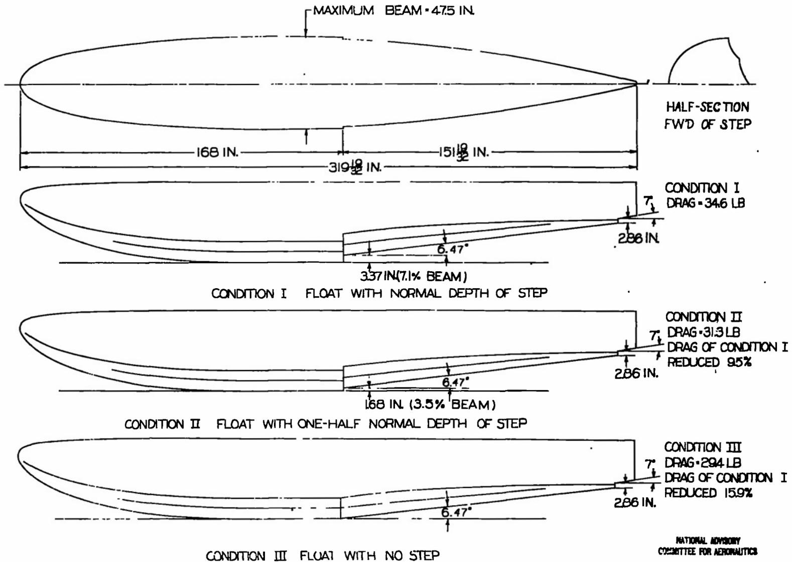
FIGURE 1.-MODIFICATIONS TO A FLOAT FOR THE PURPOSE OF SHOWING THE EFFECT OF THE DEPTH OF STEP ON AIR DRAG AT ZERO PITCH ( $V=100$  MPH;  $q=256$  LB/50 FT).
