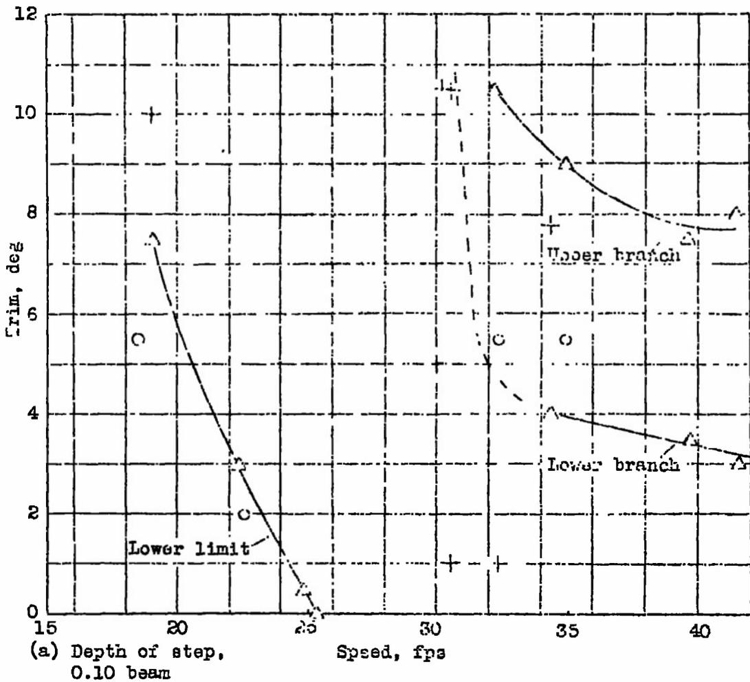
Figure 7 (a,b).- Model 134PF-2. Variation of trim limits with speed.
