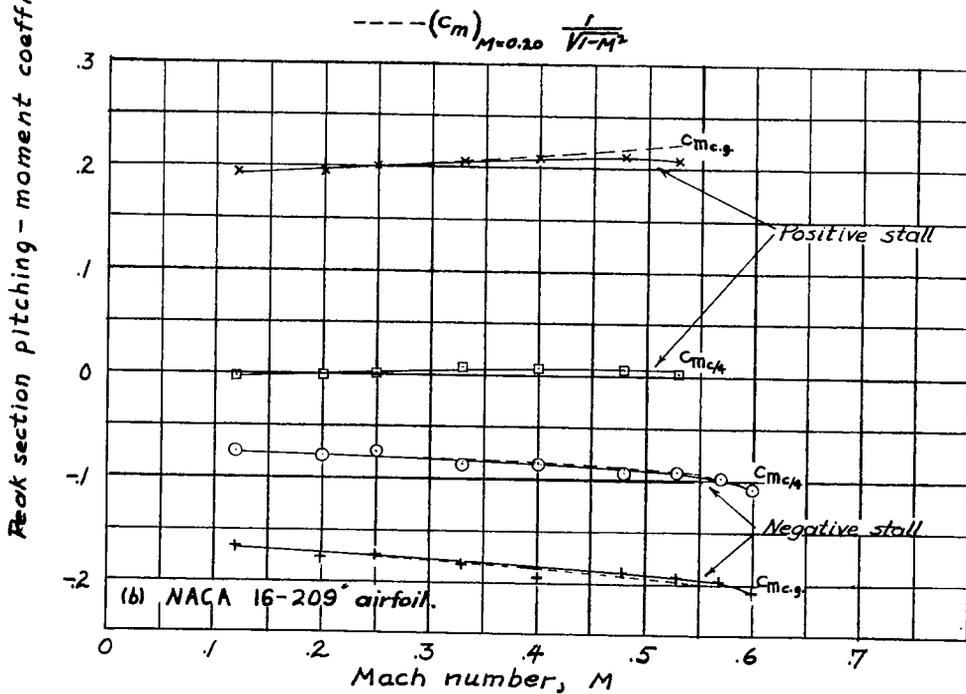
Figure 5.— Variation of peak positive and negative pitching-moment coefficients with Mach number for six 1-foot-chord NACA 16-series airfoils.
