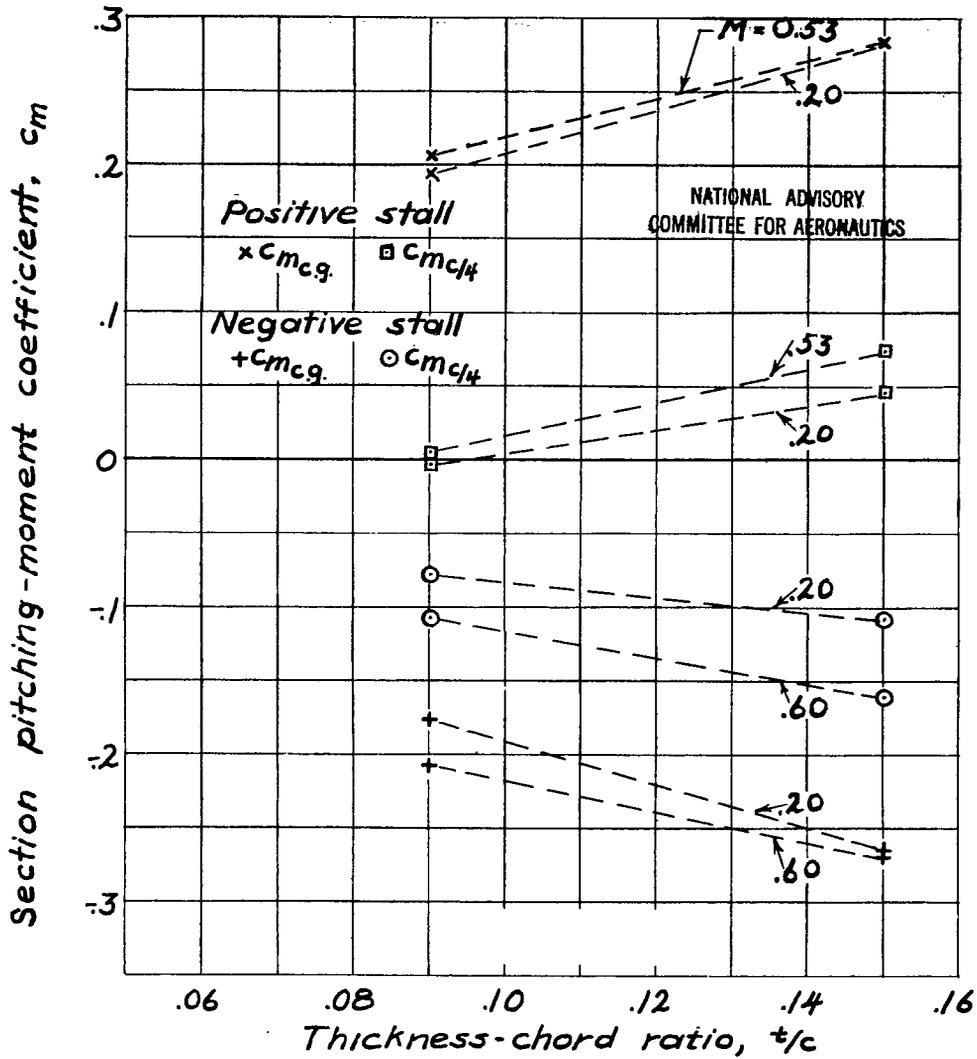
Figure 8.— Variation of peak positive and negative pitching-moment coefficients with thickness-chord ratio for NACA 16-series airfoils with camber designed to give  $c_l = 0.2$  at an angle of attack of  $0^\circ$ .
