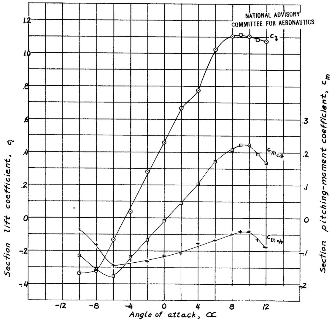
Figure 4.- Variation of section lift and pitching-moment coefficients with angle of attack for the NACA 16-509 airfoil at a Mach number of 0.33.
