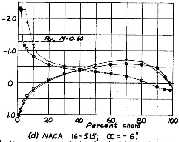
Figure 7. - Comparison of pressure distributions over 1-foot-chord NACA 16-509 and 16-515 airfoils at four negative angles of attack at  $M=0.25$  and  $M=0.60$ .
