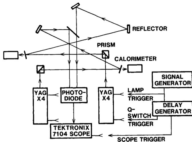
Figure 1. Simultaneity test of two quadrupled YAG lasers
