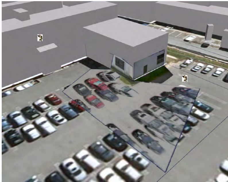
Fig. 10 A command-and-control (C2) application might show icons for forces and live sensor (including camera) data over a mixture of satellite imagery and virtual terrain.
