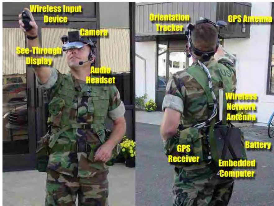
Fig. 2 We built this early prototype of our wearable AR system from commercial components. This and similar realizations were used in the research described later in this chapter.
