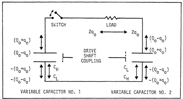
low capacitance C, and a low charge  $Q_1 = (Q_0 - q_0)$ . The switch is open; the switch, for the purpose of this exposition, shall be considered as and ideal switch (that is, it has negligible inductance, infinitely small capacitance relative to other circuit elements, infinite resistence when open, and zero resistence when closed). The potentials of the two variable capacitors are equal:
