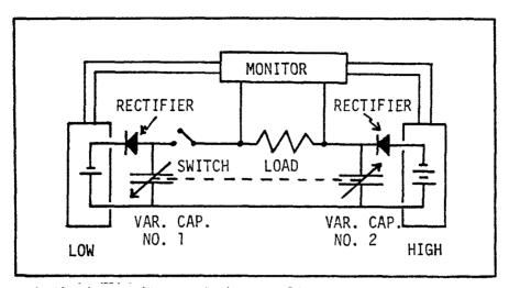
to power both the monitor and the supplies. A basic use of the low potential supply would be to replenish charge lost by leakage. With the low potential supply set at V, if Capacitor No. 1 low potential would attempt to fall below this L value because of charge leakage, then charge would be bled in from the supply through the rectifier to the capacitor to reestablish the correct operating value.
