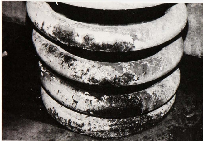
NORAD Spring, Showing Corrosion Effects
