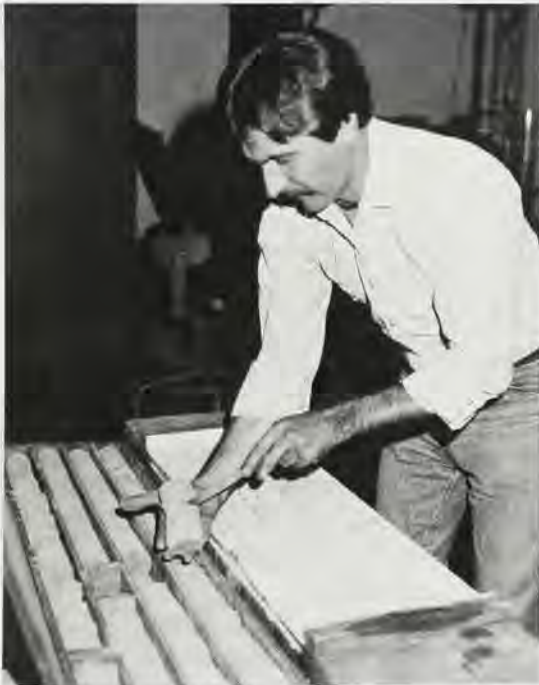
Larry Daniels in a District laboratory inspects the "core samples" extracted from the rock underlying the foundation of a District project.
