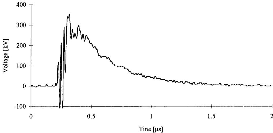
Figure 7. Output Voltage into 5 Ω from +/- 50 kV Charge of Four Stage Marx
