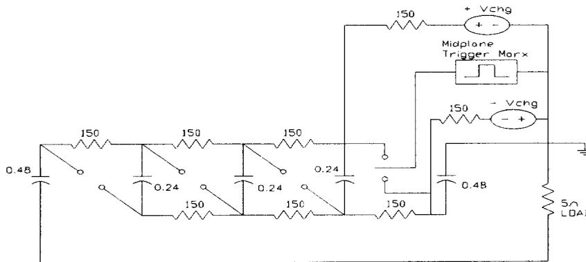
Figure 3 Circuit Diagram of Bipolar Four Stage Marx
