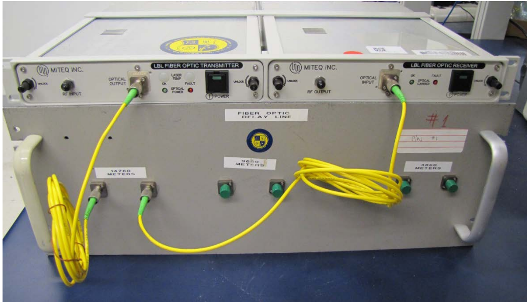
Figure 2 – Miteq FODL with three separate spools of delay lines: 4860 m, 9660 m, and 14,760 m (All incorporated in the lower unit).
