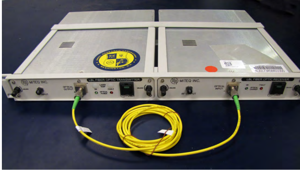
Figure 1 – Miteq fiber-optical delay line with 2-m length. (L) Transmitter unit. (R) Receiver unit.
