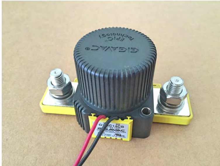
Figure 5.2: DC contactor used to provide software-based remote control of electrical power in the Chain Launcher prototype
