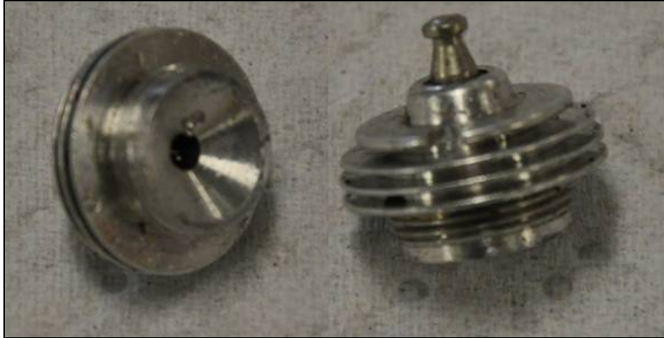
Figure 2–7: Photograph of a Cox 010 cylinder head incorporating the glow plug.
