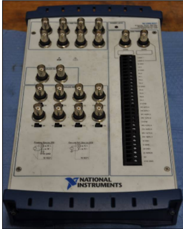
Figure 5–11: National Instruments USB–6221 BNC data acquisition module used to sample voltage signals from the cylinder pressure sensor.
