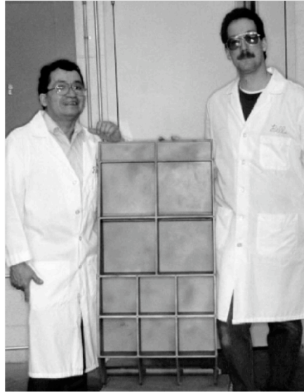
Figure 4: Proposed divergent flap prototype fabricated from cast TiAl (Ti-48Al-2Cr-2Nb) [7]
