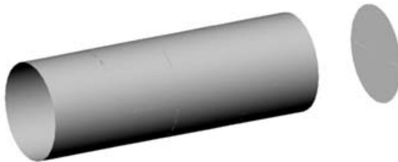
Figure A1 CAD model of the cylindrical cavity with a terminating plate at the back.
