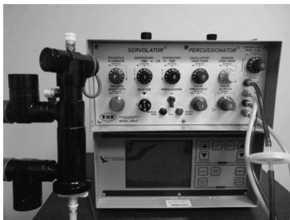
Figure 3. Photograph showing the volumetric diffusive respirator (VDR)-4 and flow amplifier (at left).
