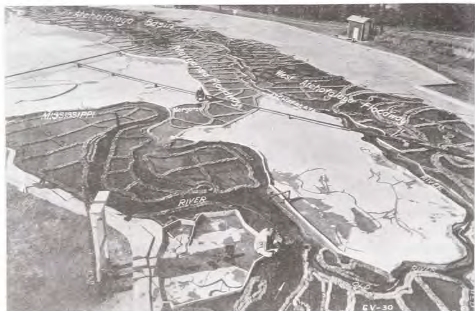
View of a portion of the Mississippi River Flood Control Model at the Waterways Experiment Station depicting the Morganza and West Atchafalaya Floodways in full operation. The large island is that portion of Pointe Coupee Parish that would have been inundated during the operation of the East Atchafalaya under the Jadwin Plan.
