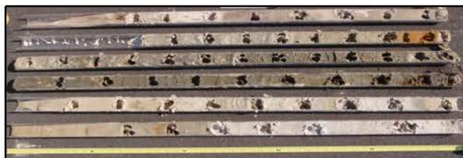
Example of high-resolution sub-sampling of soil cores for assessing attenuation in low-k zones
