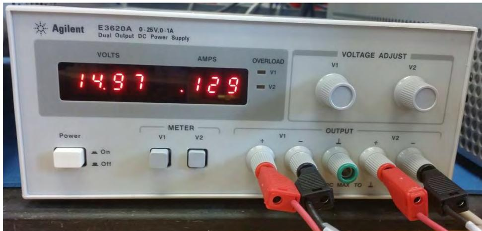
Figure 16 AT-E3620A Laboratory DC power supply, 0-25 V, 0-1A
