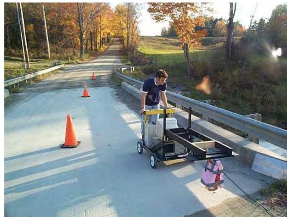
Figure 13 Use of linear vector network analyzer for penetrating radar scan of Turkey Lane Bridge deck (Hinesburg, VT, circa 2003)
