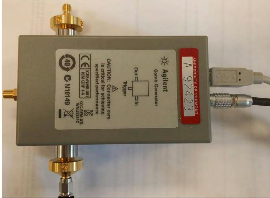
Figure 15 Agilent N10149 26.5 GHz Comb Generator
