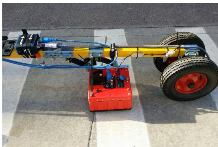
**Figure 45 Dual-band GPR during Fleming Museum sidewalk scan**
