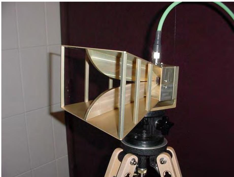
**Figure 20 A.H. Systems Double Ridge Guide Horn Antenna SAS-571 700 MHz - 18 GHz**
