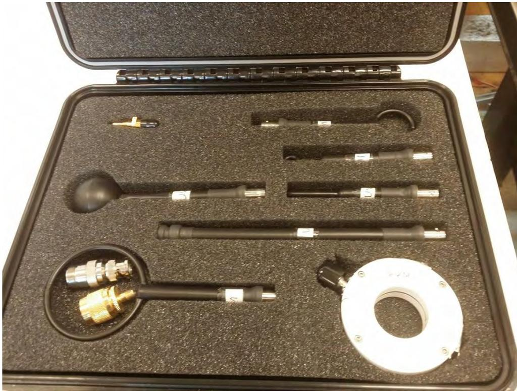
**Figure 19 Electro-Metrics EM-6992 Electromagnetic Probe Set**
