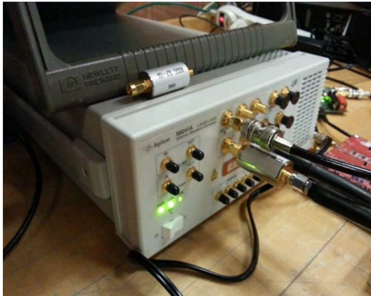
Figure 21 AT-N8241A 15 bit 1.25 GHz Arbitrary Waveform Generator with LXI Module
