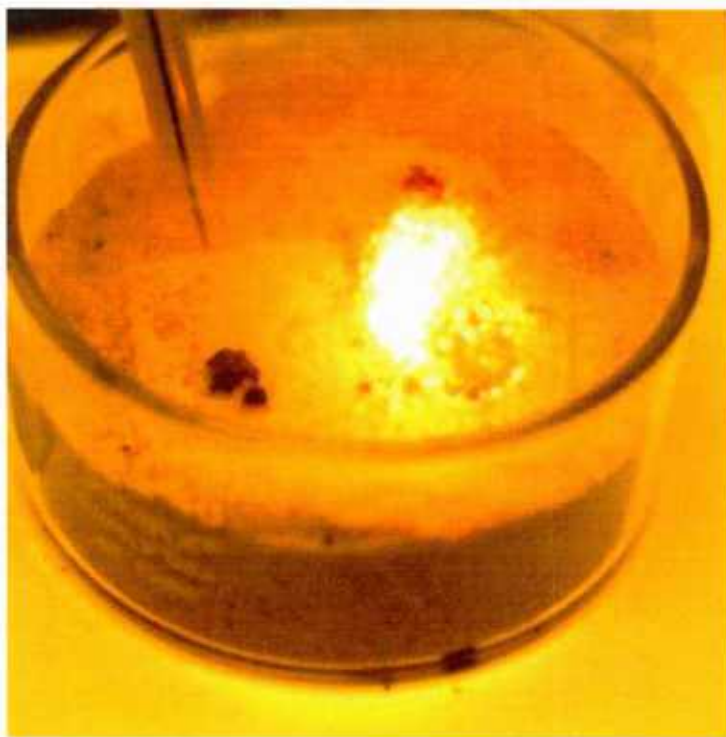
Figure 10.1 Ignition of HEHN on catalyst (preheated to 105°C) 782ms after the drop contacted the catalyst.
