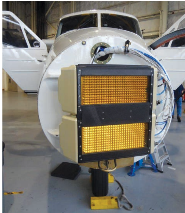
The Airborne Sense and Avoid Radar Panel is seen during installation on a Twin Otter aircraft.
