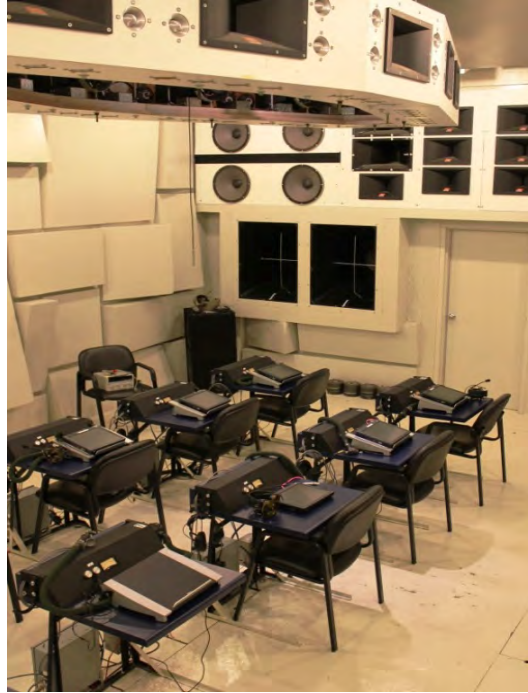
Figure 10. AFRL's VOCRES facility used to measure speech intelligibility performance
