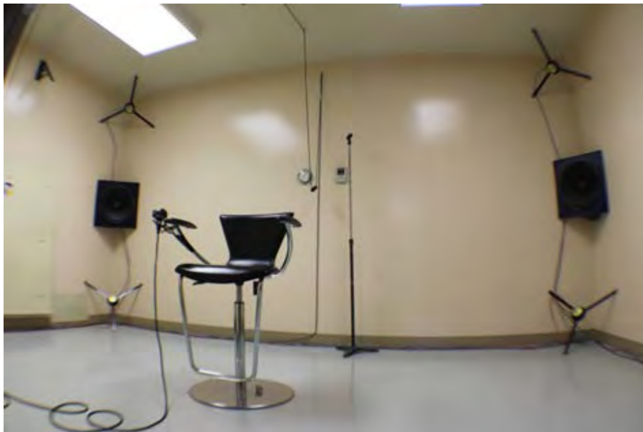
Figure 3. Facility used for measurement of passive continuous noise attenuation
