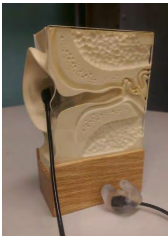
Figure 2. ACCES (custom silicone earpieces with communication cabling)
