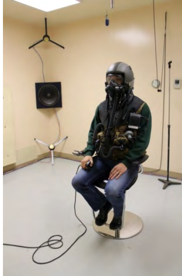
Figure 4. Subject completing the threshold measurement in the HGU-55/P and the modified A/P22P-14A (V)3 configuration
