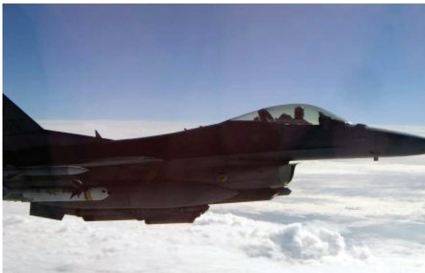
A U.S. Air Force F-16CJ from the 20th Fighter Wing on a leaflet-dropping mission over Libya on July 13, 2011. Under its right wing is a PDU-5/B leaflet dispenser.
