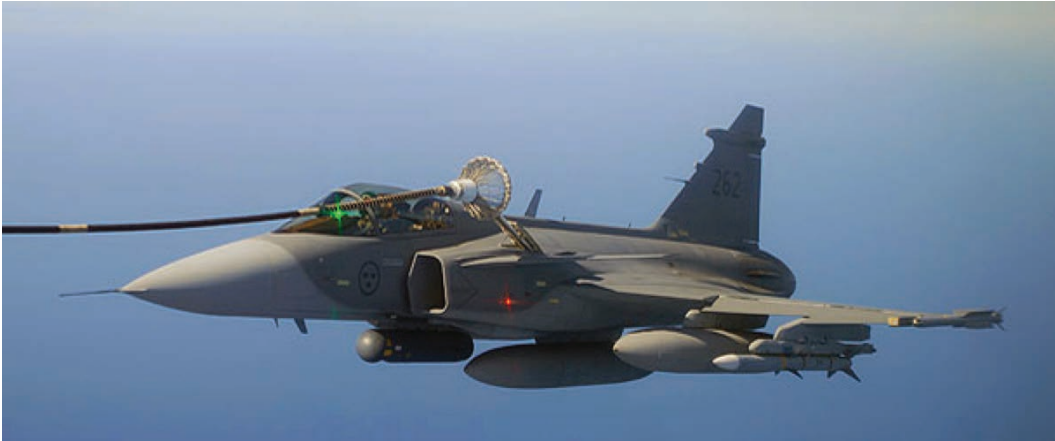
Swedish Air Force JAS 39C Gripen refueling from Tp 84 (C-130H) Hercules over the Mediterranean, April 8, 2011. Aircraft is carrying IRIS-T and AMRAAM air-to-air missiles and a Rafael RecceLite pod. Courtesy of the Swedish Armed Forces.
