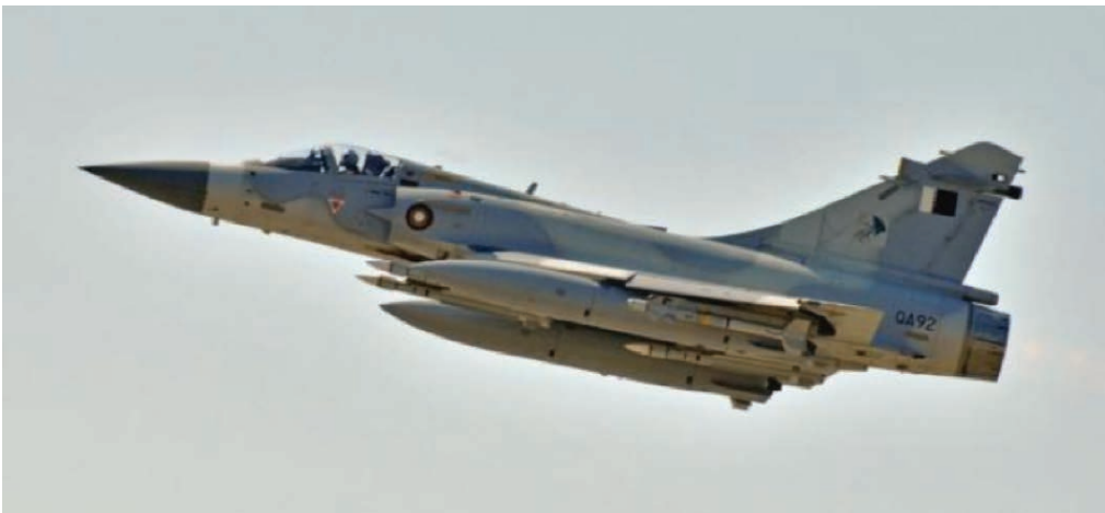
QEAF Mirage 2000-5 configured with MICA and Magic missiles.
