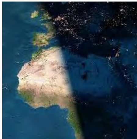
Figure 9. Areas near the day/night terminator may require additional processing to estimate and remove straylight effects.
