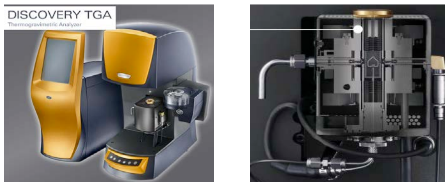
Figure 1.2.1: The Discovery Series TGA System (left). Cutaway diagram of the Discovery Series TGA IR furnace (right). The water cooled jacket, furnace interior and horizontal gas delivery system are shown. (3)
