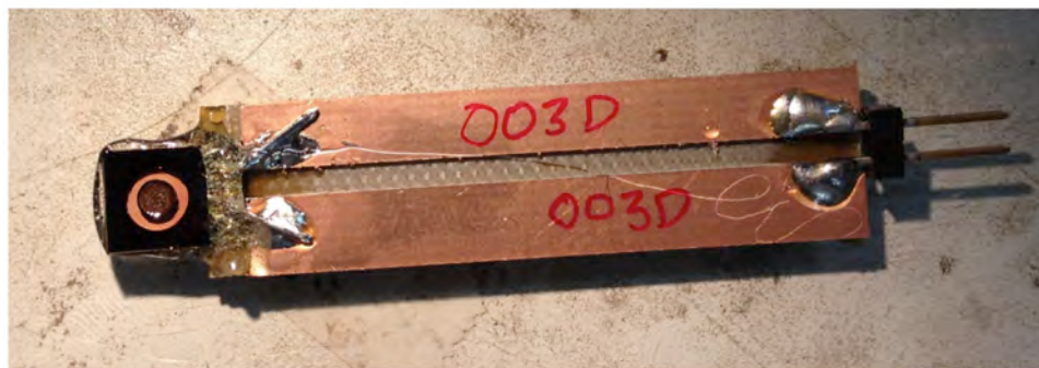
Figure 1: The \mu ZNMF actuator: (a) schematic of the actuator, (b) actuator coil die with a laser-cut orifice in the center and a double sided tape spacer at the periphery, (c) top view of the actuator assembled by placing the magnet die on the coil die, (d) actuator's bottom view from the side of the coil die, and (e) the position of the actuator on its test circuit board.
