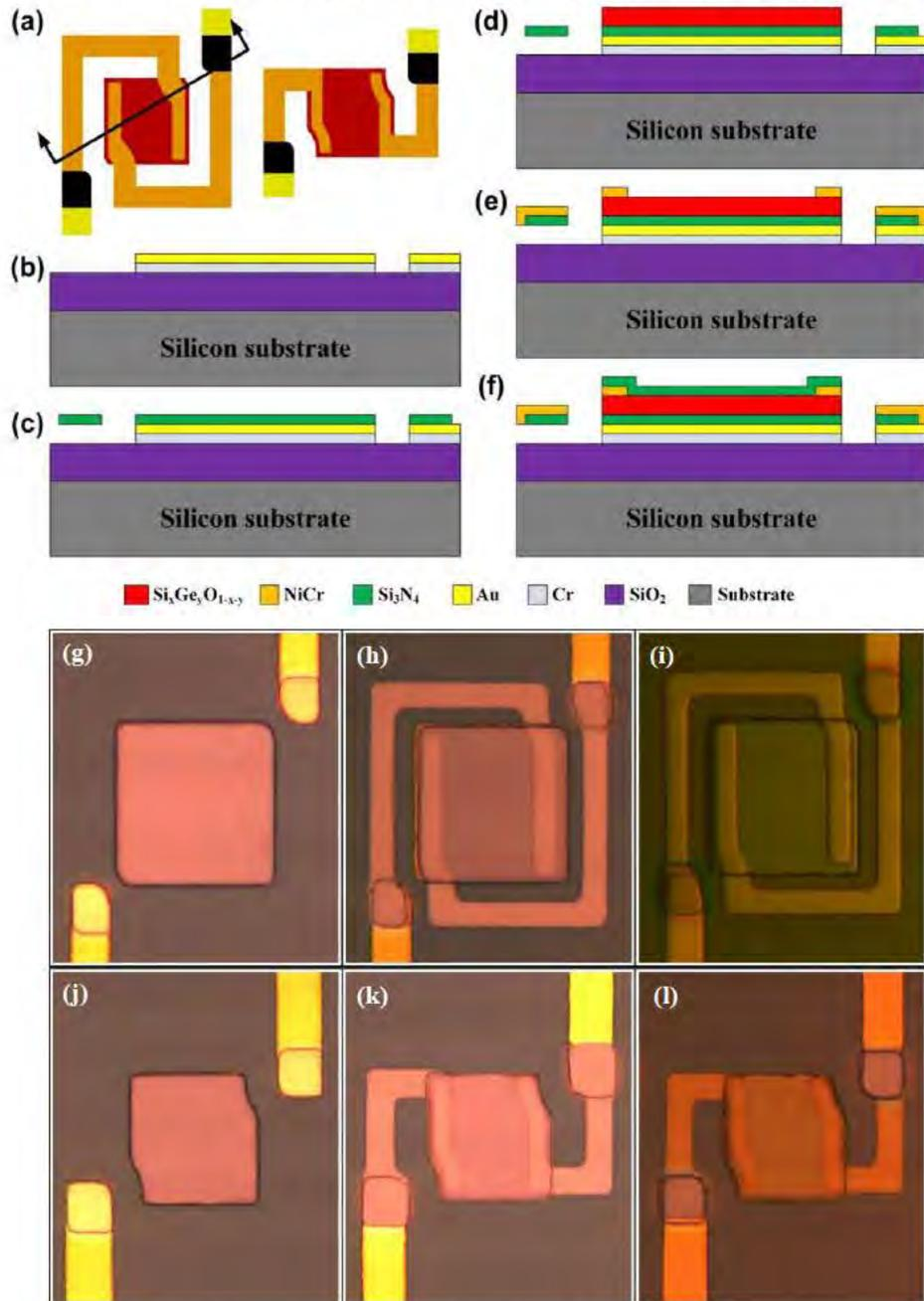
**Figure 18:** Microbolometer fabrication steps: (a) Top view of pixels of two designs with different supporting arm structure; (b) Cross sectional view of different steps of fabrication. Optical images of the microbolometer with a pixel area of  $40 \times 40 \mu\text{m}^2$  at the end of different steps of fabrication, (g) Si-Ge-O layer, (h) Ni-Cr layer, (i) final device for L-shaped anchor; (j) Si-Ge-O layer, (k) Ni-Cr layer, (l) final device for I-shaped anchor
