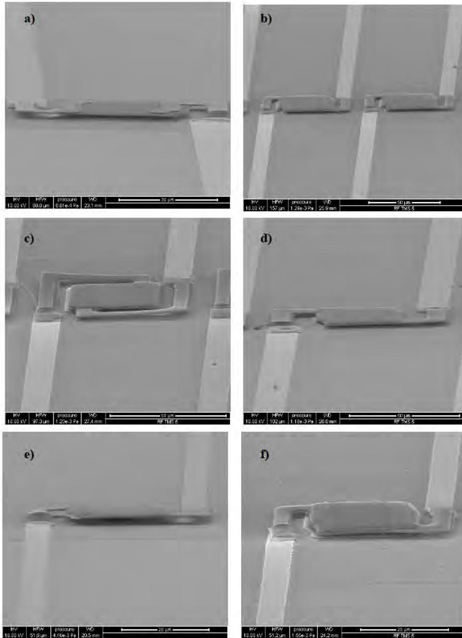
**Figure 17:** SEM micrographs of the microbolometer after removing the polyimide sacrificial layer with a pixel area of a-d)  $40 \times 40 \mu\text{m}^2$ , e, f)  $25 \times 25 \mu\text{m}^2$ .
