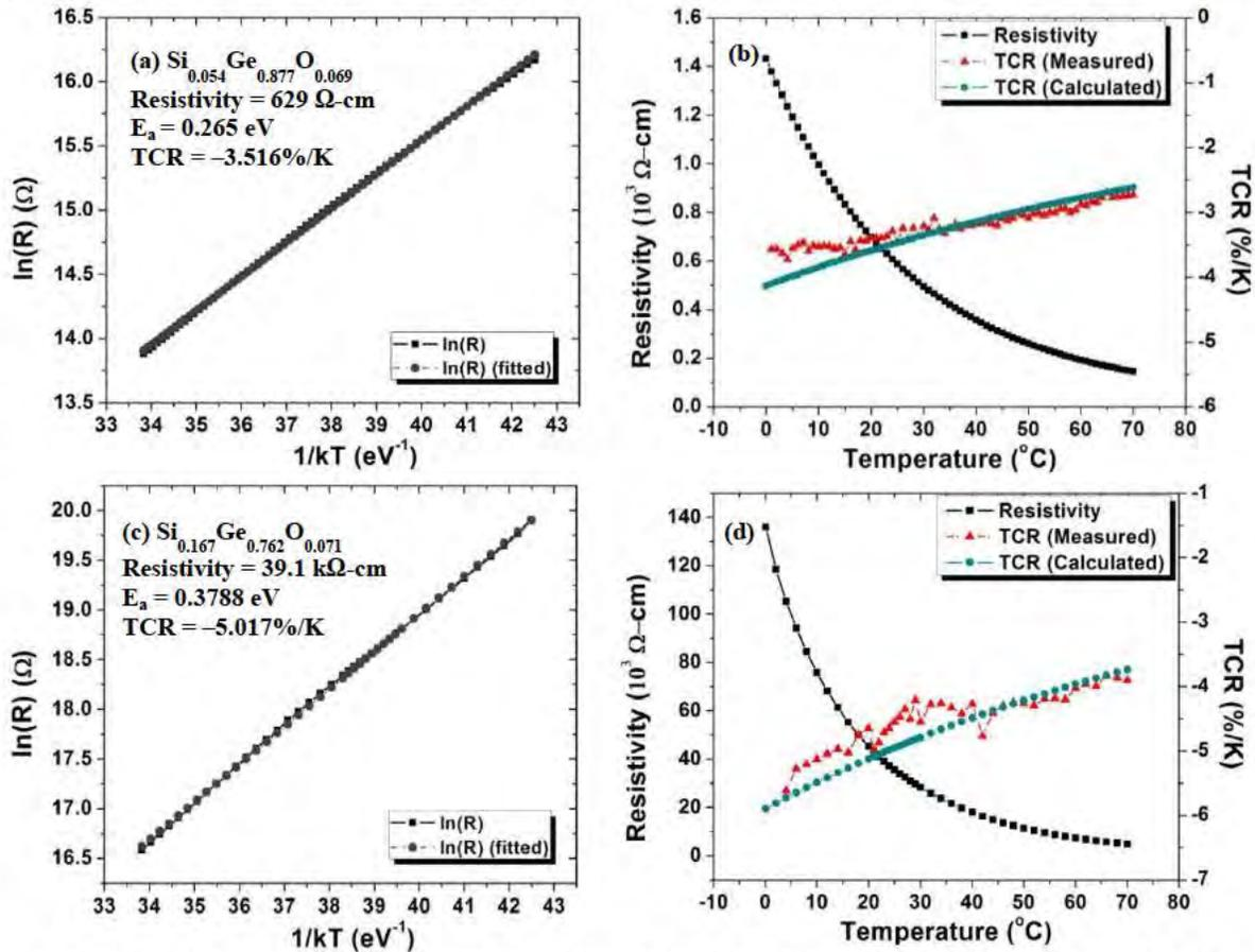
**Figure 3:** Arrhenius plot of resistance versus  $1/kT$ , and TCR and resistivity versus temperature of (a, b)  $\text{Si}_{0.054}\text{Ge}_{0.877}\text{O}_{0.069}$ , (c, d)  $\text{Si}_{0.167}\text{Ge}_{0.762}\text{O}_{0.071}$  films deposited at room temperature.
