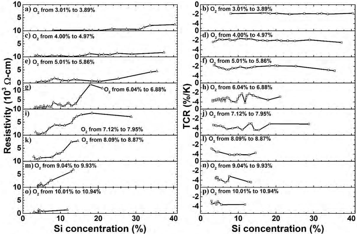
**Figure 6:** Resistivity and TCR as a function of Si concentration for a fixed  $O_2$  (a-b) 3.01-3.89%, (c-d) 4.00-4.97%, (e-f) 5.01-5.86%, (g-h) 6.04-6.88%, (i-j) 7.12-7.95%, (k-l) 8.09-8.87%, (m-n) 9.04-9.93%, (o-p) 10.01-10.94%
