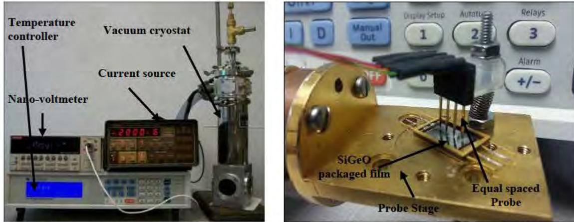
**Figure 2:** Experimental set up for the measurement of resistance vs. temperature characteristics. An image of a) the whole setup, b)  $\text{Si}_x\text{Ge}_y\text{O}_{1-x-y}$  packaged sample mounted on the base stage of equally spaced 4-probe sample holder inside a closed-cycle cryostat.
