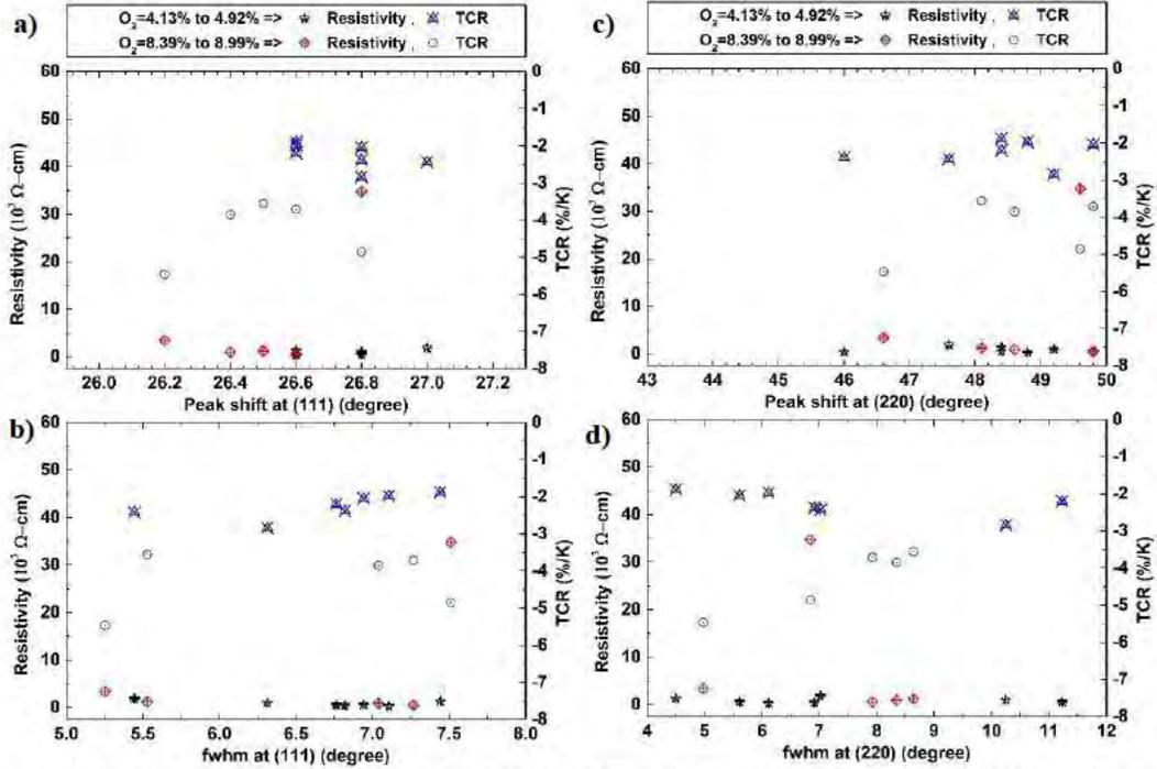
**Figure 10:** Resistivity and TCR vs Peak shift of films for fixed O<sub>2</sub> (a) peak at (111) (c) peak at (200); Resistivity and TCR vs fwhm of films for fixed O<sub>2</sub> (a) peak at (111) (c) peak at (200)
