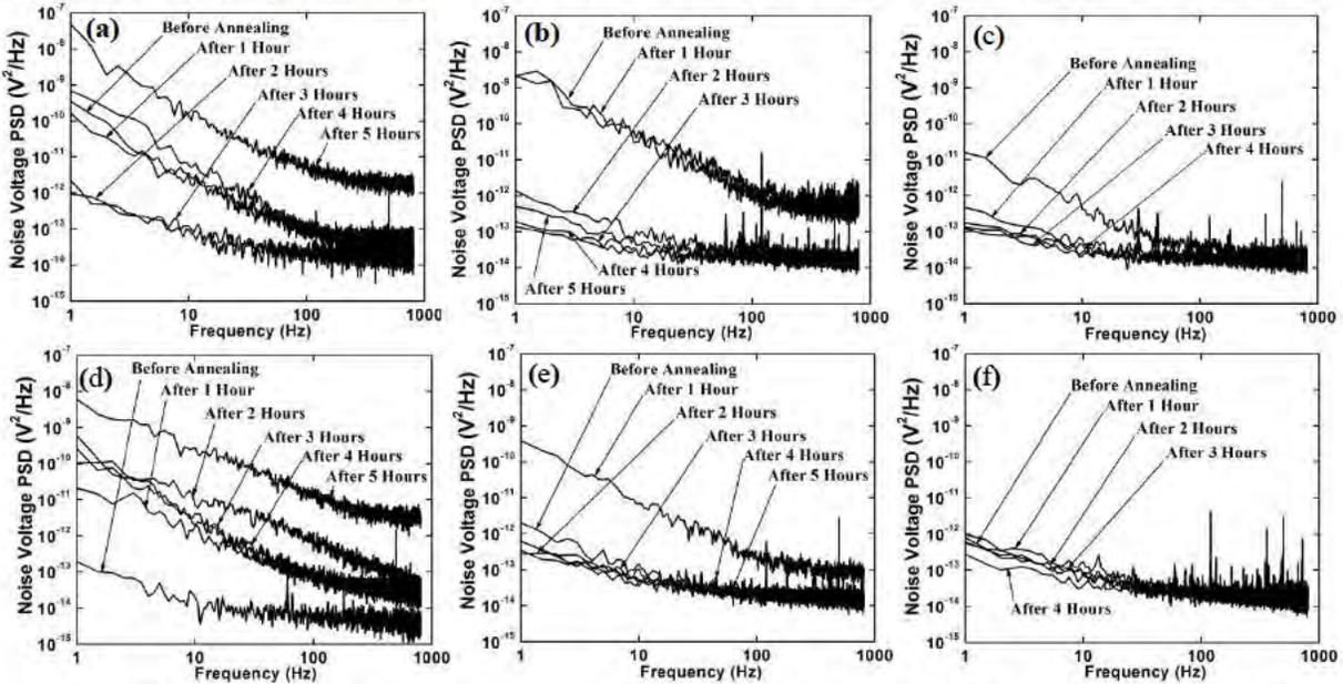
**Figure 24:** Noise PSD before and after annealing for different durations: in W04, devices a) W04D43, b) W04D11 and c) W04D33 annealed at 200 °C, 250 °C and 300 °C respectively; in W01, devices d) W01D21, e) W01D22, f) W01D52 annealed at 200 °C, 250 °C and 300 °C respectively
