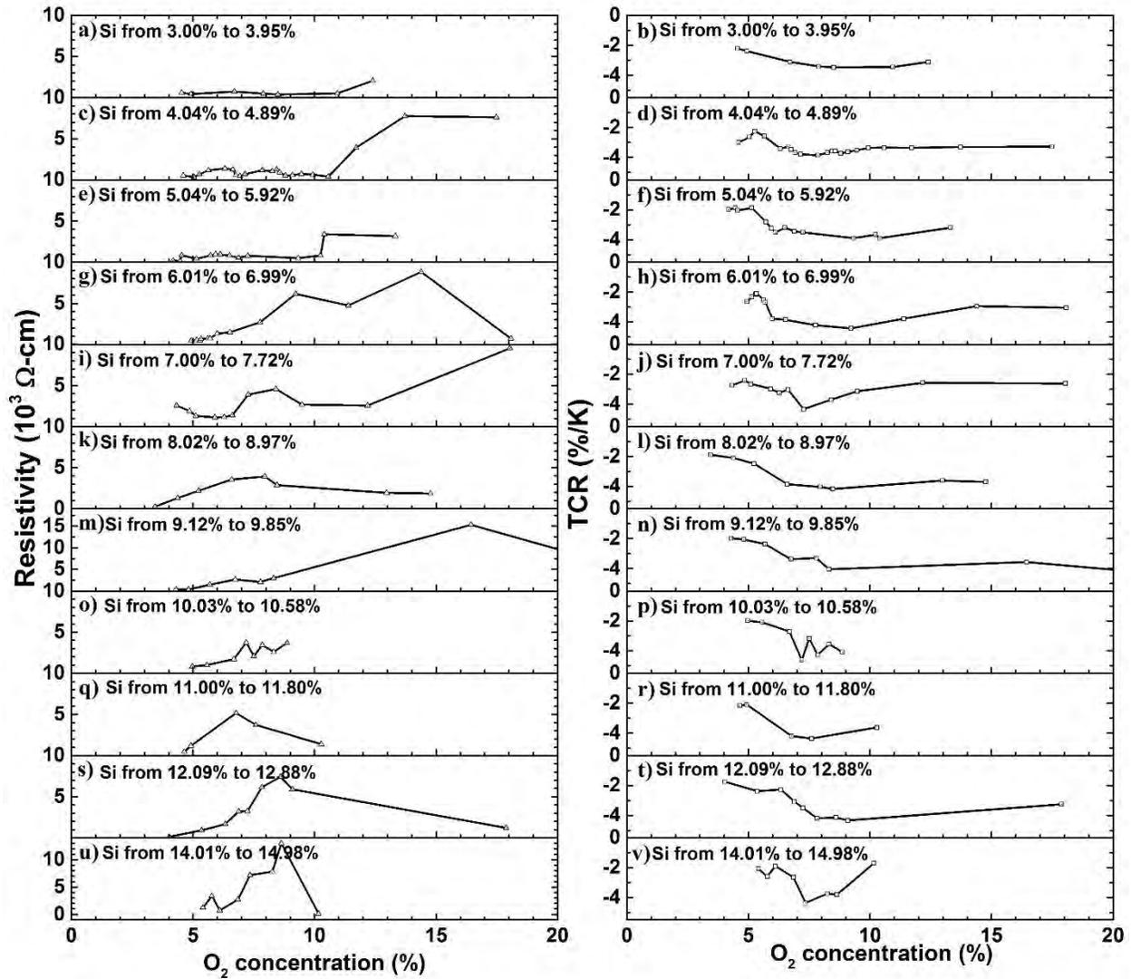
**Figure 7:** TCR and Resistivity as a function of  $\text{O}_2$  concentration for fixed Si of (a-b) 3% to 3.95%, (c-d) 4.00% to 4.89%, (e-f) 5.04% to 5.92%, (g-h) 6.01% to 6.99%, (i-j) 7.00% to 7.72%, (k-l) 8.02% to 8.97%, (m-n) 9.12% to 9.85%, (o-p) 10.03% to 10.58%, (q-r) 11% to 11.8%, (s-t) 12.09% to 12.88% and (u-v) 14.01% to 14.98%.
