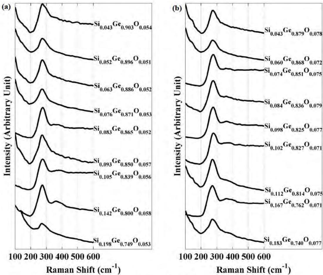
Figure 12: Raman spectra of  $\text{Si}_x\text{Ge}_y\text{O}_{1-x-y}$  films with oxygen content of (a) 5%, (b) 7%
