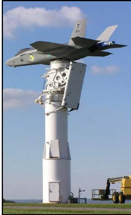
Figure 9. Aircraft Positioner with a Full-Scale Model of an F-35
